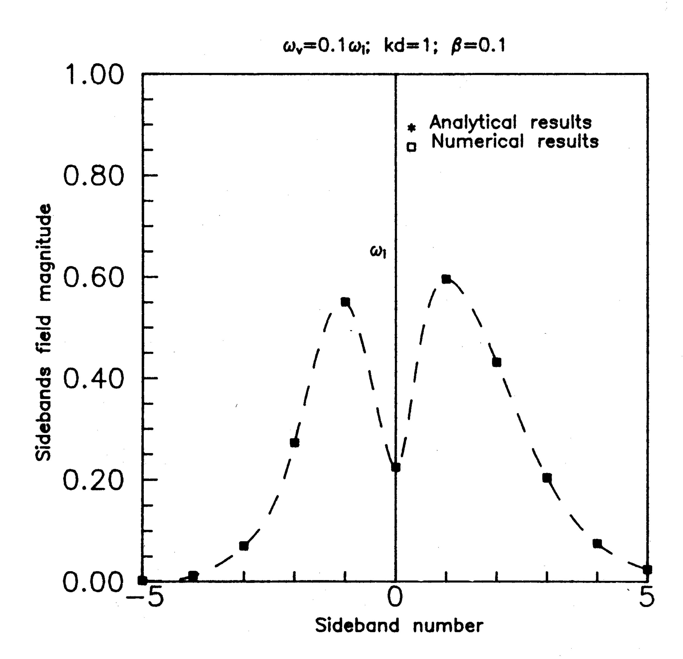
Fig. 2. Major sidebands of the reflected field spectrum as obtained both numerically and analytically.
