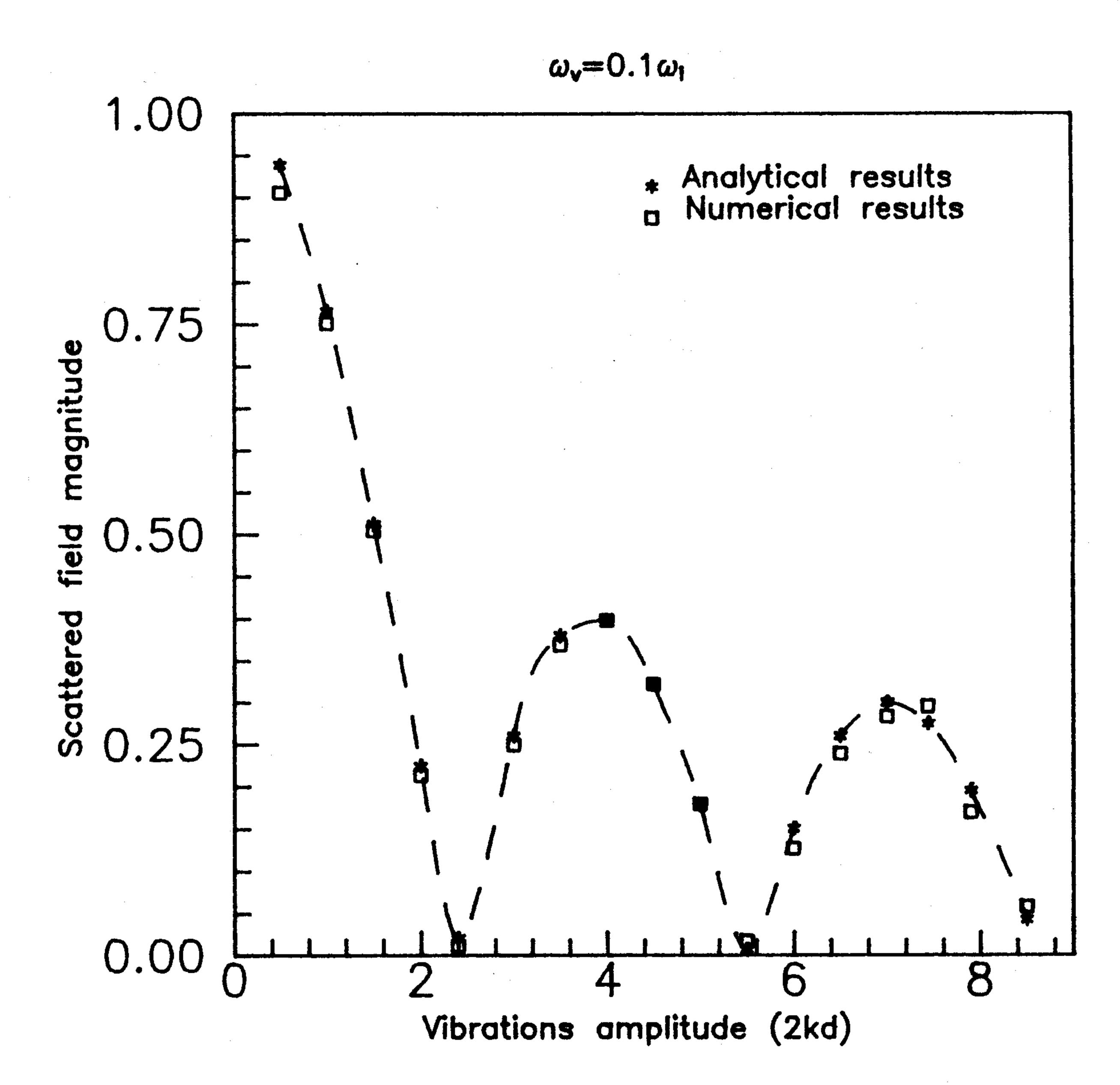
Fig. 3. Variations of the scattered field amplitude at the illumination frequency for different vibrations amplitude (d) of the mirror.
