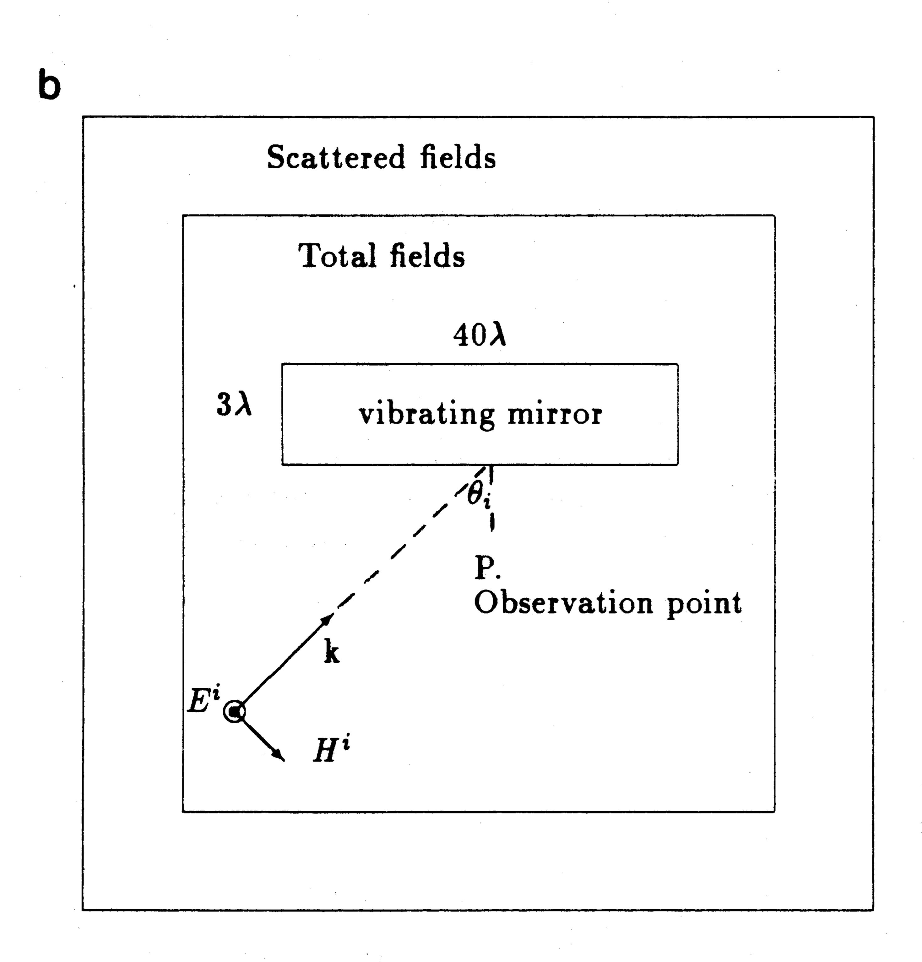
Fig. 1. (a) Snapshot of a Moving Mirror in a 1D FD-TD Grid. (b) Vibrating Mirror in a 2D FT-TD Grid.
