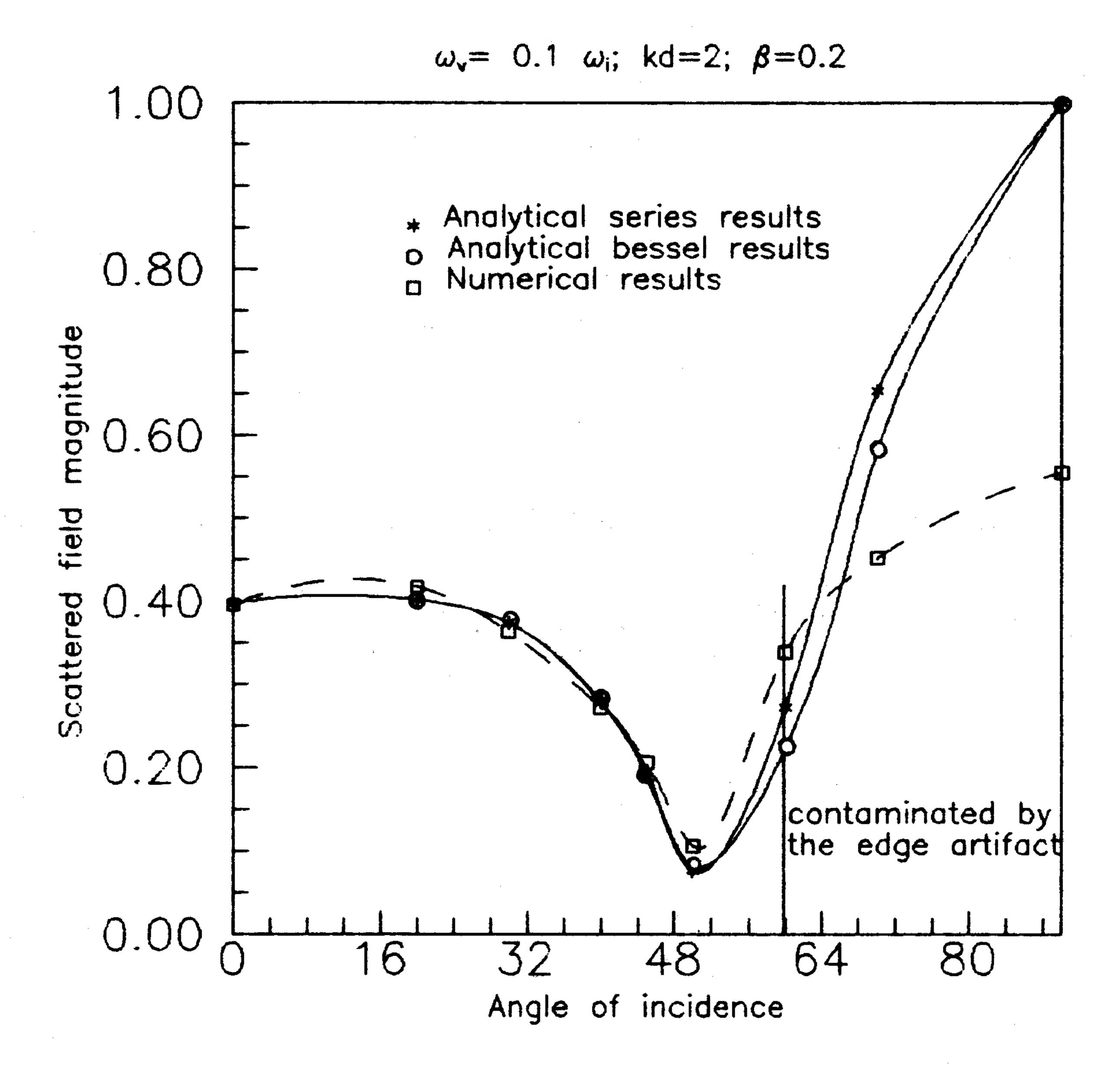
Fig. 8. Variations of the scattered field amplitude at the illumination frequency  $\omega_i$  for different angles of incidence  $\theta_i$ .
