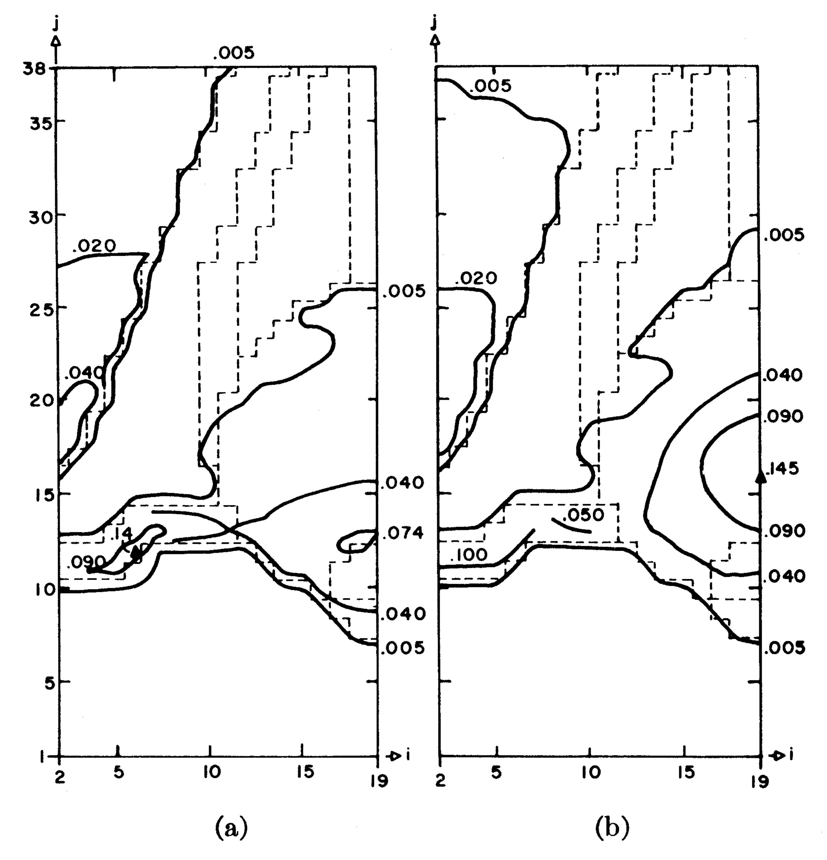
Fig. 5. Maps of the computed, normalized heating potential  $Q_n$  at lattice symmetry plane  $z = 19\delta$ . (a) Incident frequency = 750 MHz. (b) Incident frequency = 1.5 GHz.
