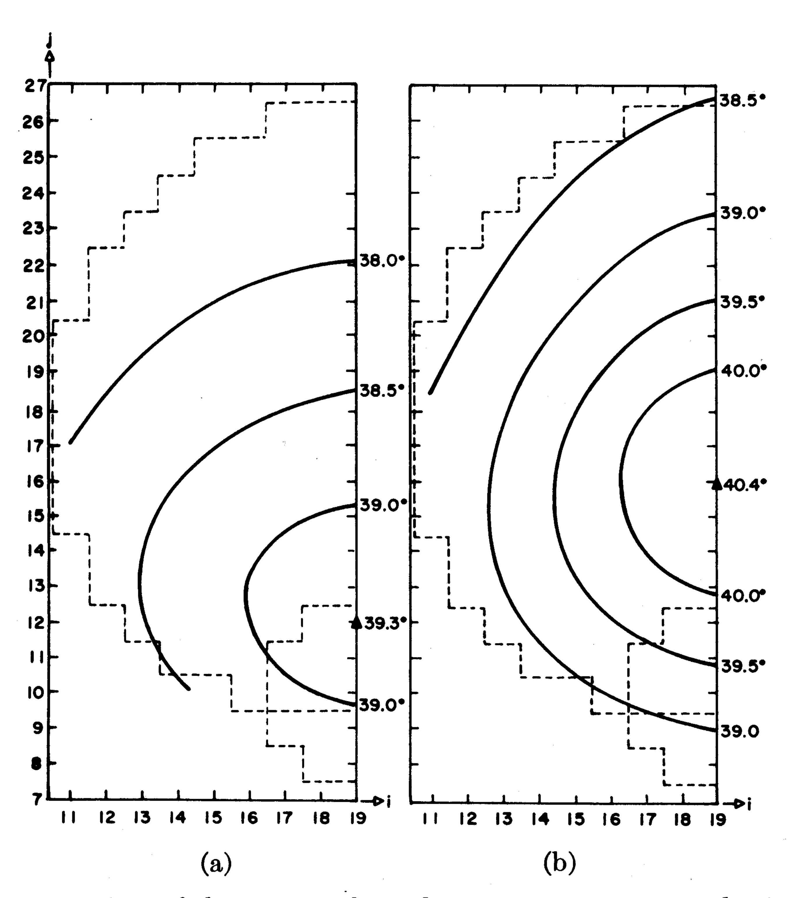
Fig. 7. Maps of the computed steady-state temperatures at lattice symmetry plane  $z=19\delta$  for  $P_{\rm inc}=100$  mW/cm<sup>2</sup> and h=50 W/m<sup>2</sup>·°C. (a) Incident frequency = 750 MHz. (b) Incident frequency = 1.5 GHz.
