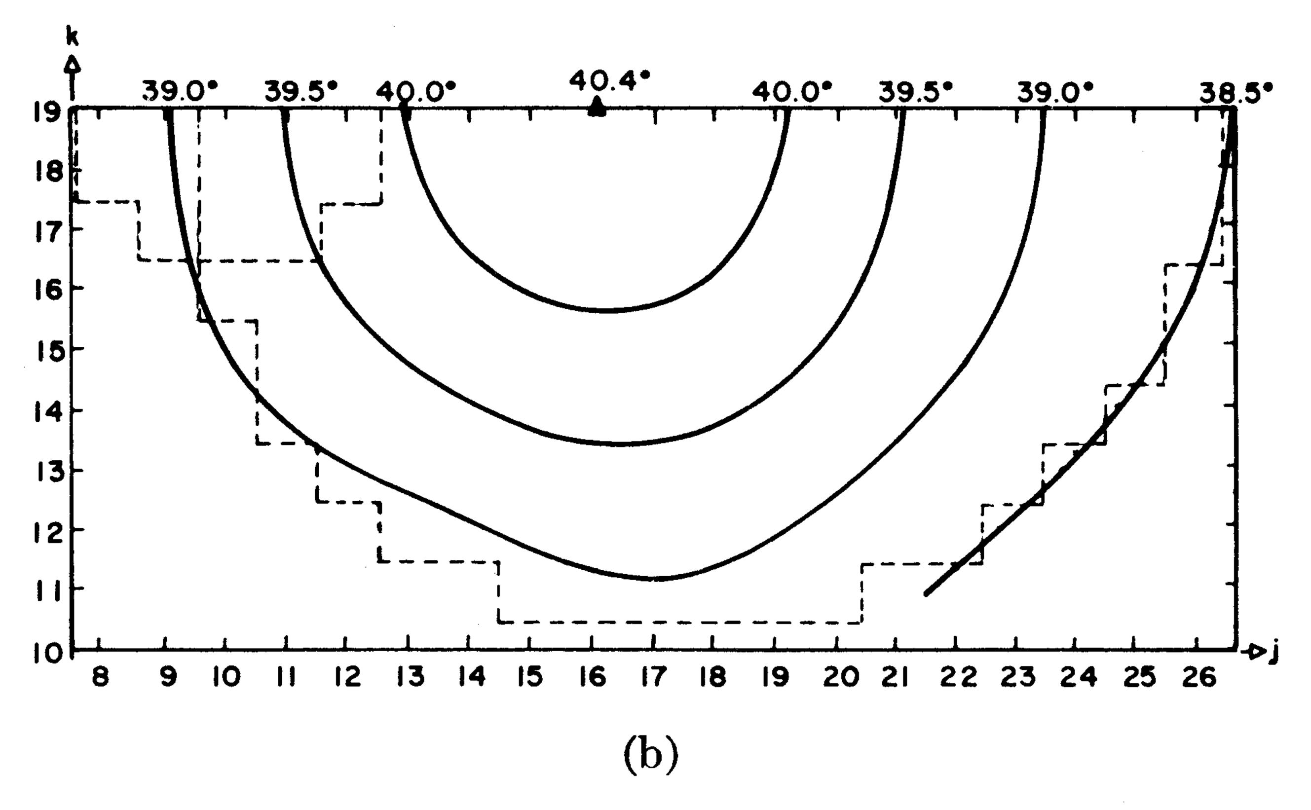
Fig. 8. Maps of the computed steady-state temperatures at lattice symmetry plane  $x = 19\frac{1}{2}\delta$  for  $P_{\text{inc}} = 100 \text{ mW/cm}^2$  and  $h = 50 \text{ W/m}^2 \cdot ^{\circ}\text{C}$ . (a) Incident frequency = 750 MHz. (b) Incident frequency = 1.5 GHz.
