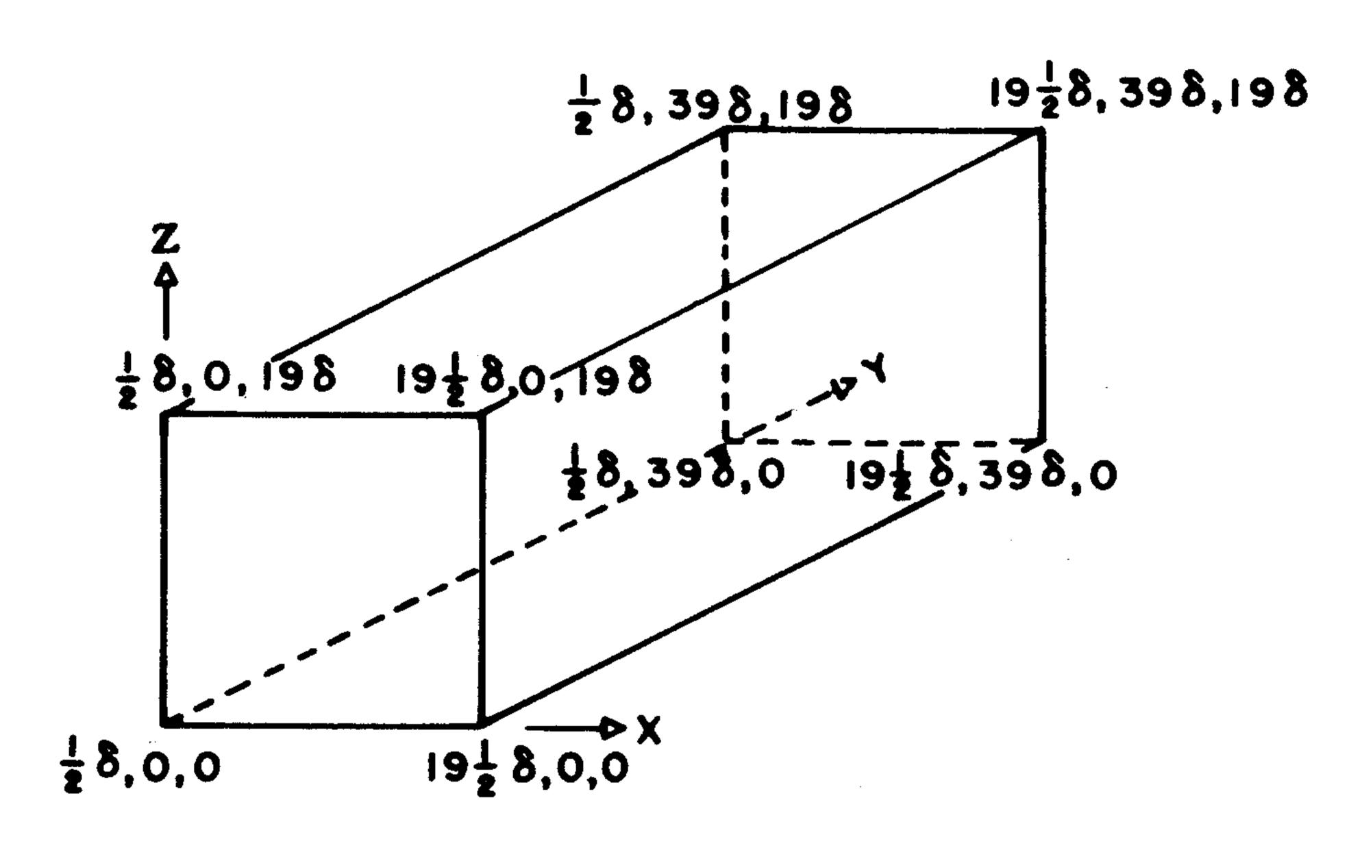
Boundary planes of the finite-difference lattice used for the microwave scattering problem.
