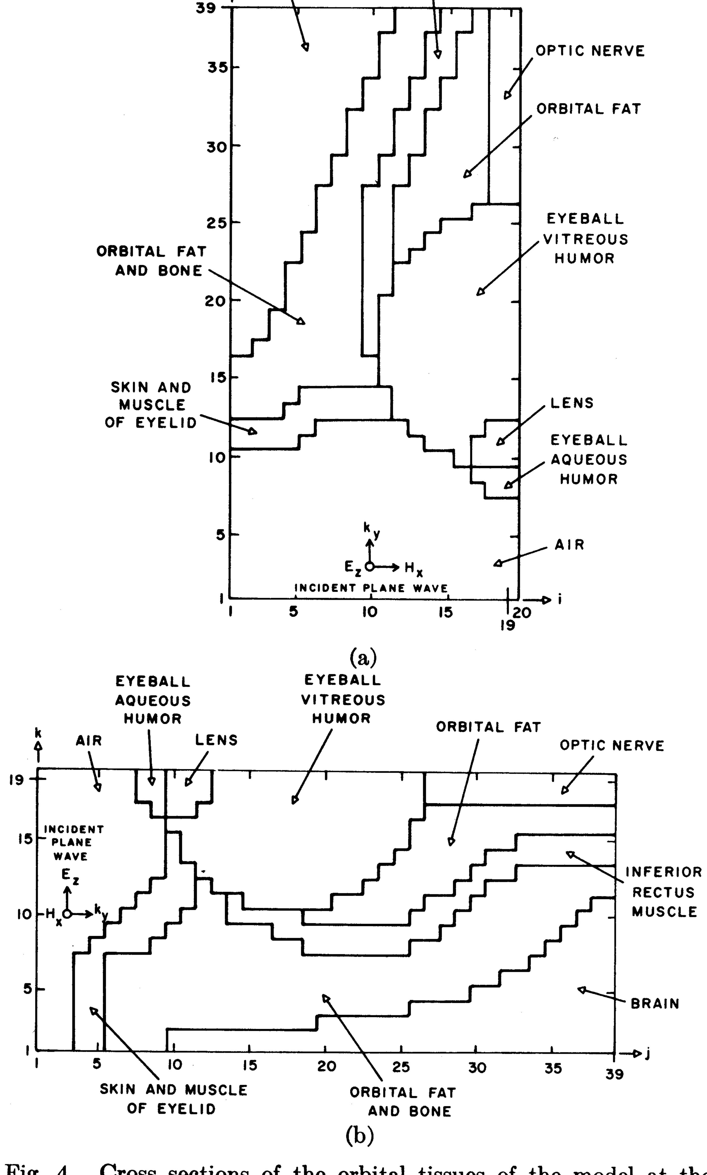
Fig. 4. Cross sections of the orbital tissues of the model at the lattice symmetry planes. (a) Plane  $z = 19\delta$ . (b) Plane  $x = 19\frac{1}{2}\delta$ .
