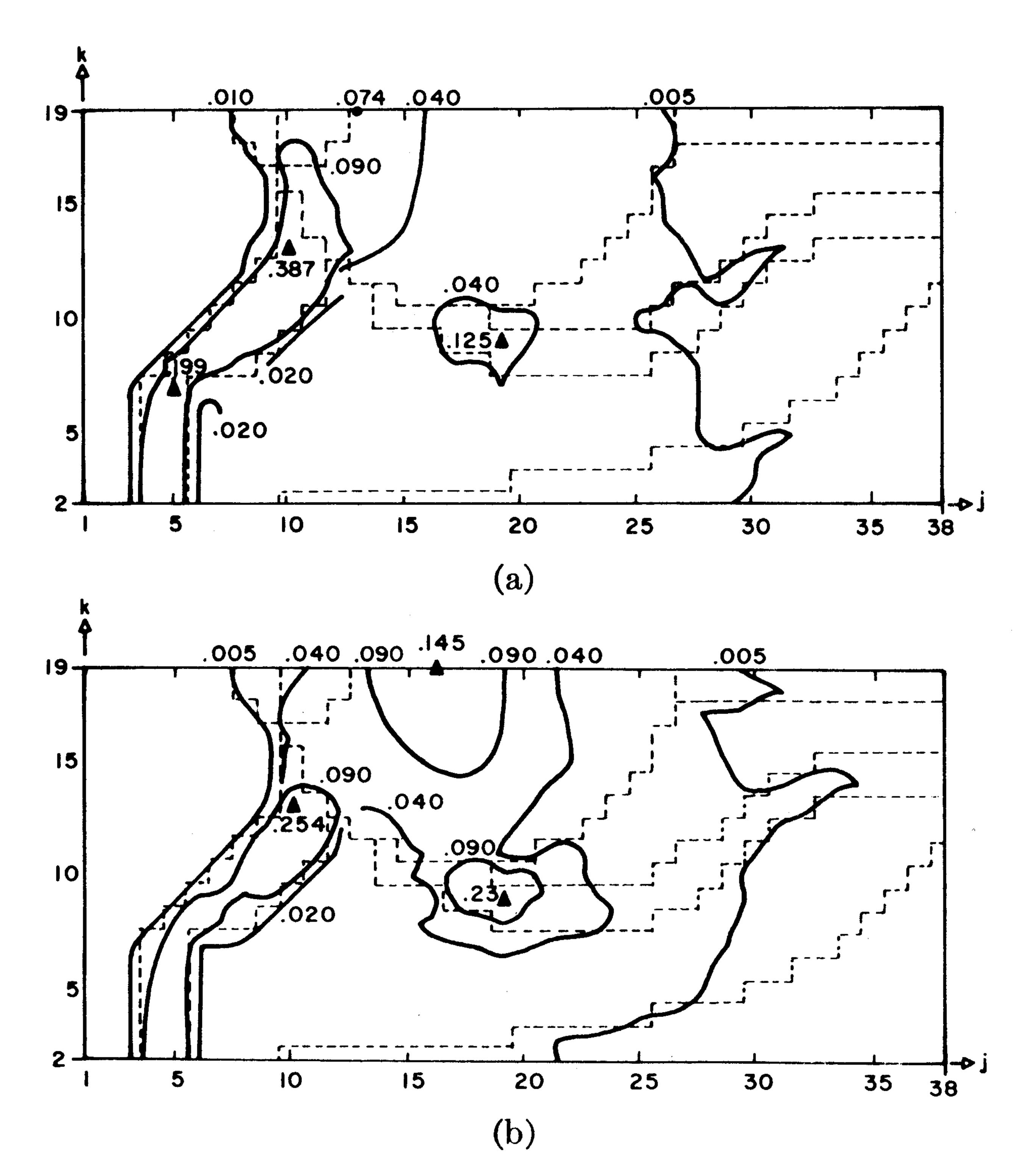
Fig. 6. Maps of the computed, normalized heating potential  $Q_n$  at lattice symmetry plane  $x = 19\frac{1}{2}\delta$ . (a) Incident frequency = 750 MHz. (b) Incident frequency = 1.5 GHz.
