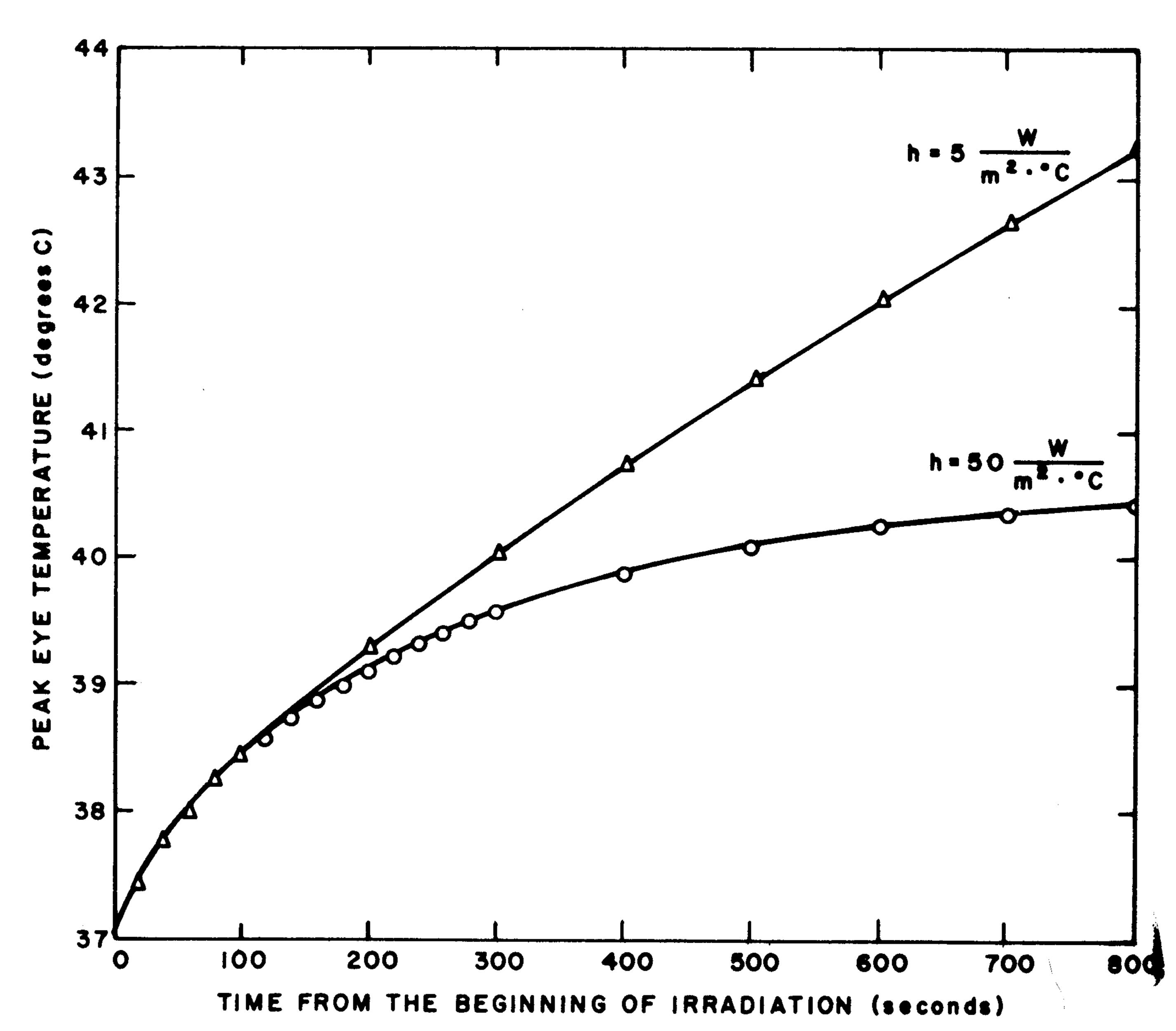
Fig. 9. Range of the peak eye temperature versus time for incident frequency = 1.5 GHz and  $P_{\rm inc} = 100 \, \rm mW/cm^2$ .
