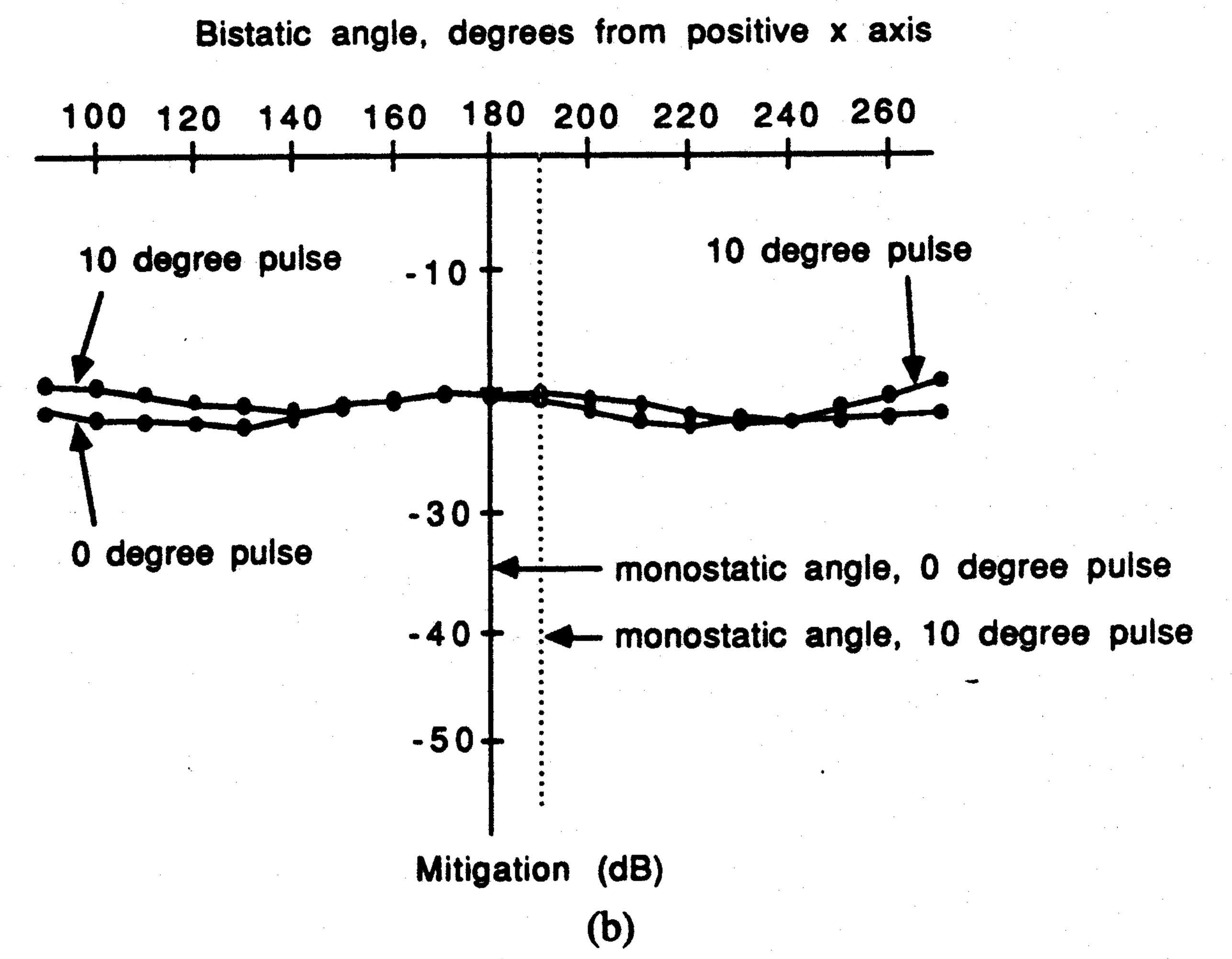
Synthesis results for the rounded conducting strip, isotropic coating case. (a) Final coating state after convergence of the synthesis algorithm. (b) Mitigation of the broad-band scattered pulse in the far field versus bistatic angle.
