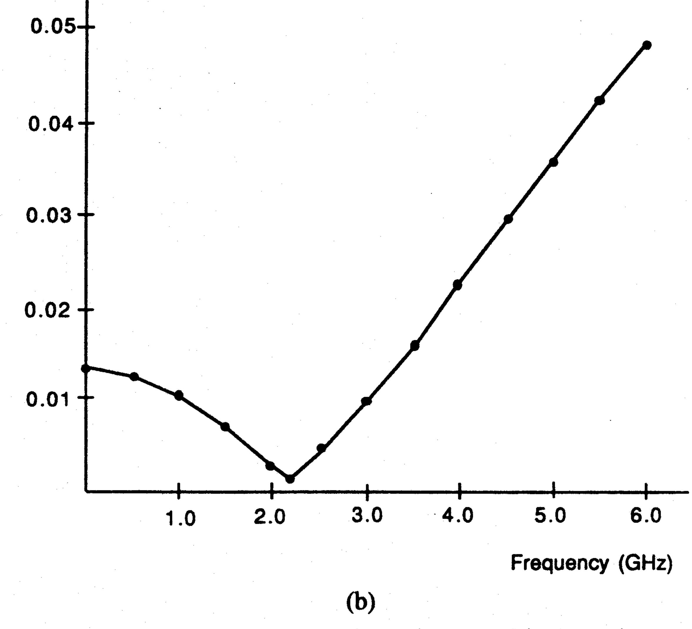
Synthesis example in one dimension. (a) Final coating state after convergence of the synthesis algorithm. (b) Reflection coefficient magnitude versus frequency for the synthesized coating over metal.
