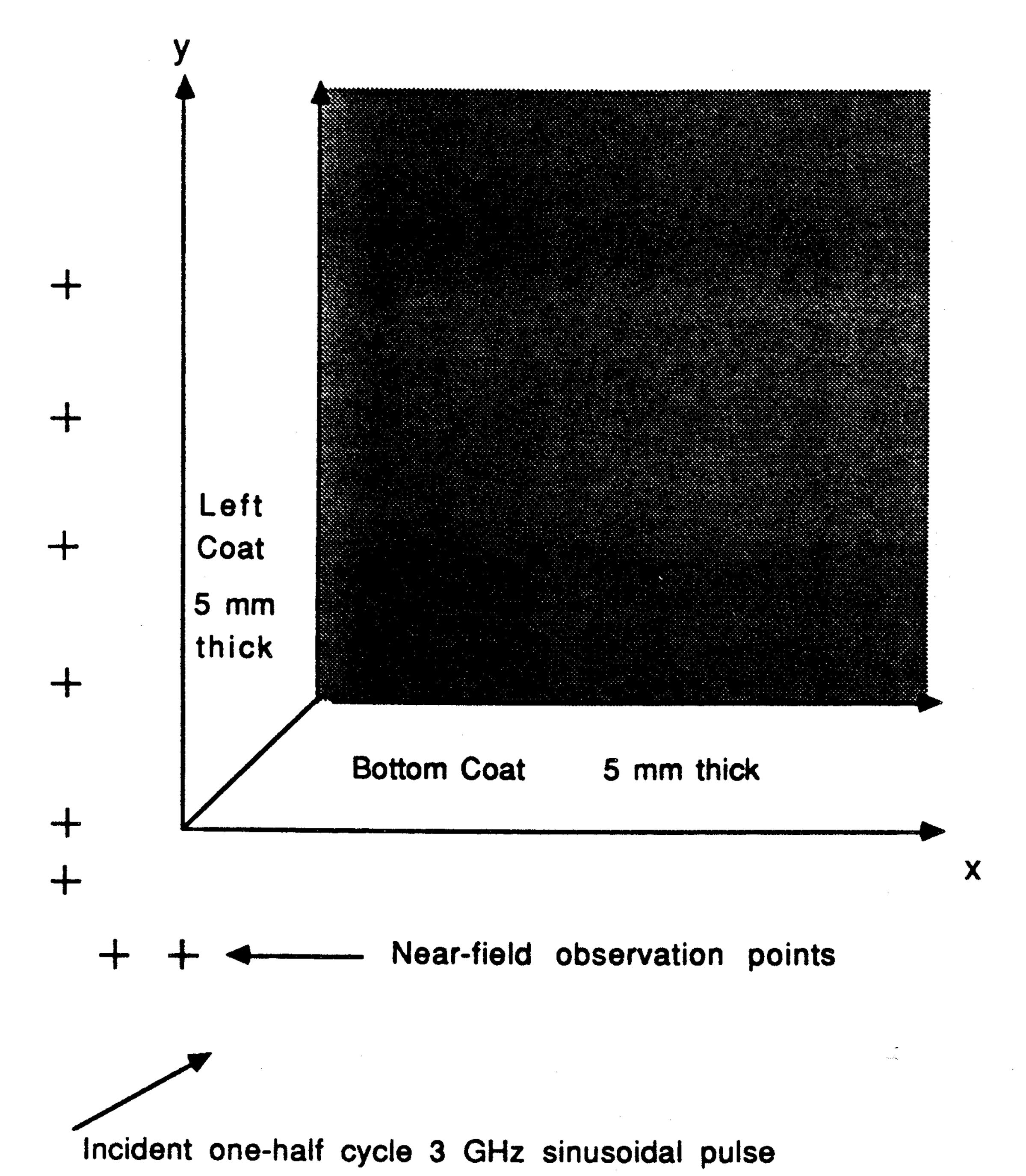
Fig. 3. Assumed geometry for the synthesis of absorbing coatings on an infinite, perfectly conducting, right-angle wedge.
