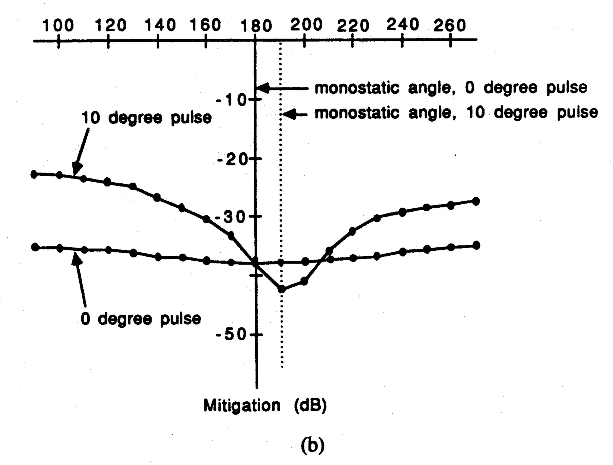
Fig. 8. Synthesis results for the rounded conducting strip, anisotropic coating case. (a) Final coating state after convergence of the synthesis algorithm. (b) Mitigation of the broad-band scattered pulse in the far field versus bistatic angle.
