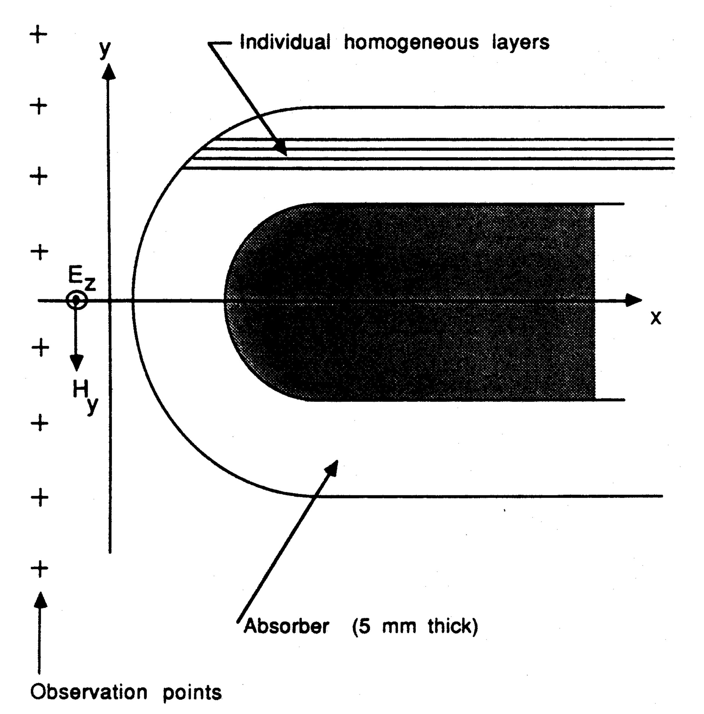
Fig. 6. Assumed geometry for the synthesis of absorbing coatings on an infinite, perfectly conducting strip of finite thickness with rounded edge.
