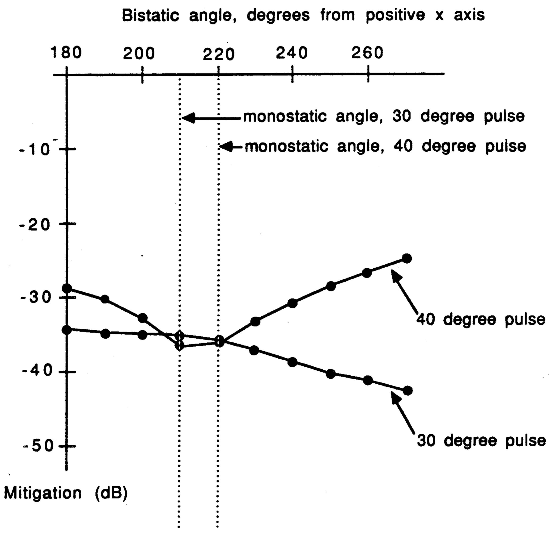
Fig. 4. Synthesis results for the conducting right-angle wedge, isotropic coating case. (a) Final coating state after convergence of the synthesis algorithm. (b) Mitigation of the broad-band scattered pulse in the far field versus bistatic angle.
