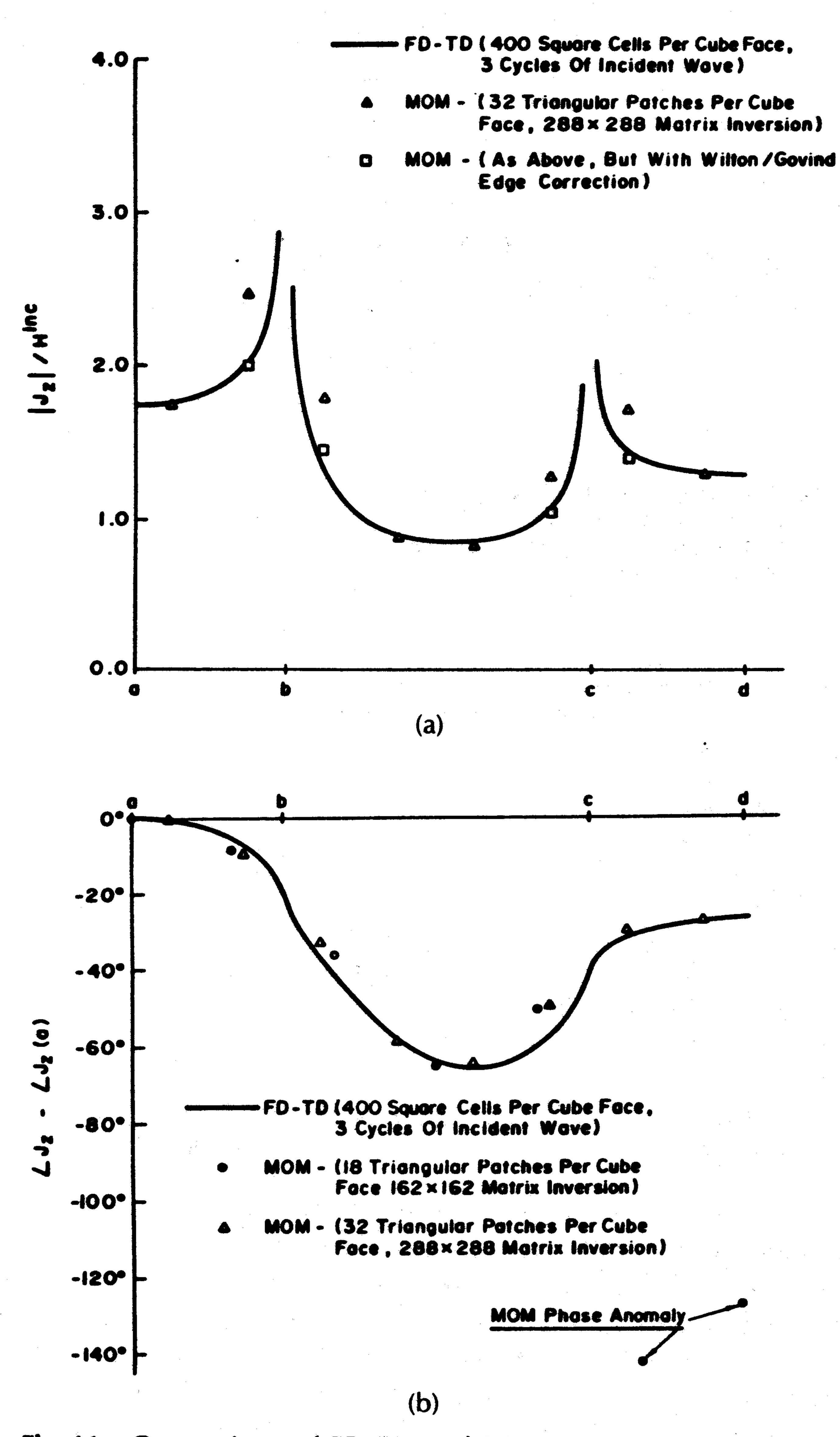
**Fig. 11.** Comparison of FD-TD and EFIE-MoM results for surface electric current distribution induced along H-plane locus of a perfectly conducting cube of size  $k_0 s = 2$ . (a) Magnitude. (b) Phase [13].
