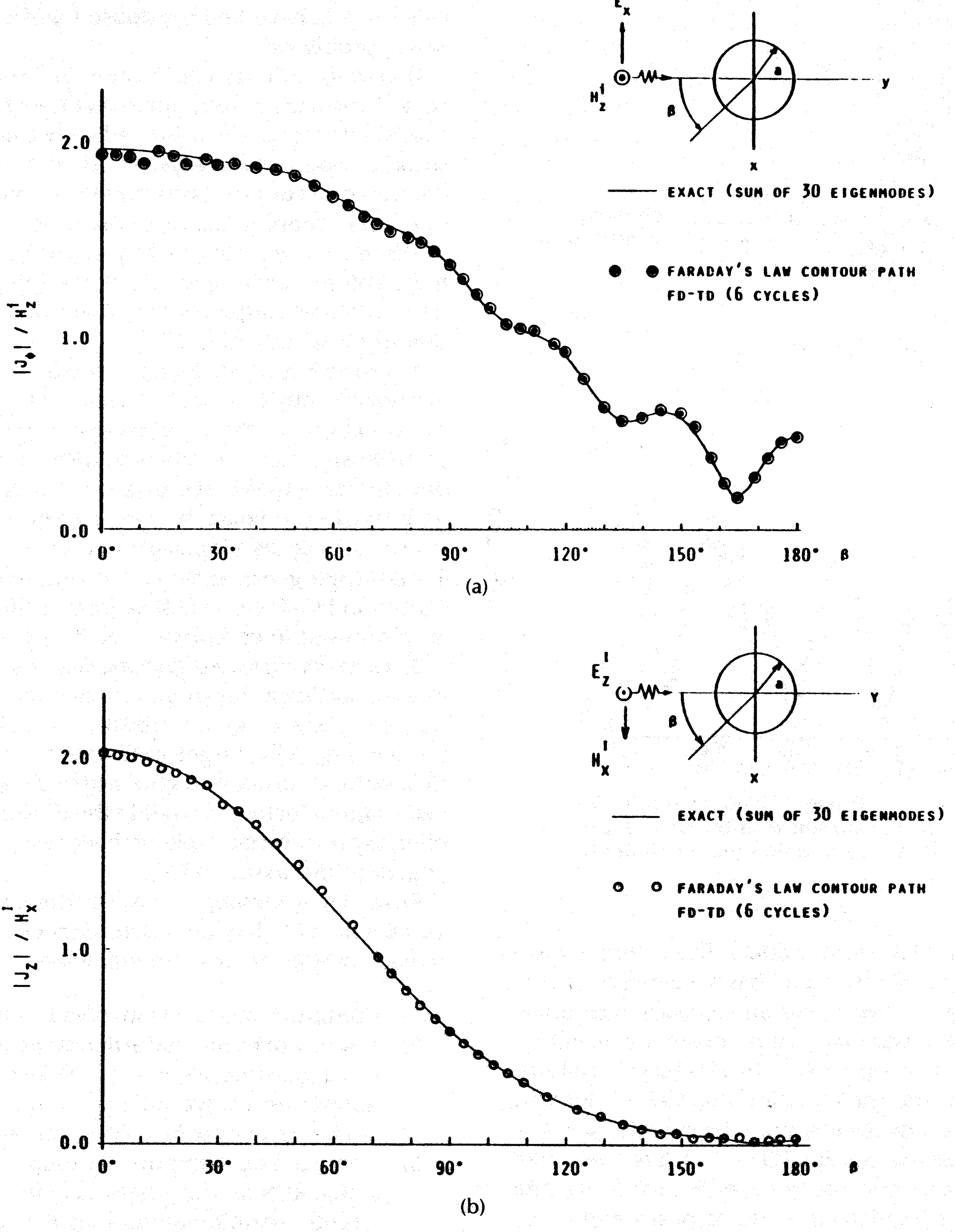
Fig. 7. Comparison of FD-TD and exact summed-eigenfunction solutions for surface electric current distribution induced on a  $k_0a = 5$  circular conducting cylinder (conformal FD-TD model used, 0.05 wavelength grid cell size). (a) TE case, azimuthal current. (b) TM case, longitudinal current [27].
