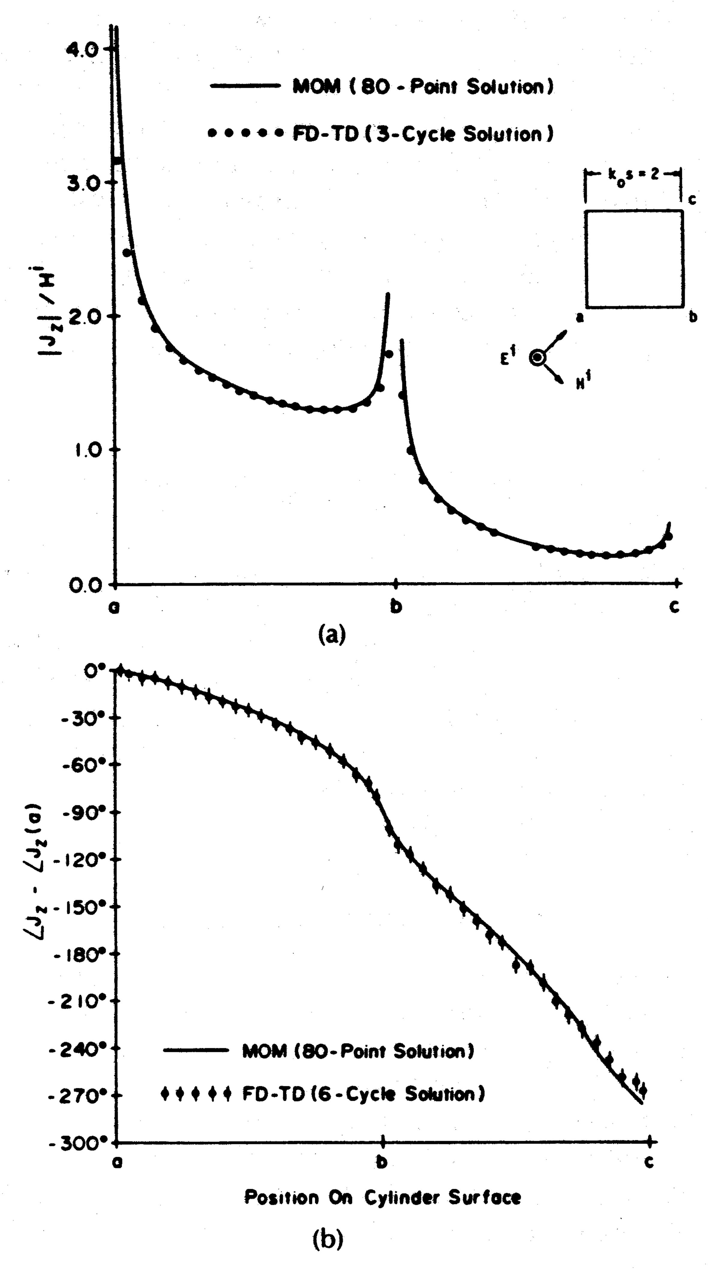
Fig. 4. Comparison of FD-TD and EFIE-MoM results for longitudinal surface electric current distribution induced on a perfectly conducting square cylinder of size  $k_0 s = 2$ . (a) Magnitude. (b) Phase [12].
