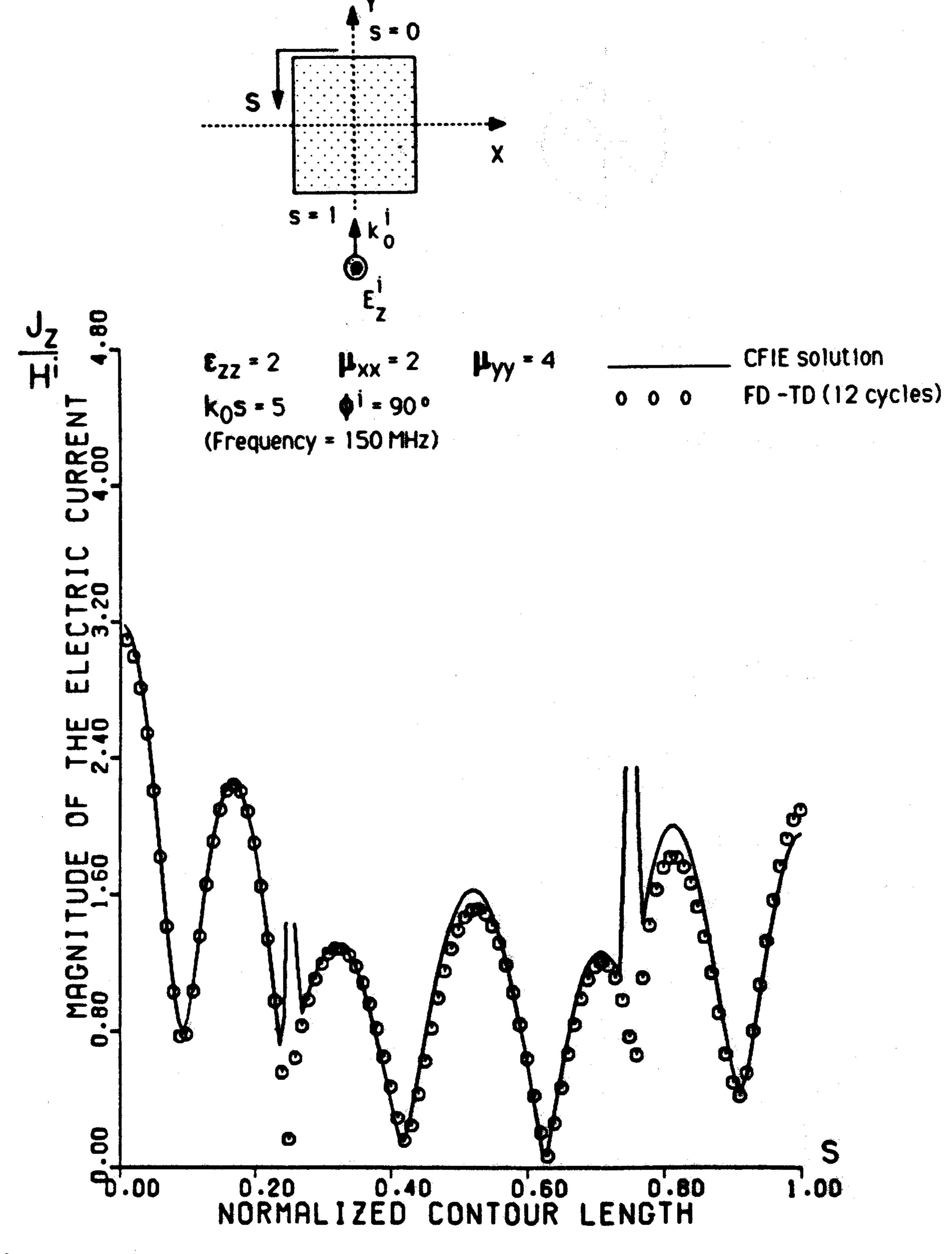
Fig. 6. Comparison of FD-TD and CFIE-MoM results for longitudinal surface electric current distribution induced on an anisotropic dielectric-permeable square cylinder of size  $k_0 s = 5$ , TM case [23].
