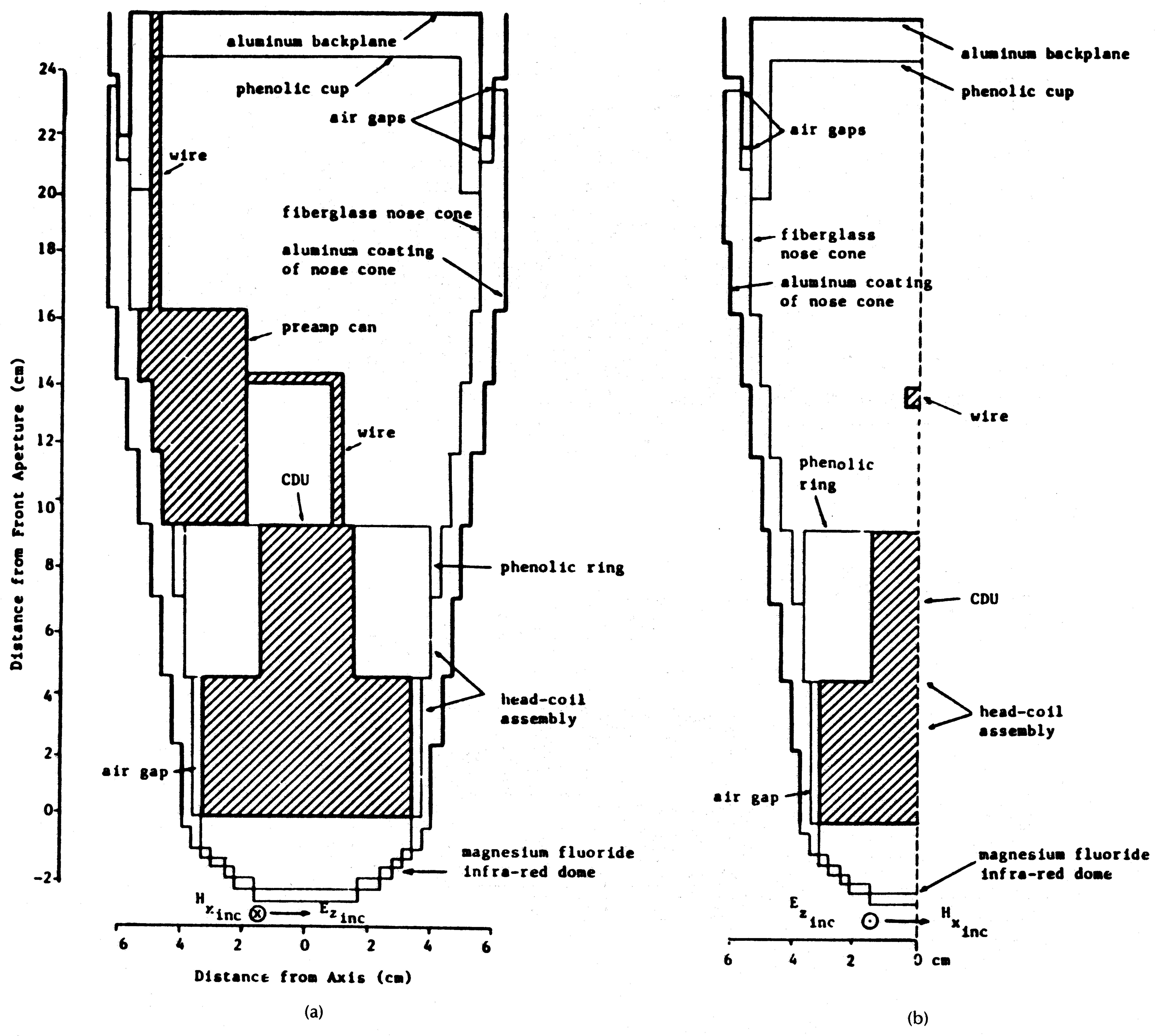
Fig. 14. Three-dimensional FD-TD model of missile seeker section showing component materials. (a) At vertical symmetry plane. (b) At horizontal observation plane [5], [7].
