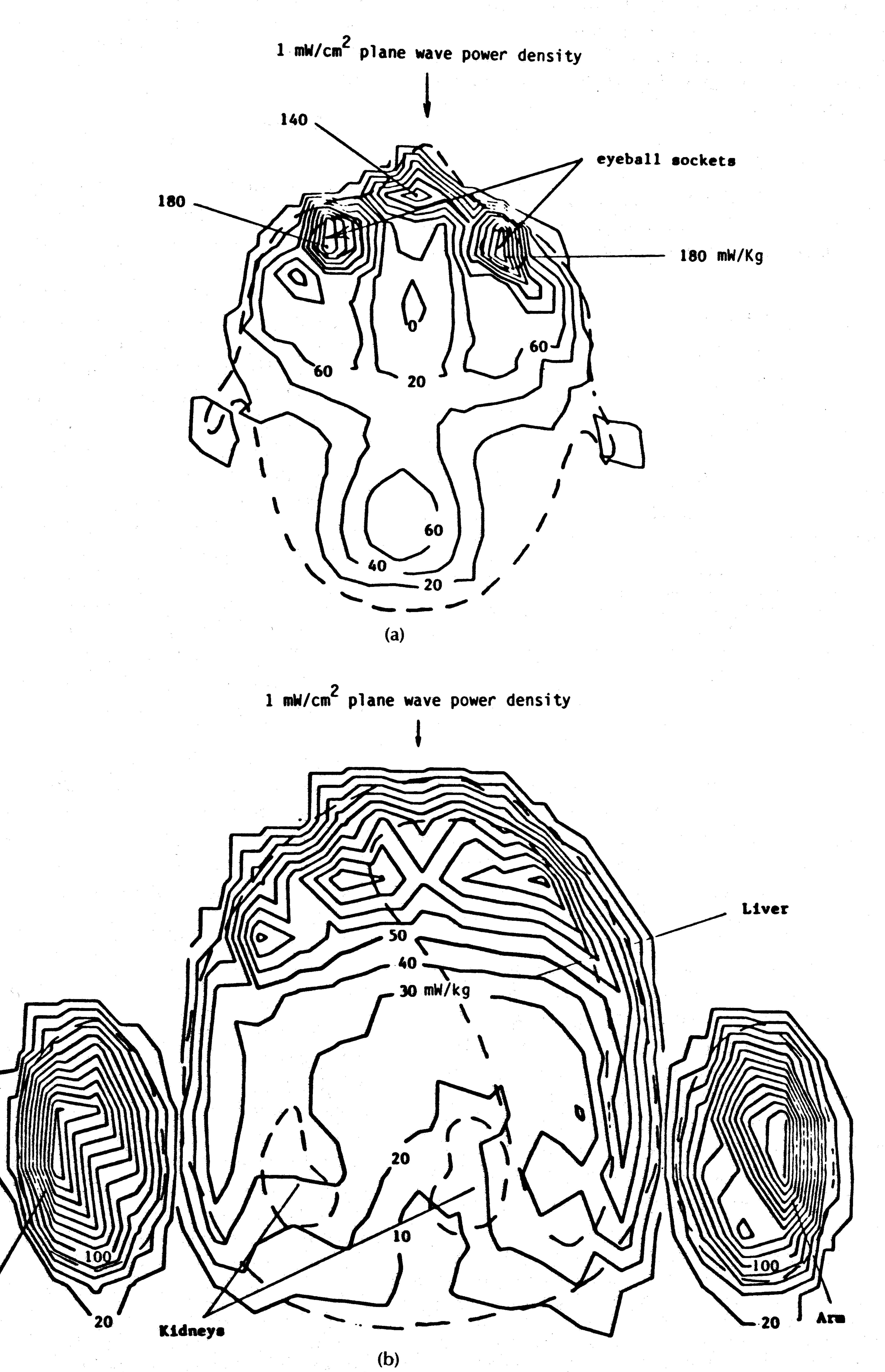
Fig. 16. FD-TD computed contour maps of specific absorption rate (SAR) due to penetrating electromagnetic fields within a highly realistic three-dimensional model of the entire human body. (a) Along horizontal cut through head at 350 MHz. (b) Along horizontal cut through liver at 100 MHz [34].
