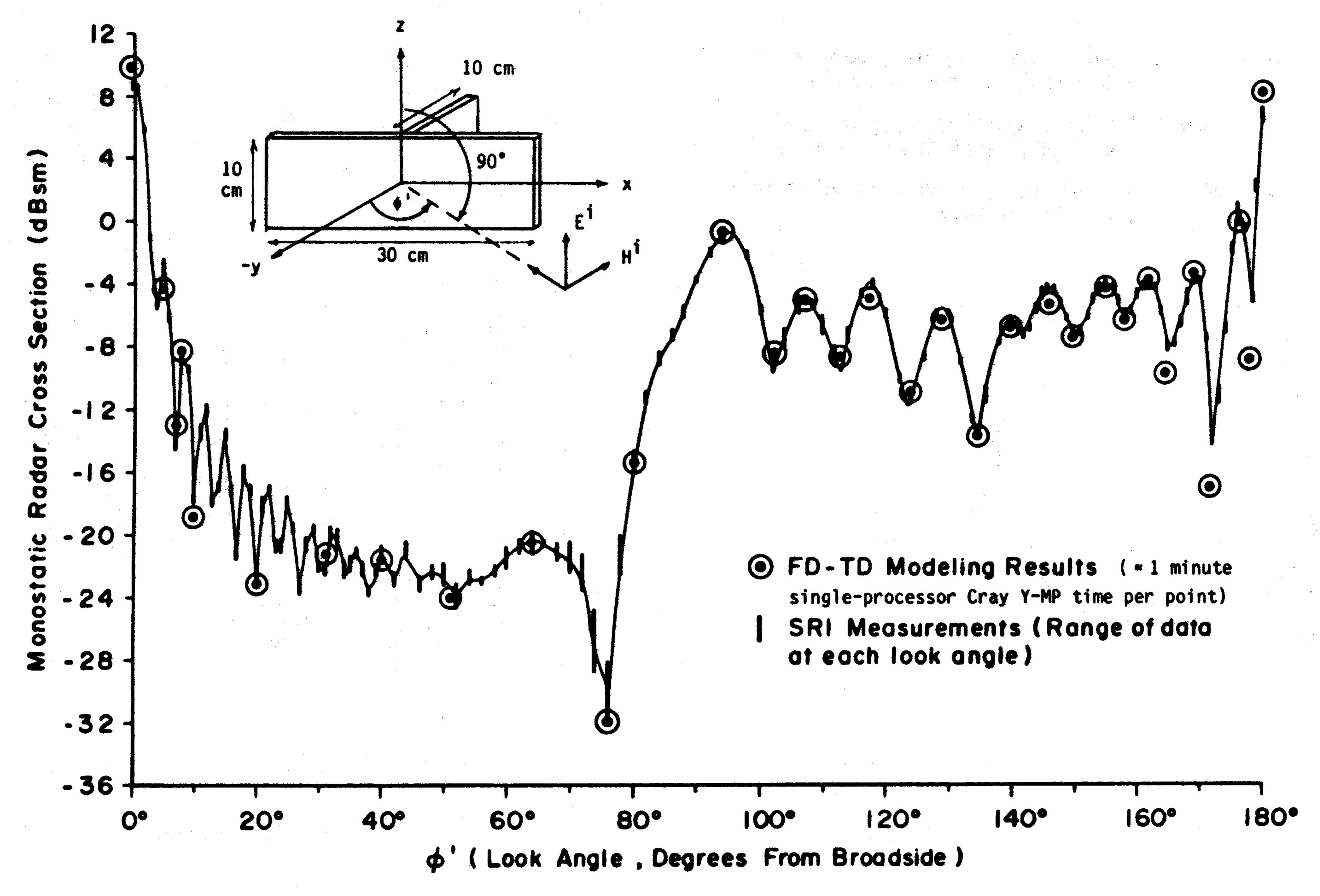
Fig. 13. Experimental validation of FD-TD modeling predictions of monostatic radar cross section versus azimuth for crossed-plate target at 9 GHz (main plate size  $9 \times 3$  wavelengths, bisecting fin size  $3 \times 3$  wavelengths) [14], [24].
