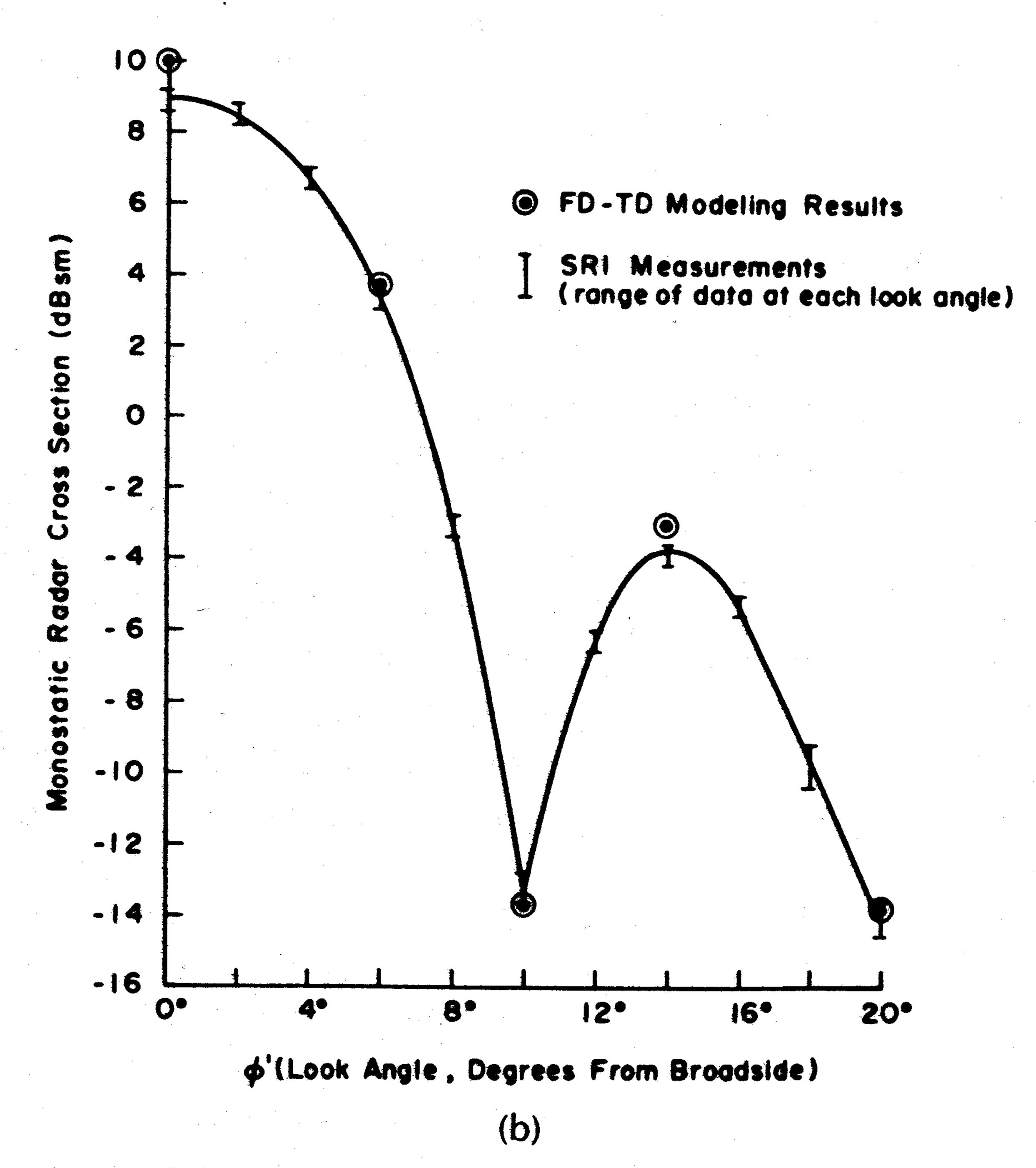
Fig. 12. Validation of FD-TD results for monostatic radar cross section of flat conducting plate. (a) Versus EFIE-MoM at 1 GHz (plate size  $1 \times 1/3$  wavelength). (b) Versus SRI measurements at 9 GHz (plate size  $9 \times 3$  wavelengths) [14], [24].
