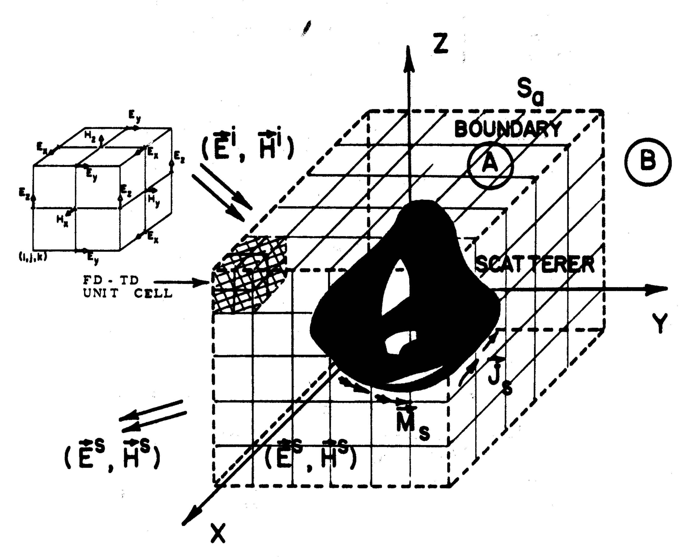
Fig. 2. Arbitrary three-dimensional scatterer embedded in FD-TD space lattice.
