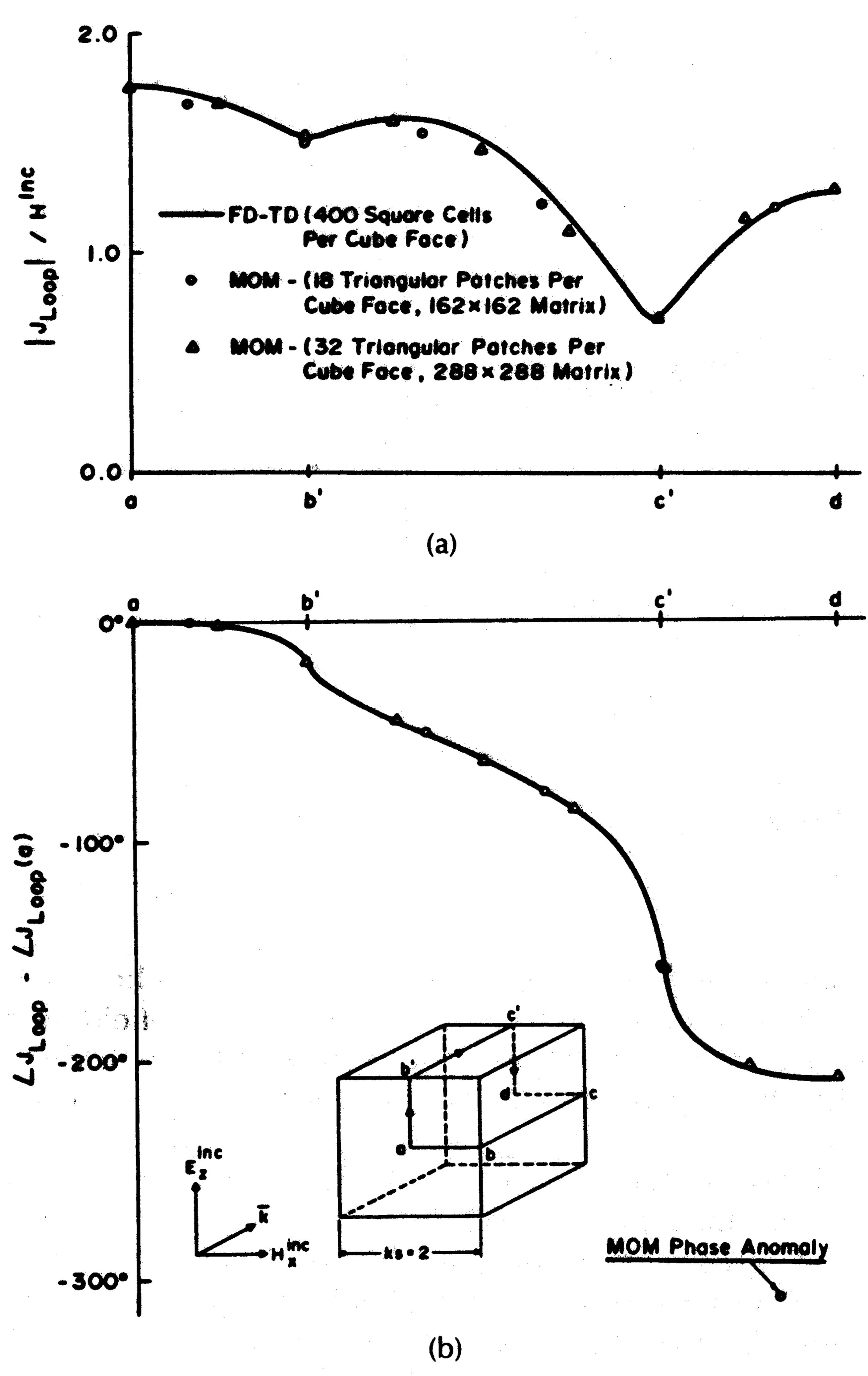
**Fig. 10.** Comparison of FD-TD and EFIE-MoM results for surface electric current distribution induced along *E*-plane locus of a perfectly conducting cube of size  $k_0 s = 2$ . (a) Magnitude. (b) Phase [13].
