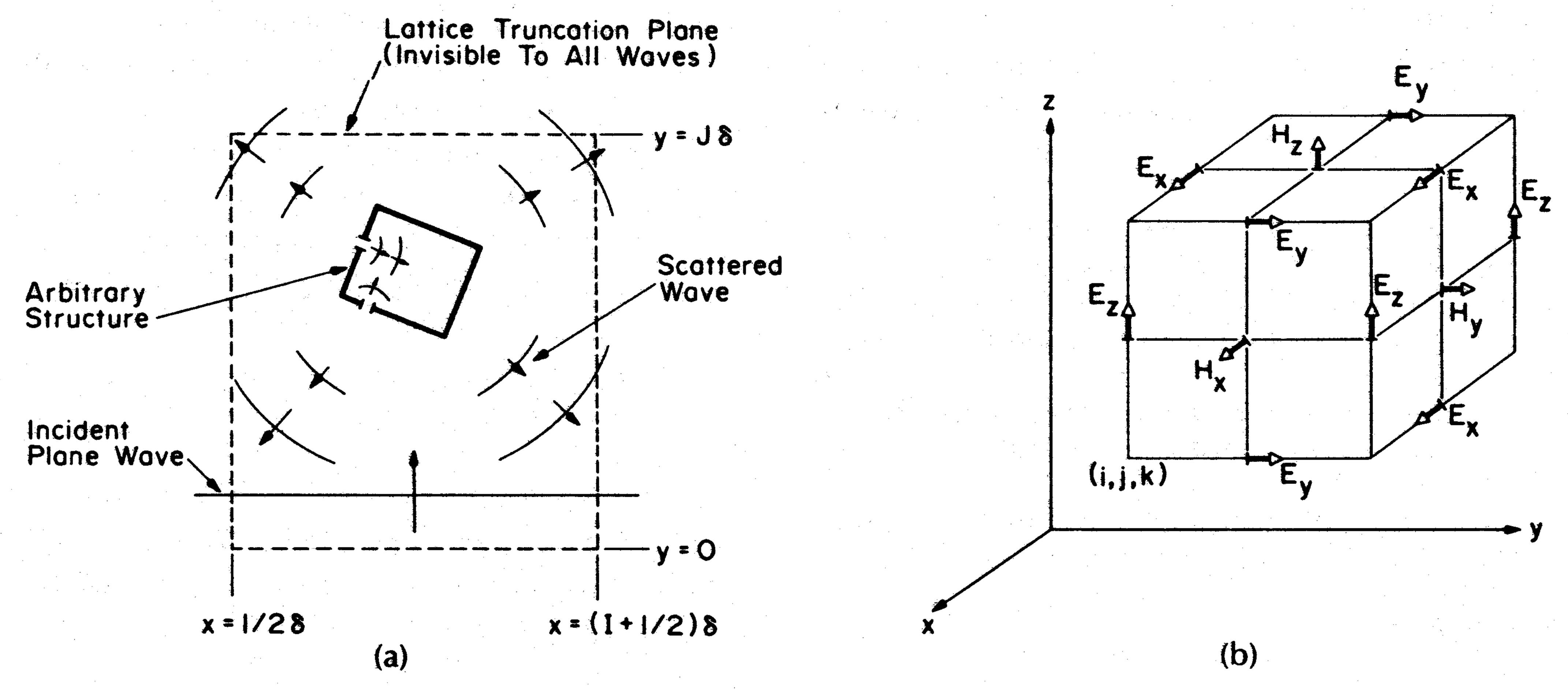
Fig. 1. Basic elements of FD-TD space lattice. (a) Time-domain wave tracking concept. (b) Lattice unit cell in Cartesian coordinates [1].
