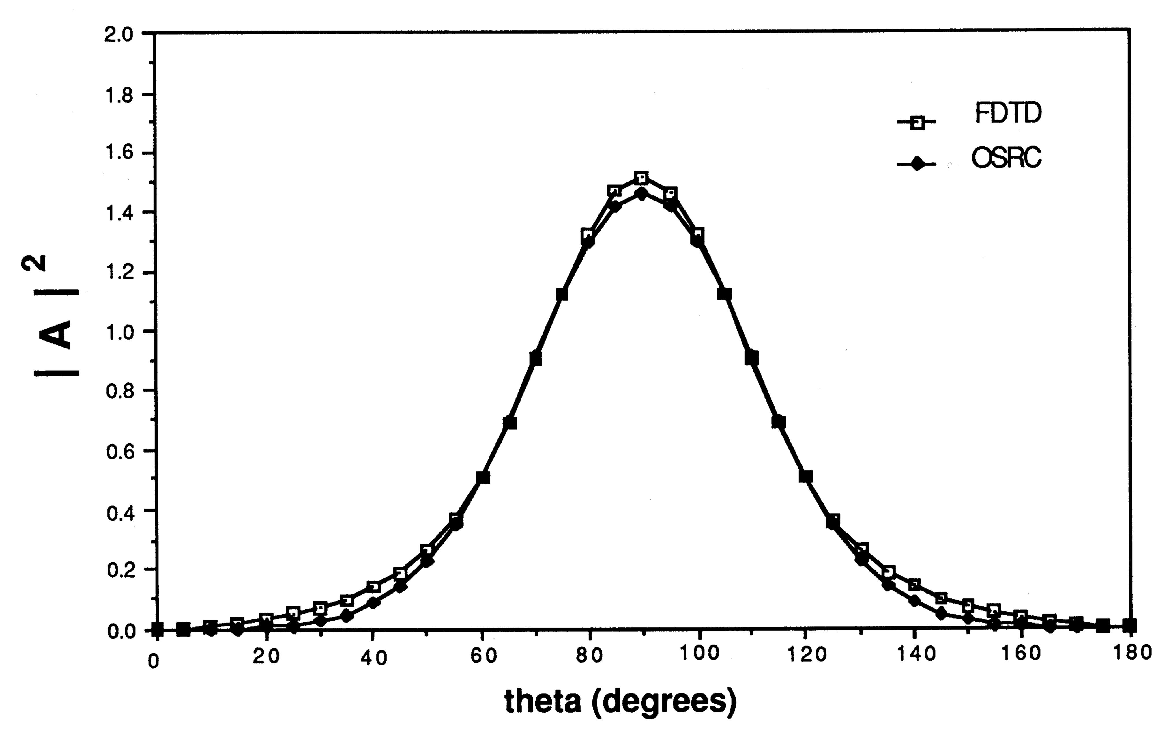
Fig. 6. Bistatic cross-section for the field scattered from the aperture of the infinite waveguide in the region z < 0 for  $\alpha = 0^{\circ}$ . The angle  $\theta$  is as shown in Fig. 1.
