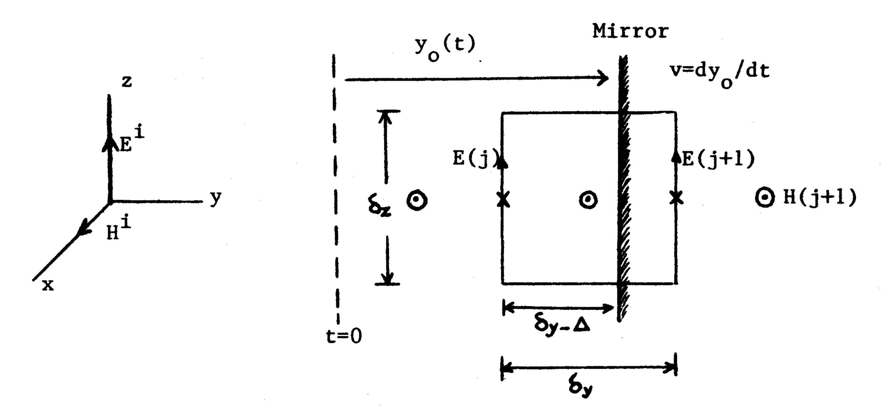
Fig. 1. FD-TD field component geometry for the moving mirror case in a one-dimensional FD-TD grid.
