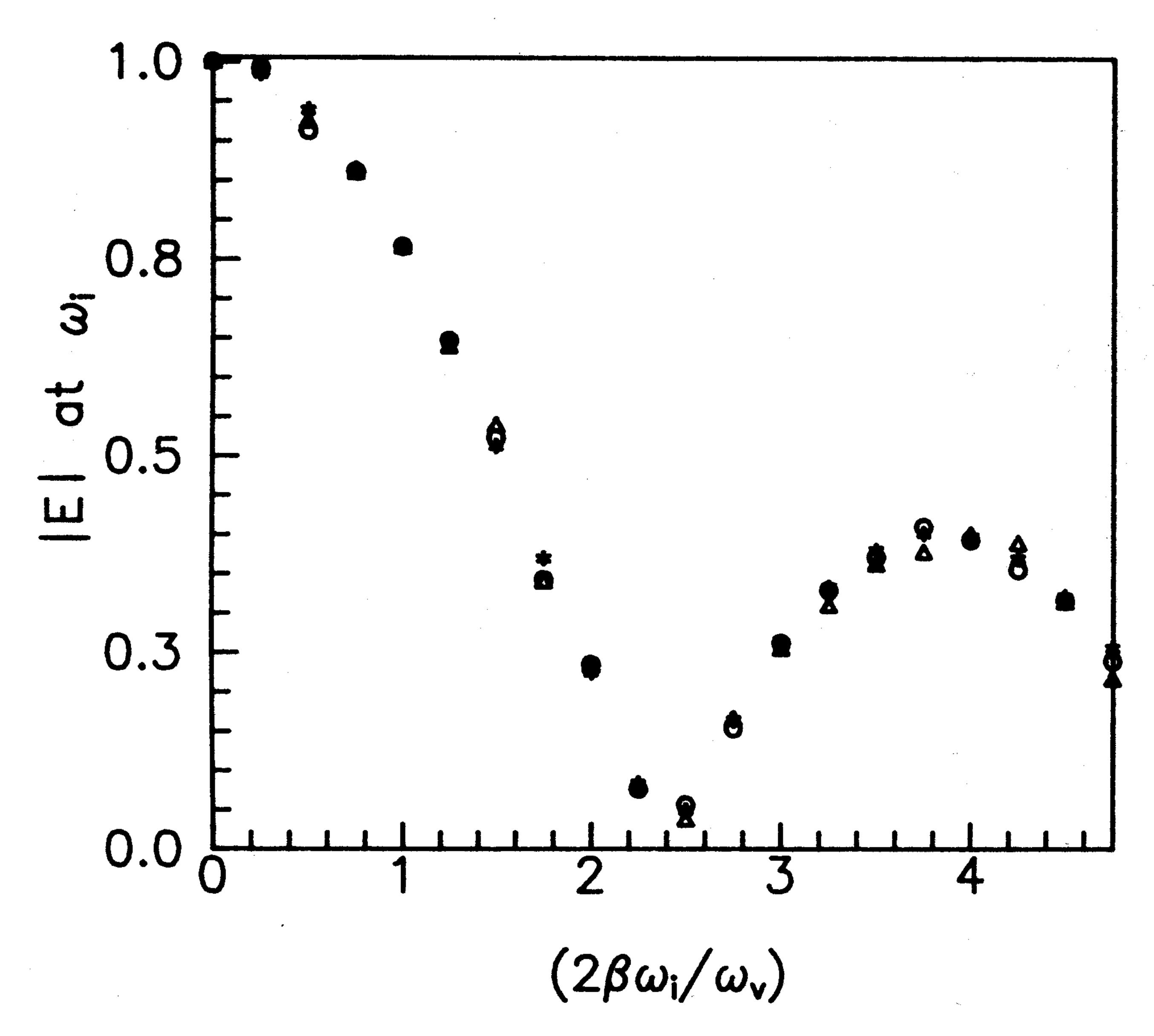
Fig. 3. Comparison of FD-TD and analytical results for the scattered field magnitude at the illumination frequency. \*: exact values; o: FD-TD values for  $\omega_i = 5\omega_v$ ;  $\triangle$ : FD-TD values for  $\beta = 0.1c$ .
