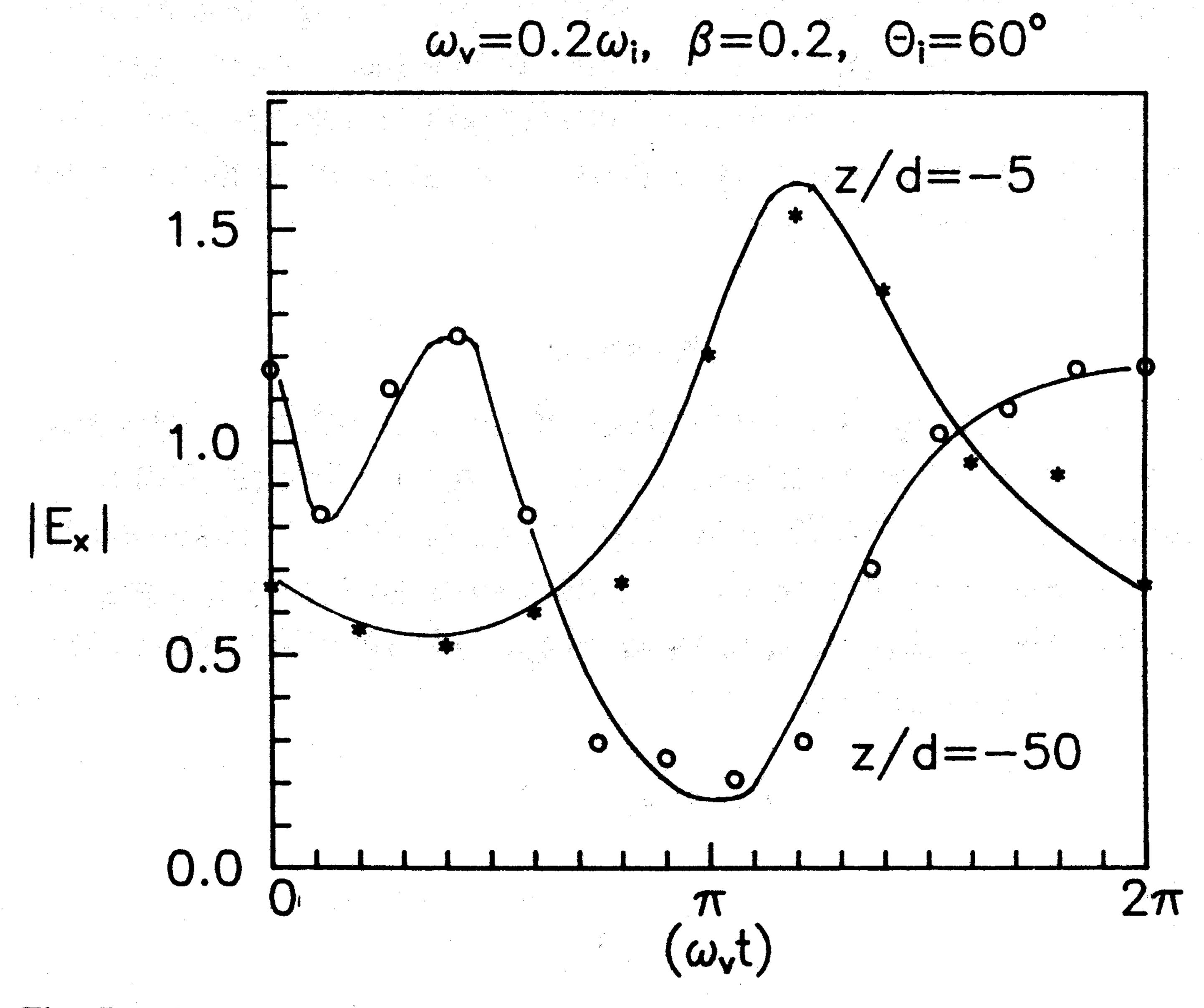
Comparison of FD-TD and analytical results for the scattered field time envelope at oblique incidence. —: analytical results; \*0: FD-TD results.
