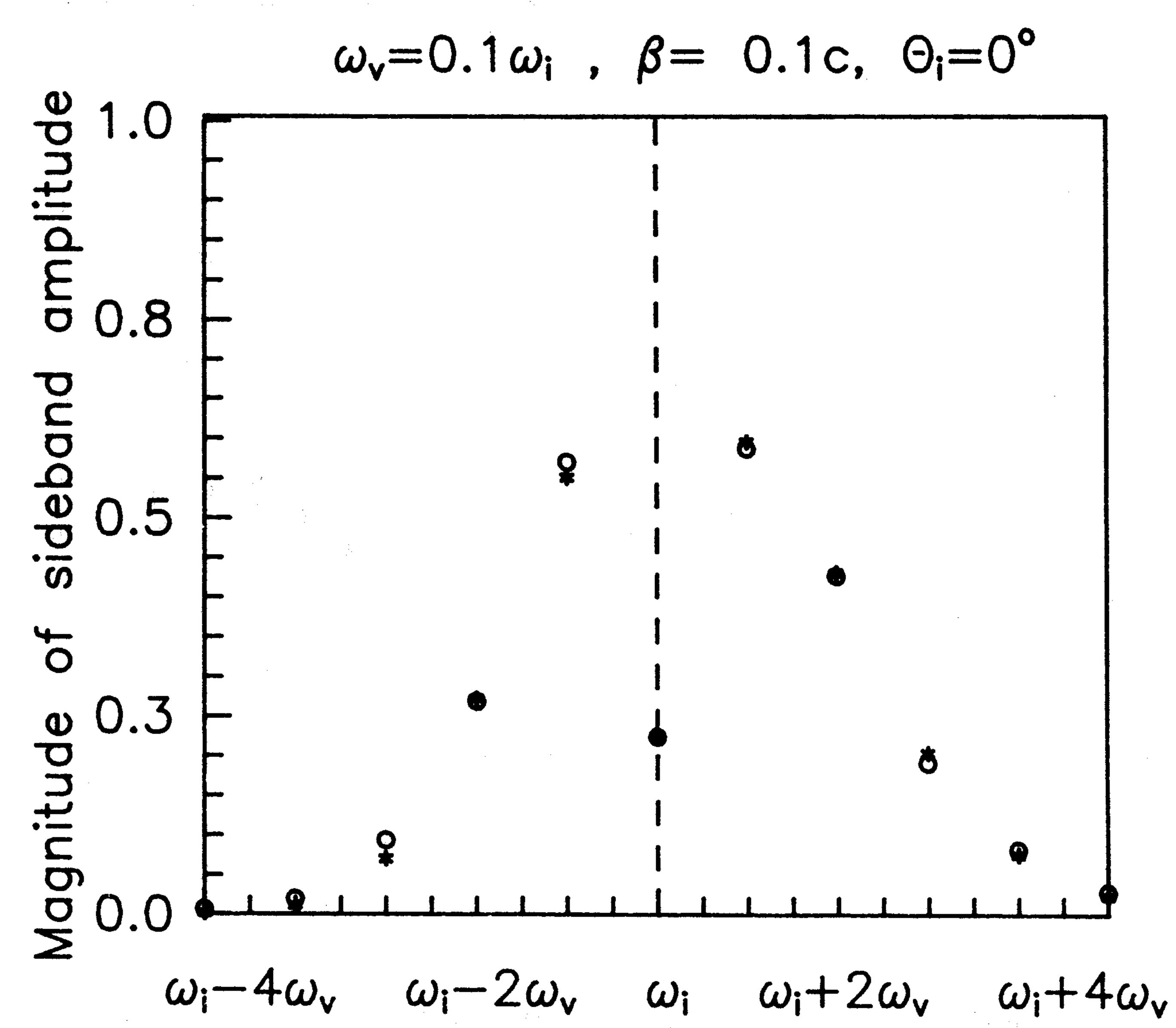
Fig. 2. Comparison of FD-TD and analytical results for the sidebands of the reflected spectrum. \*: exact values; o: FD-TD values.
