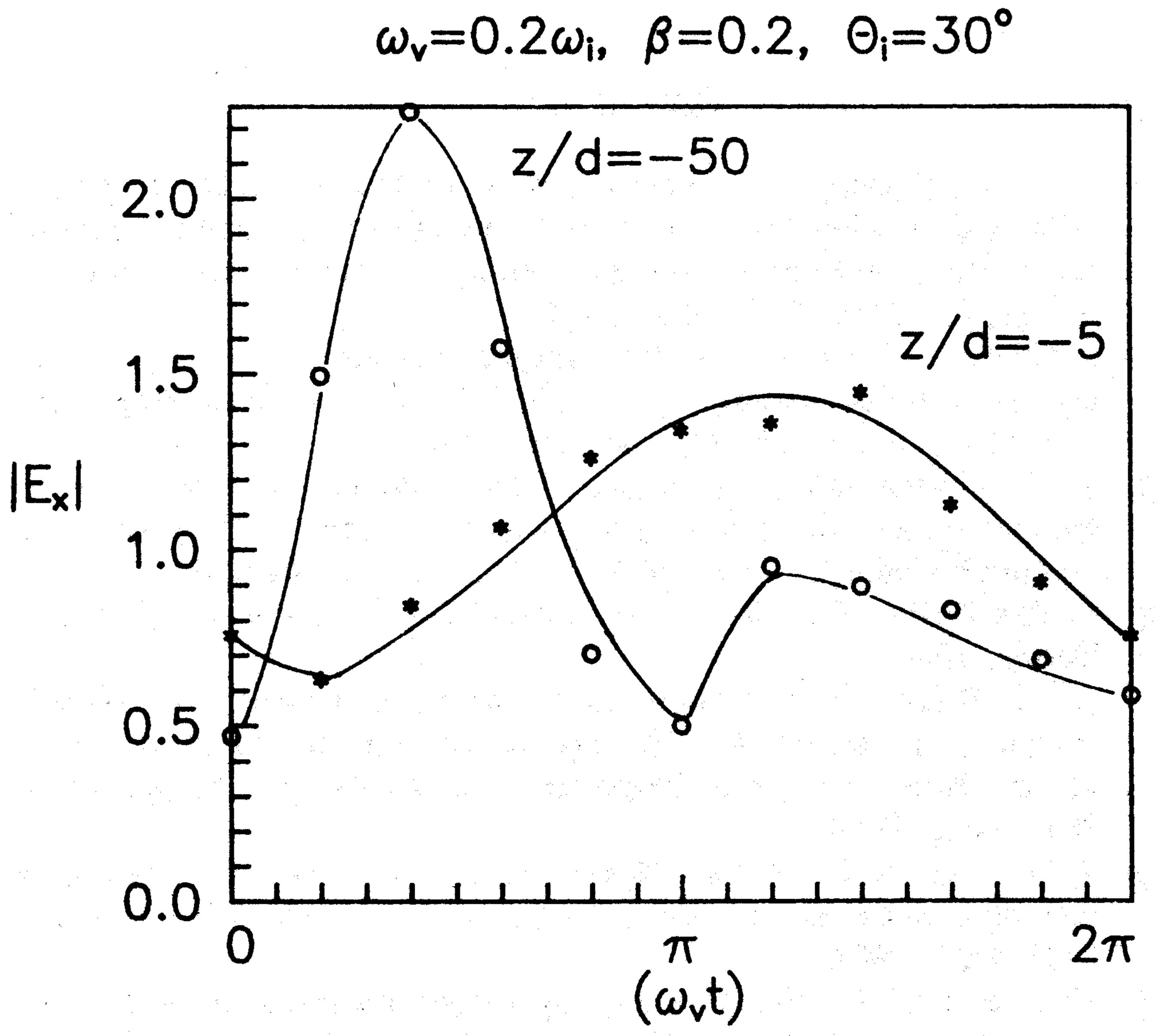
Comparison of FD-TD ana analytical results for the scattered field time envelope at oblique incidence. —: analytical results; \*o: FD-TD results.
