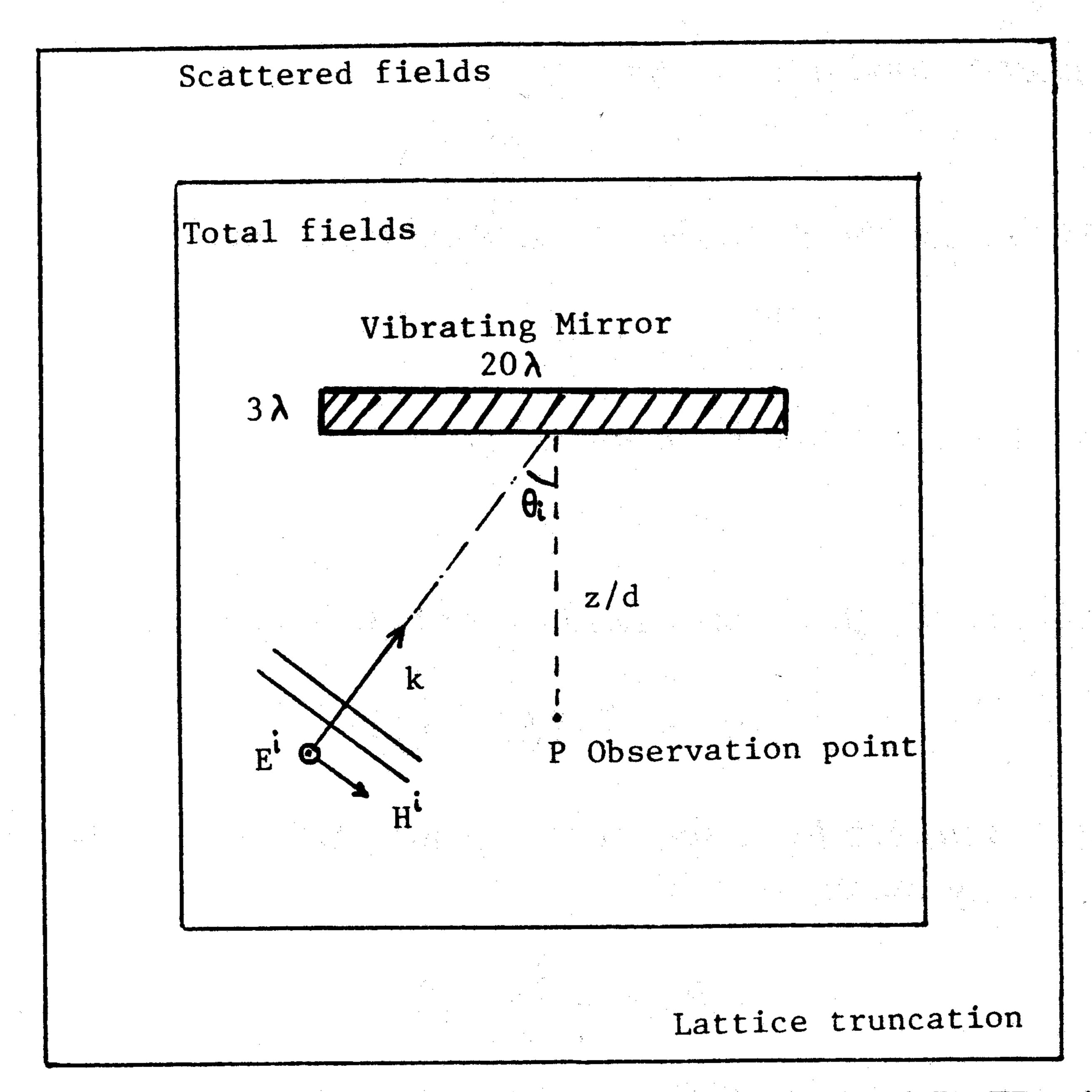
Modeling of a vibrating mirror in a two-dimensional FD-TD grid.
