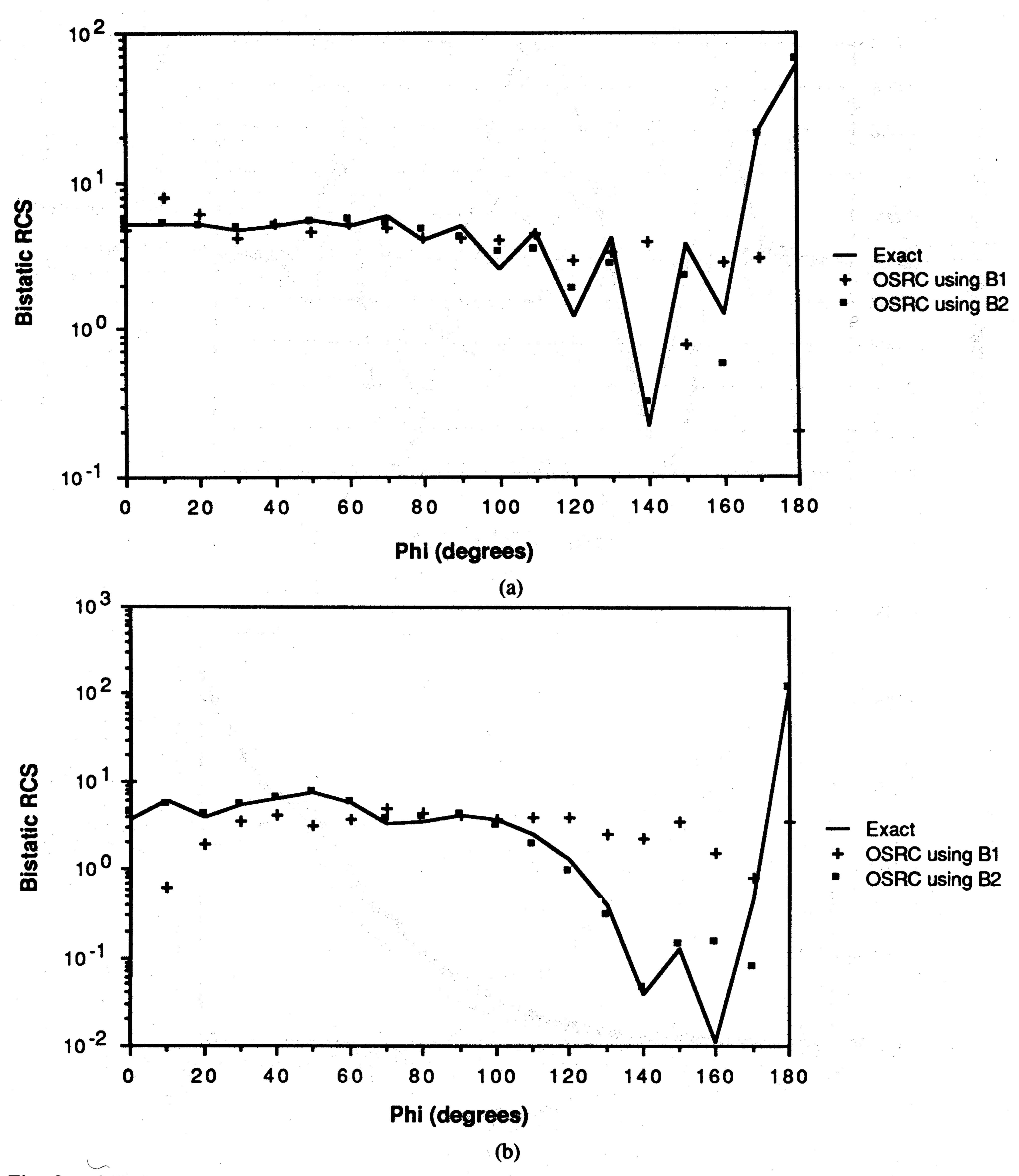
Fig. 8. OSRC computed bistatic RCS of conducting circular cylinder, TE case. (a) ka = 10. (b) ka = 20.
