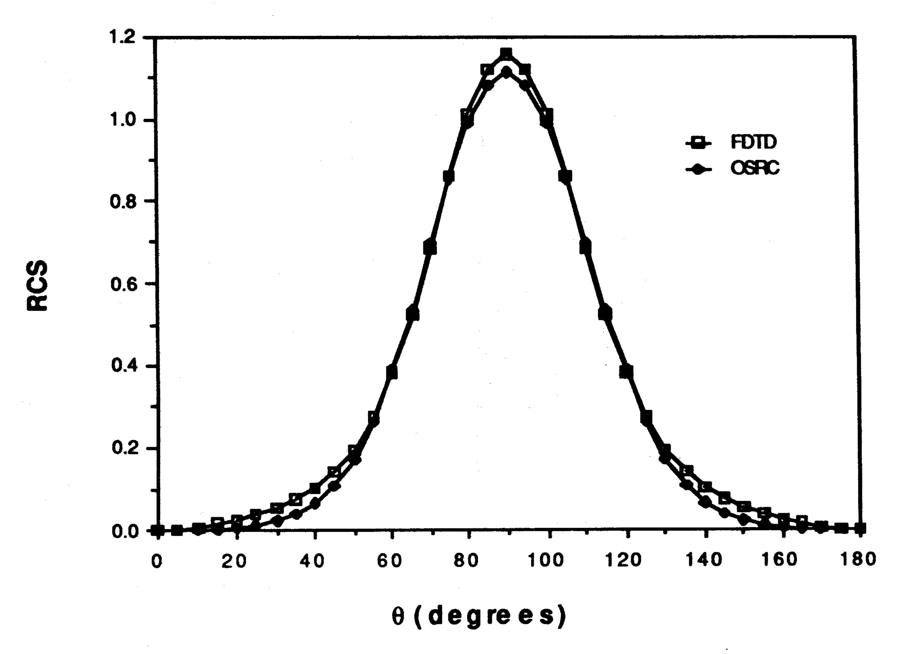
Fig. 12. Bistatic cross section for scattering from waveguide aperture due to plane wave at  $\alpha = 0^{\circ}$  and f = 250 MHz. Angle  $\theta$  is as shown in Fig. 11.
