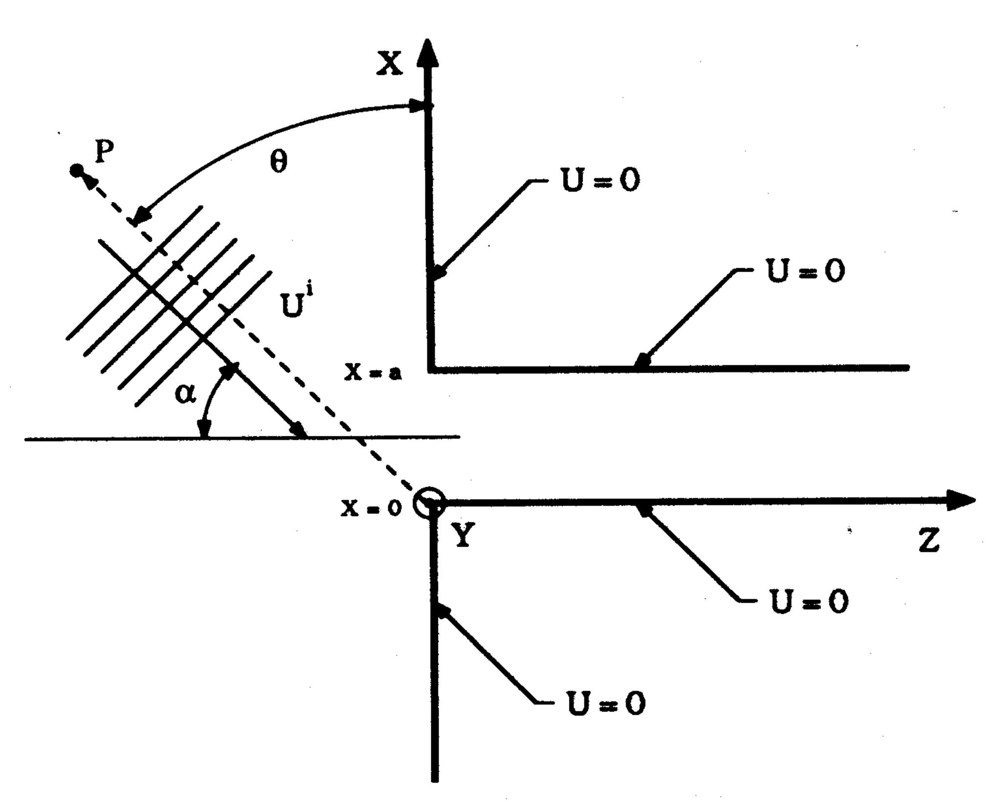
Fig. 11. Plane wave incident on open end of flanged, semi-infinite parallelplate waveguide. a = 1.5 m, f = 250 MHz.
