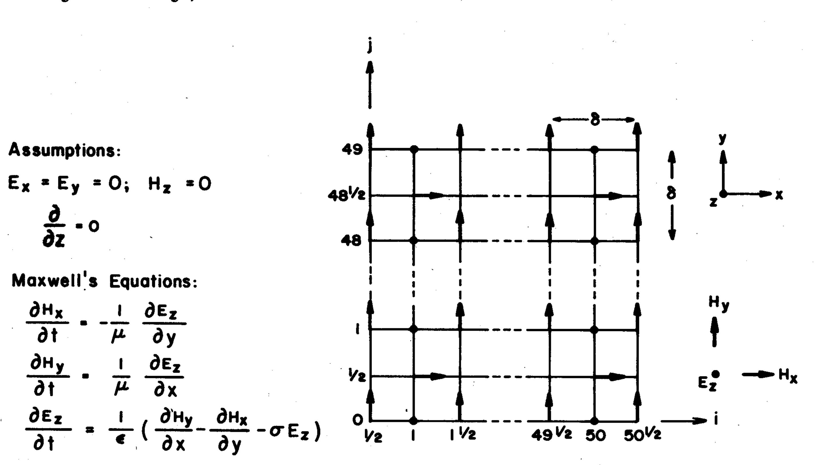
Fig. 3. Two-dimensional lattice, illustrating a set of approximate soft lattice truncation conditions.
