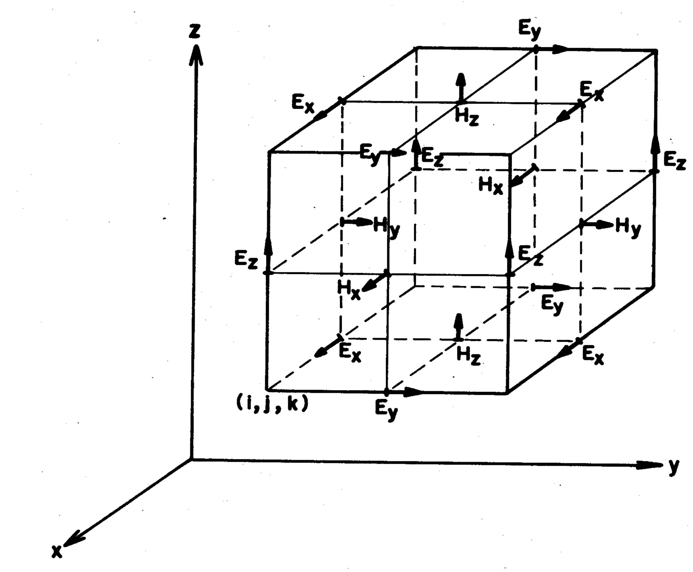
Fig. 1. Positions of the field components about a unit cell of the
