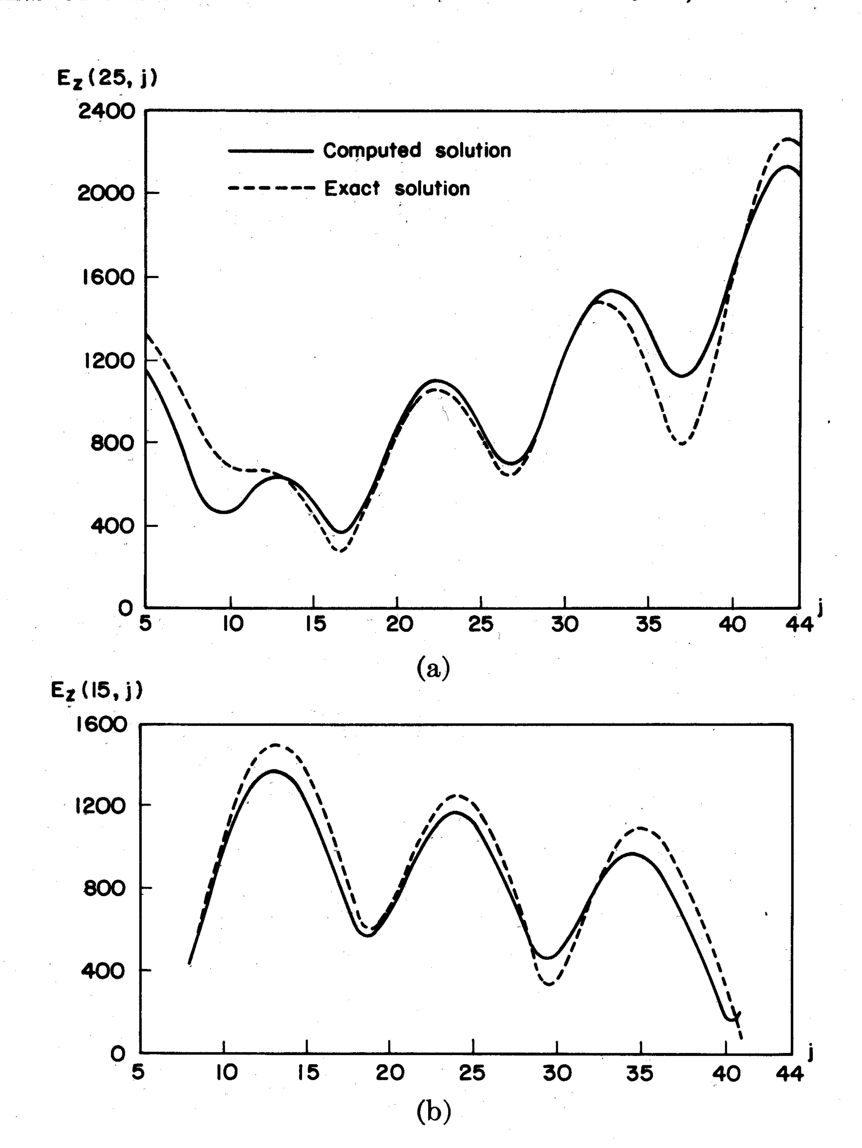
Fig. 6. Results of the first cylinder scatterer program.
