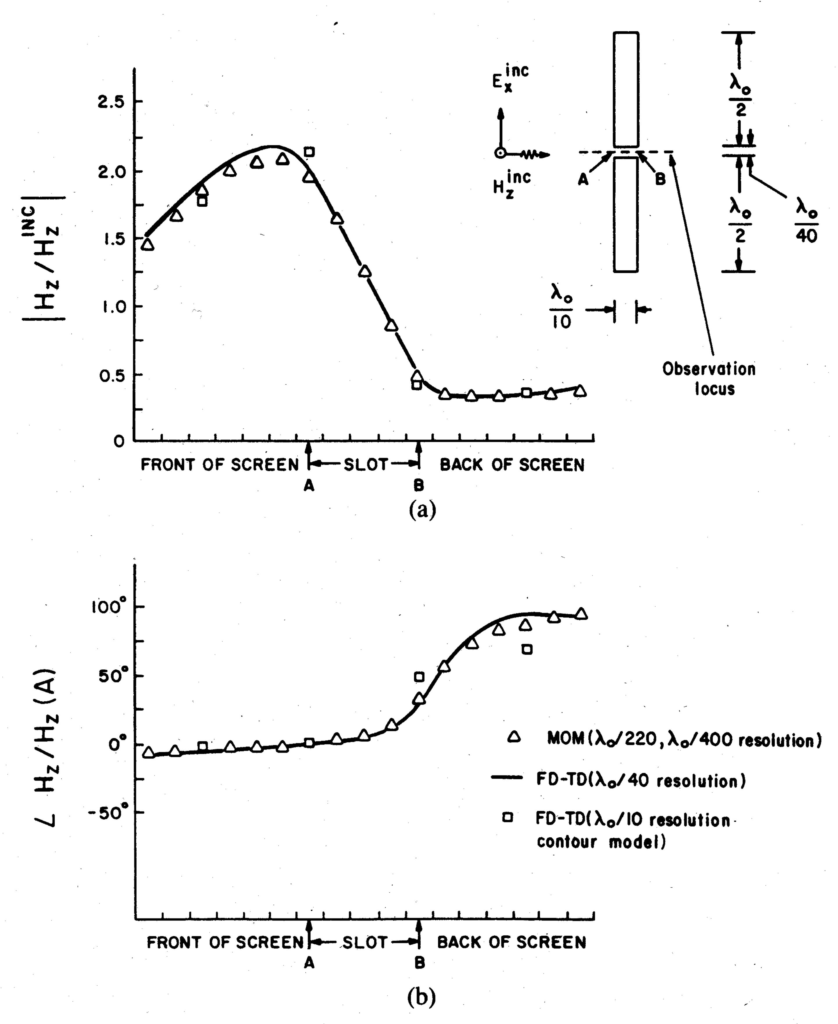
Fig. 7. Comparison of FD-TD and MM solutions for gap magnetic field distribution, straight-slot case. (a) Magnitude. (b) Phase.
