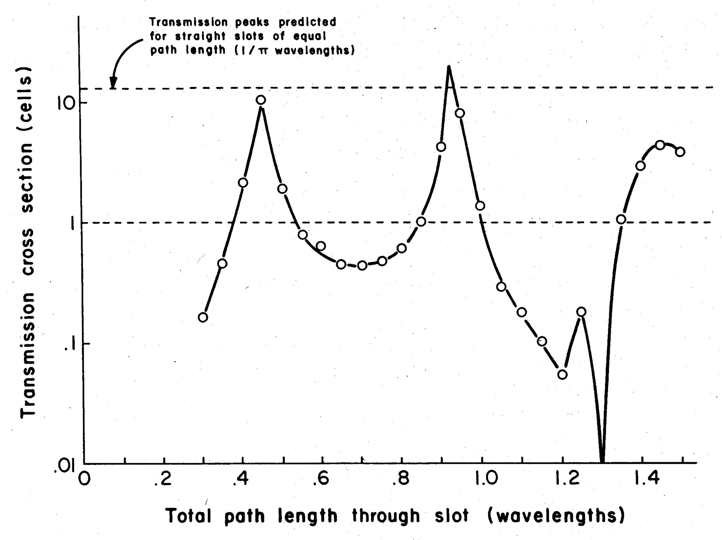
Fig. 11. Transmission cross section of U-shaped lapped joint.
