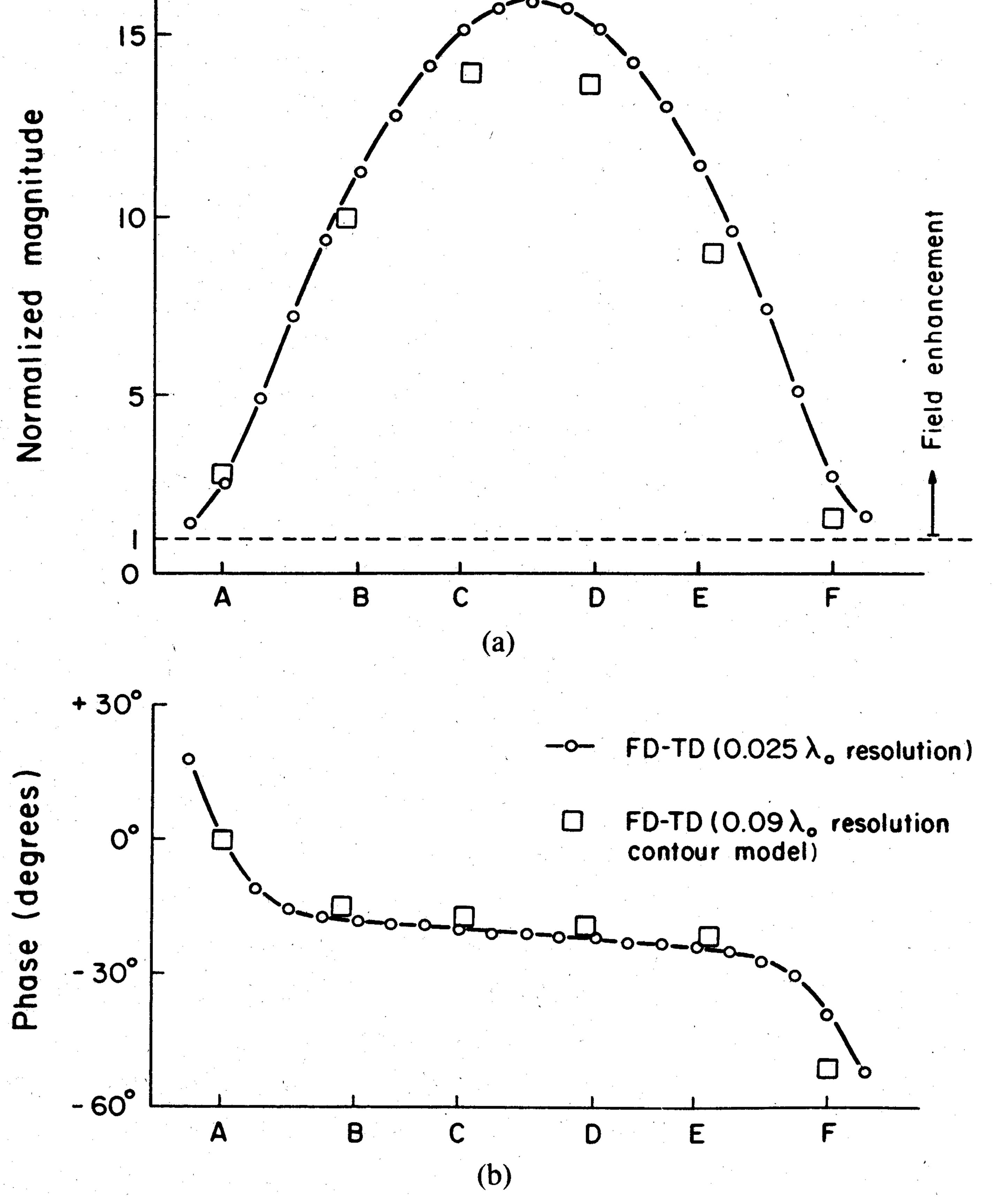
Fig. 13. FD-TD computed magnetic field within 0.45-wavelength path length, U-shaped lapped joint. (a)  $|H_{gap}/H_{inc}|$ . (b)  $\angle H_{gap}/H_z(A)$ .
