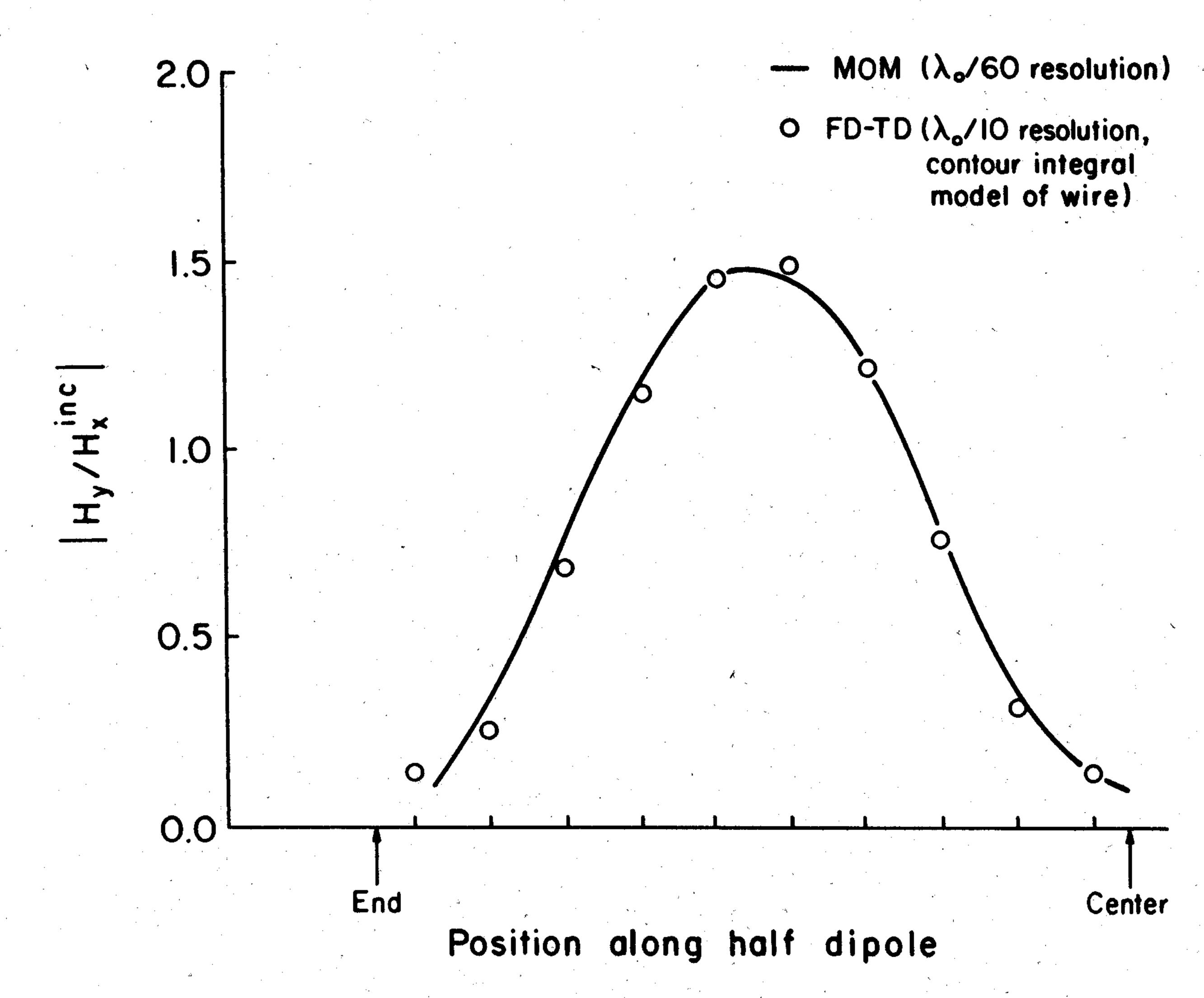
Fig. 4. Comparison of FD-TD and MM solutions for scattered circumferential magnetic field distribution along 2.0-wavelength (antiresonant) wire of radius 1/300 wavelength (broadside TM illumination).
