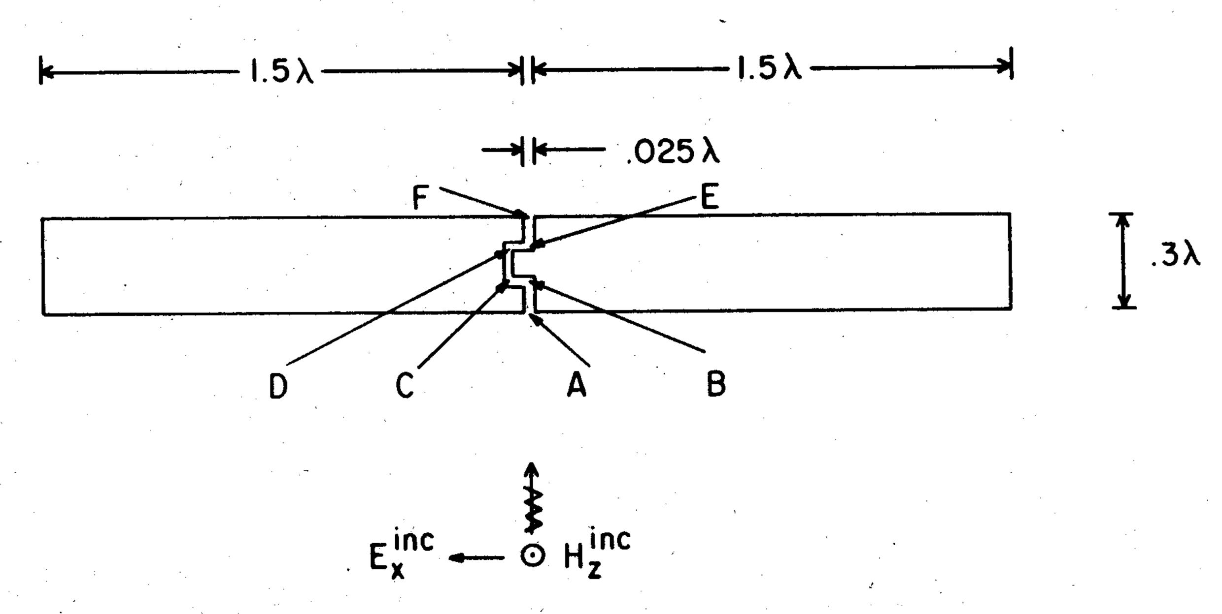
Fig. 10. Geometry of U-shaped lapped joint for TE illumination, shown to scale.
