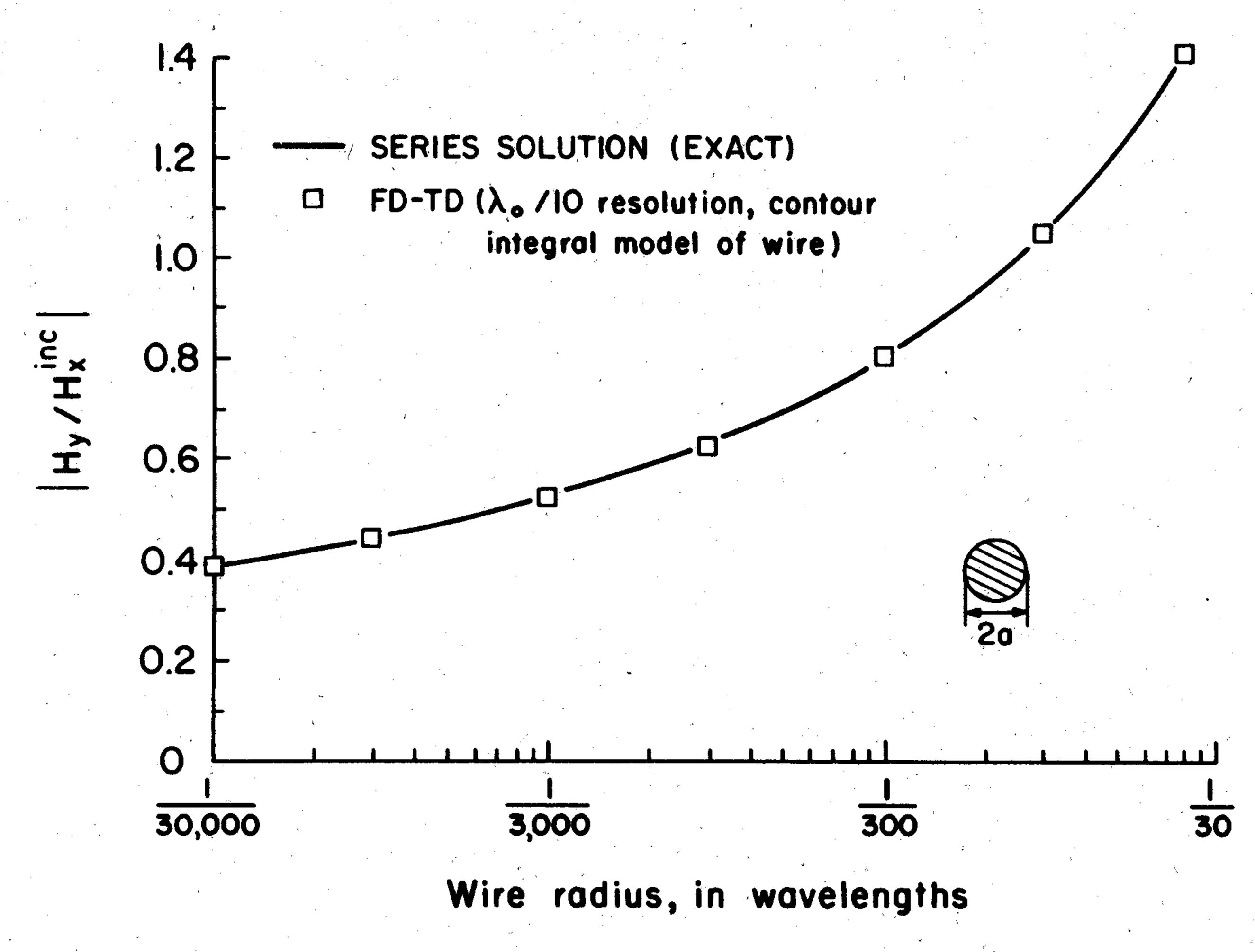
Fig. 3. Comparison of FD-TD and eigenfunction expansion solutions for scattered circumferential magnetic field at point 1/20 wavelength from center of infinite wire.
