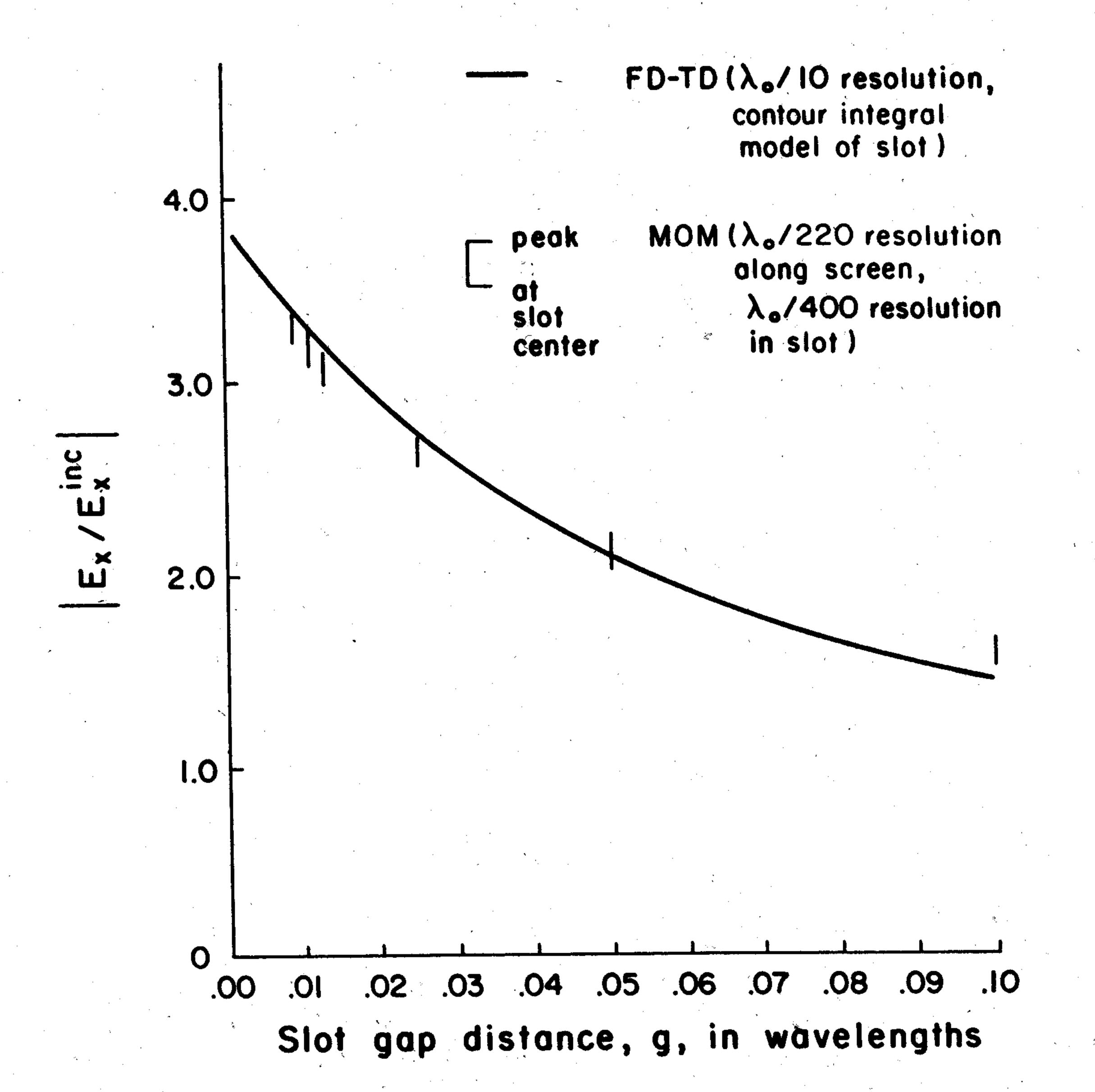
Fig. 9. Comparison of FD-TD contour model and MM calculations for variation of gap electric field with gap distance, straight-slot case.
