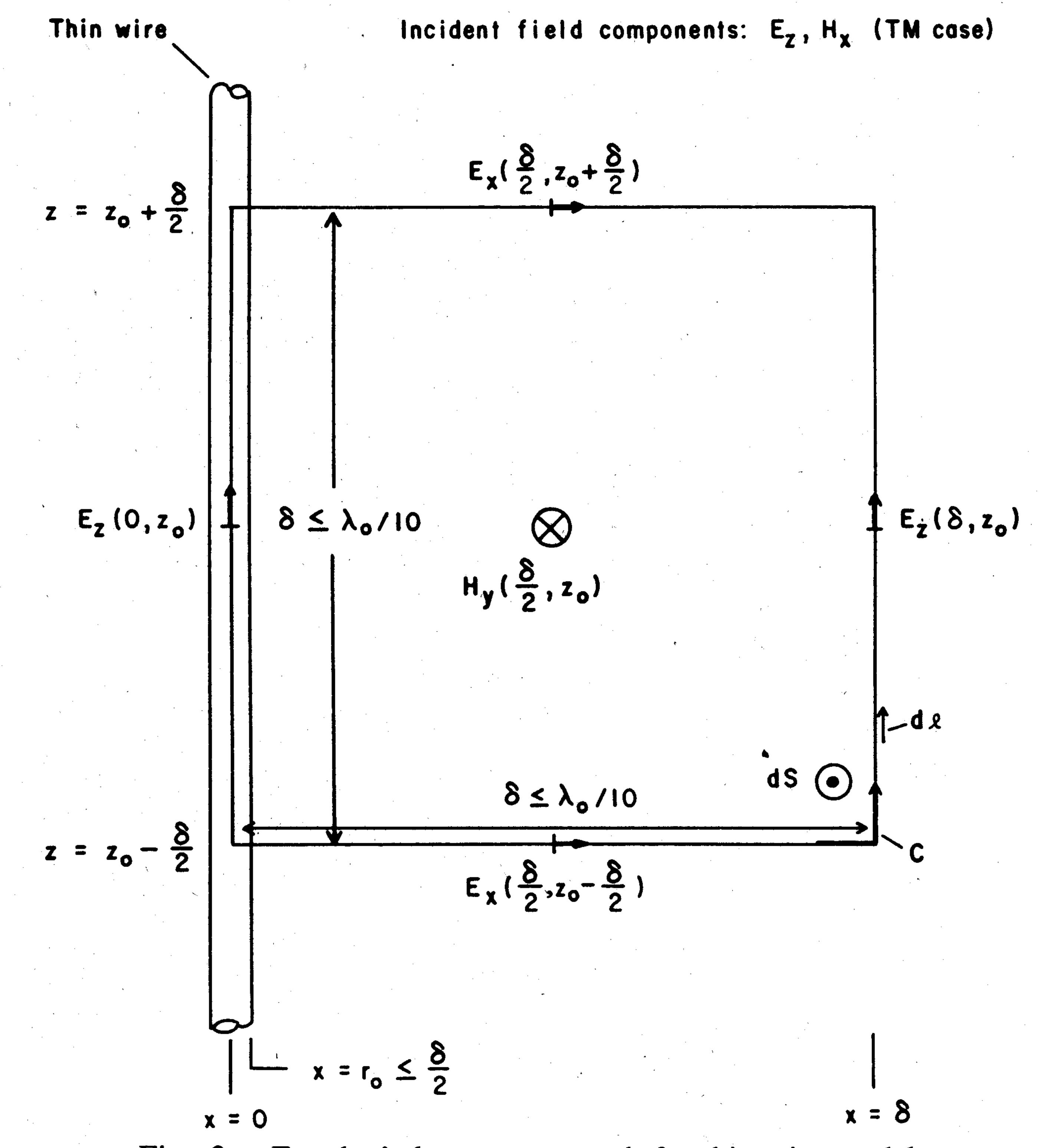
Fig. 2. Faraday's law contour path for thin-wire model.
