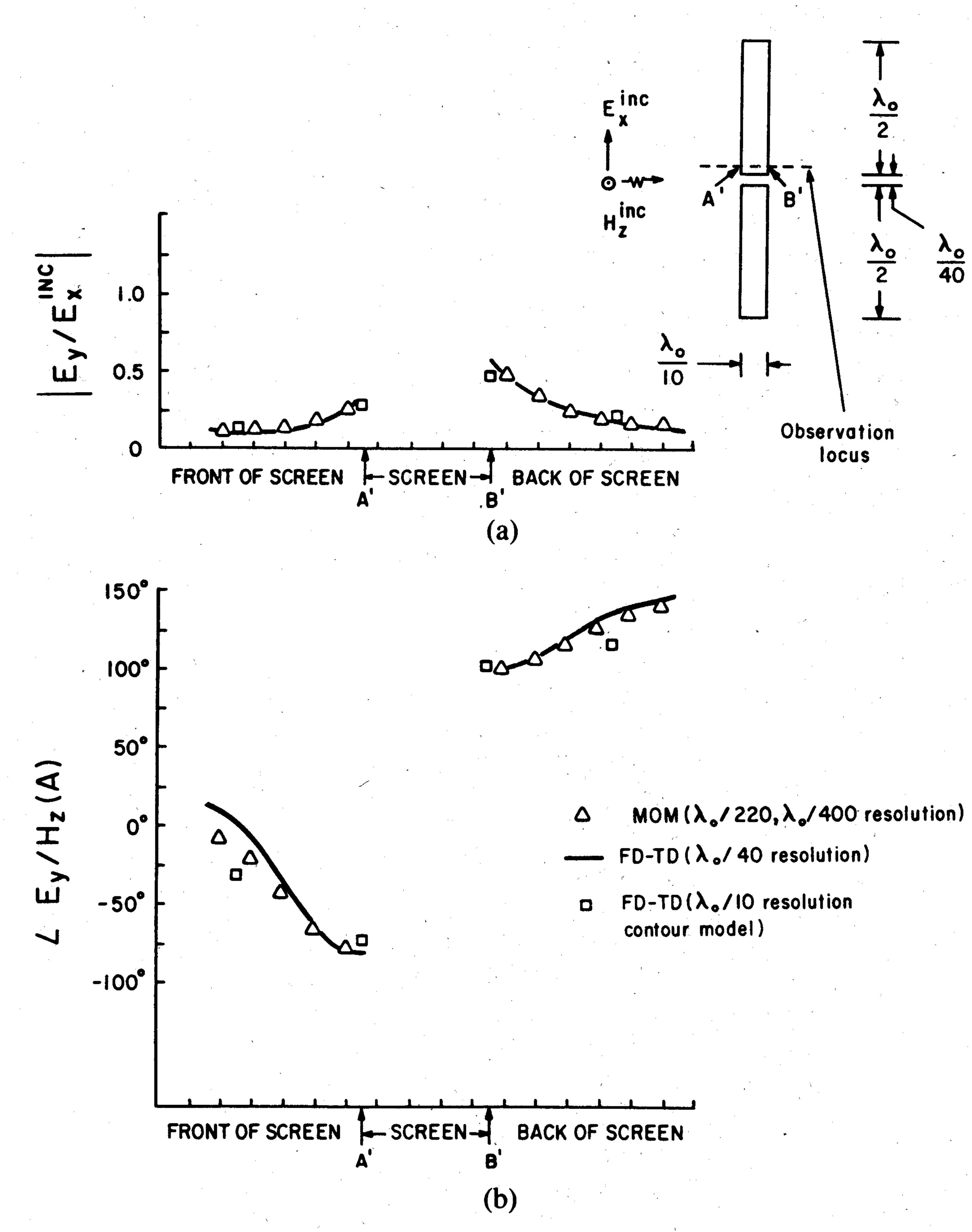
Fig. 8. Comparison of FD-TD and MM solutions for electric field perpendicular to screen, near slot. (a) Magnitude. (b) Phase.
