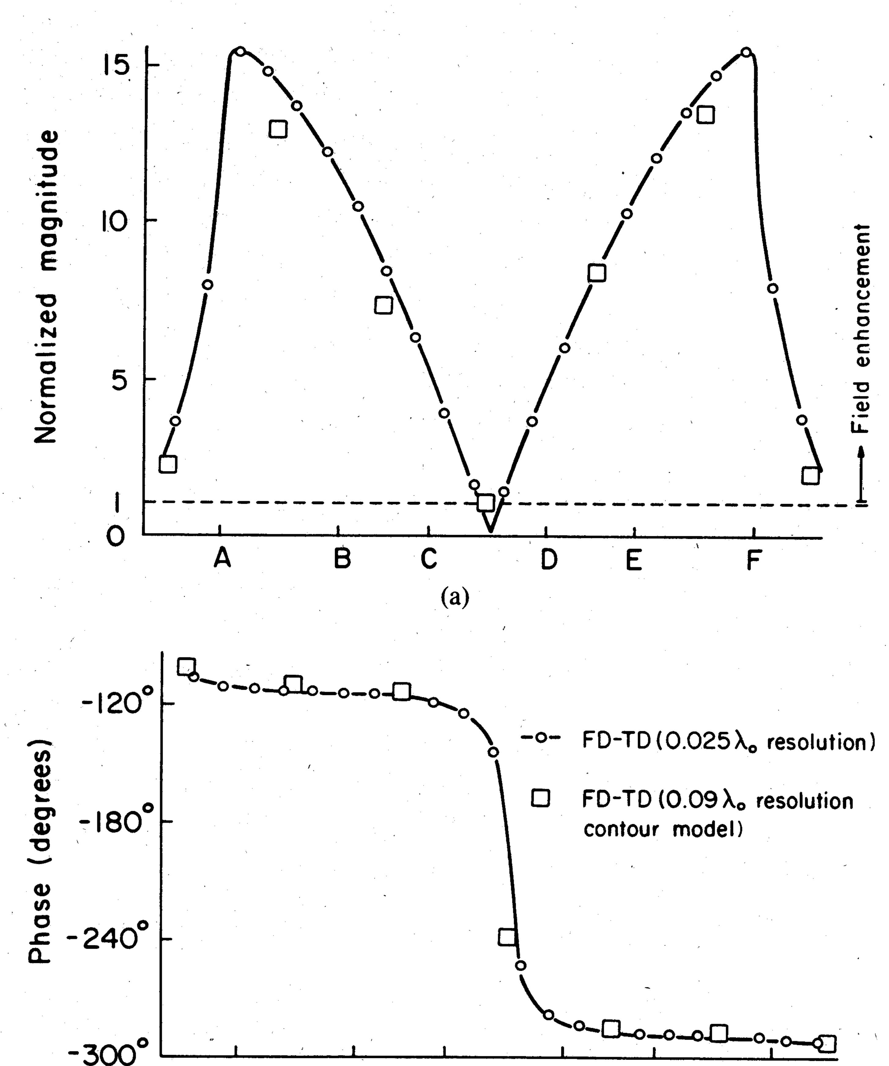
Fig. 12. FD-TD computed electric field within 0.45-wavelength path length, U-shaped lapped joint. (a)  $|E_{\rm gap}/E_{\rm inc}|$ . (b)  $\angle E_{\rm gap}/H_z(A)$ .
