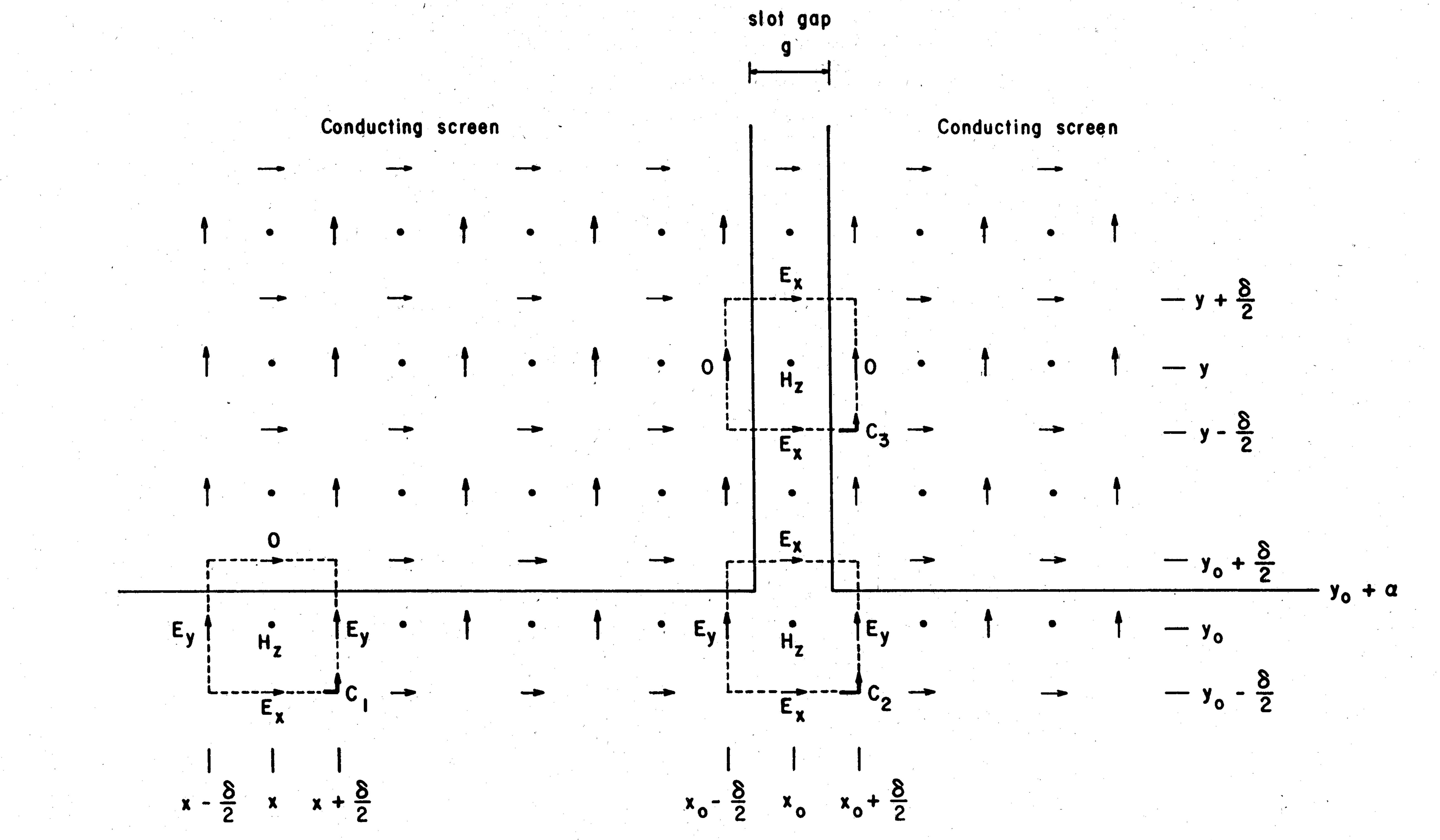
Fig. 5. Faraday's law contour paths for two-dimensional planar conducting screen with thin straight slot (TE case).
