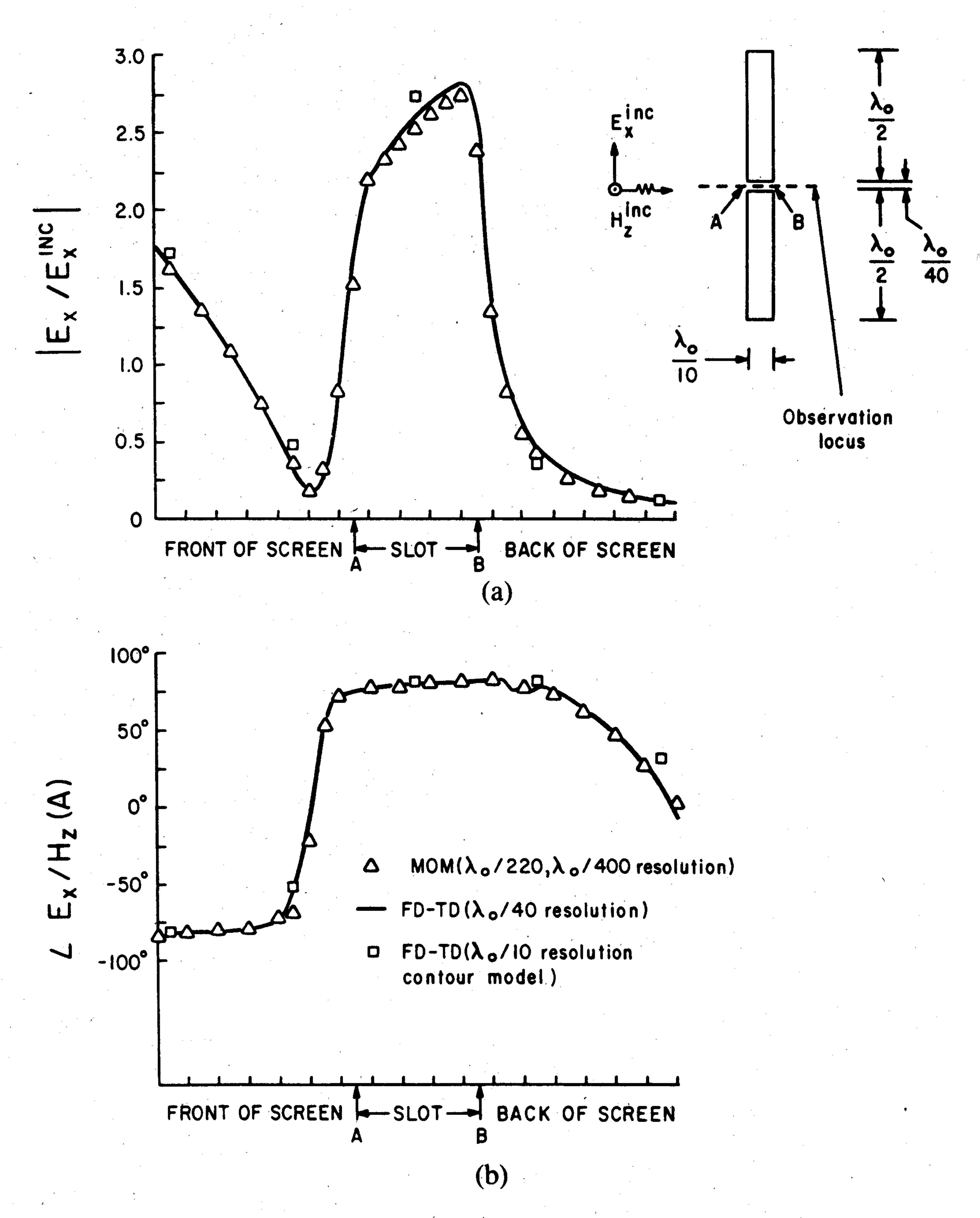
Fig. 6. Comparison of FD-TD and MM solutions for gap electric field distribution, straight-slot case. (a) Magnitude. (b) Phase.
