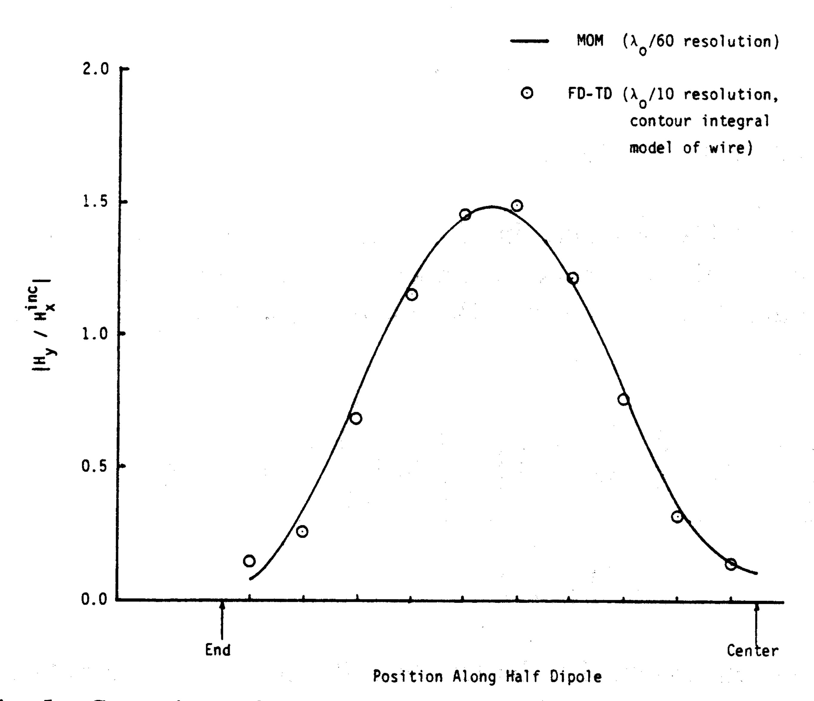
Fig. 5. Comparison of FD-TD and MM solutions for the scattered circumferential magnetic field distribution along a 2.0-Wavelength (Antiresonant) wire of radius 1/300 wavelength (broadside TM-illumination).
