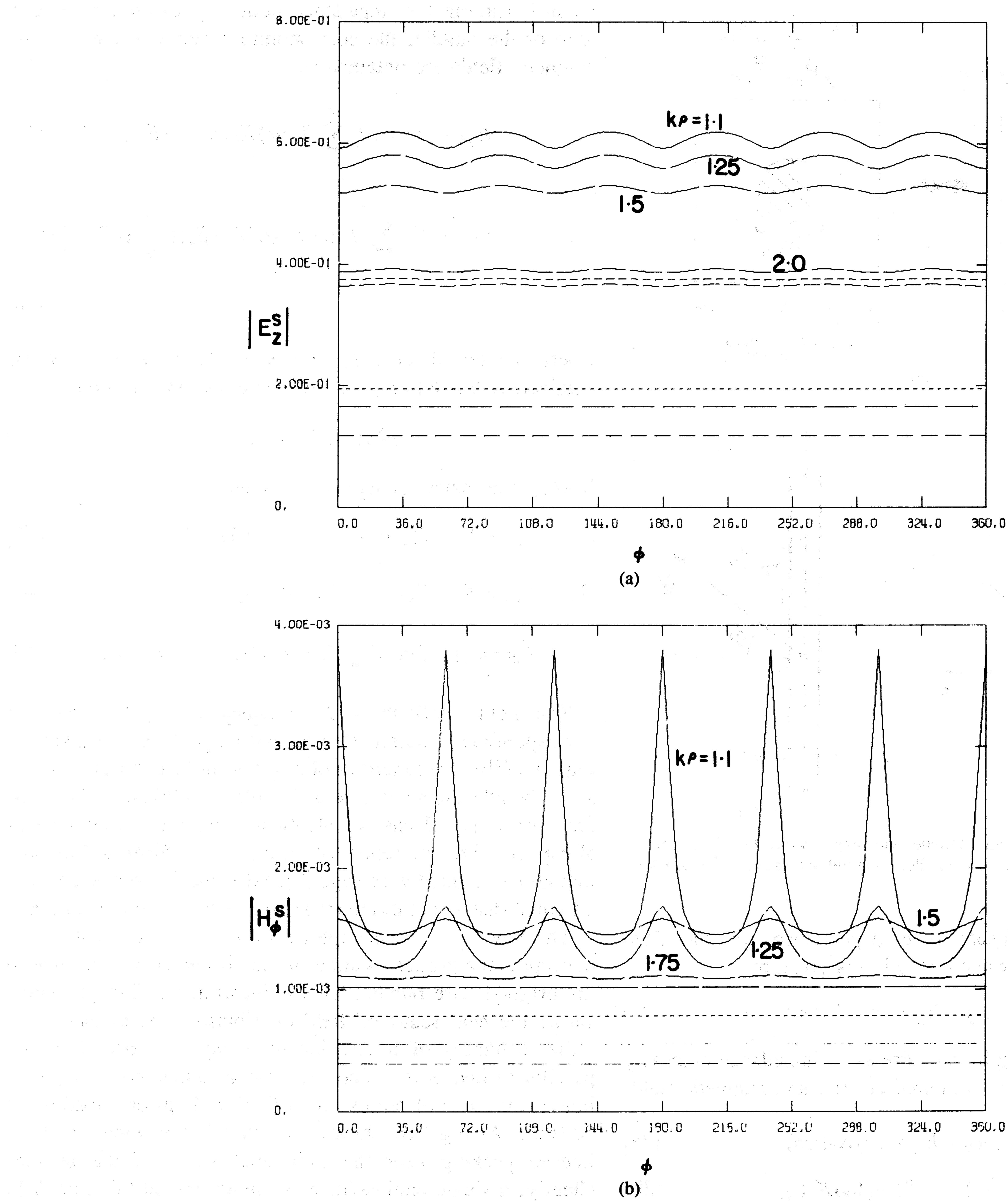
Fig. 2. Near scattered field distributions of circular wire cage versus angle and radial distance. (a)  $|E_z^s|$ . (b)  $|H_{\phi}^s|$ .
