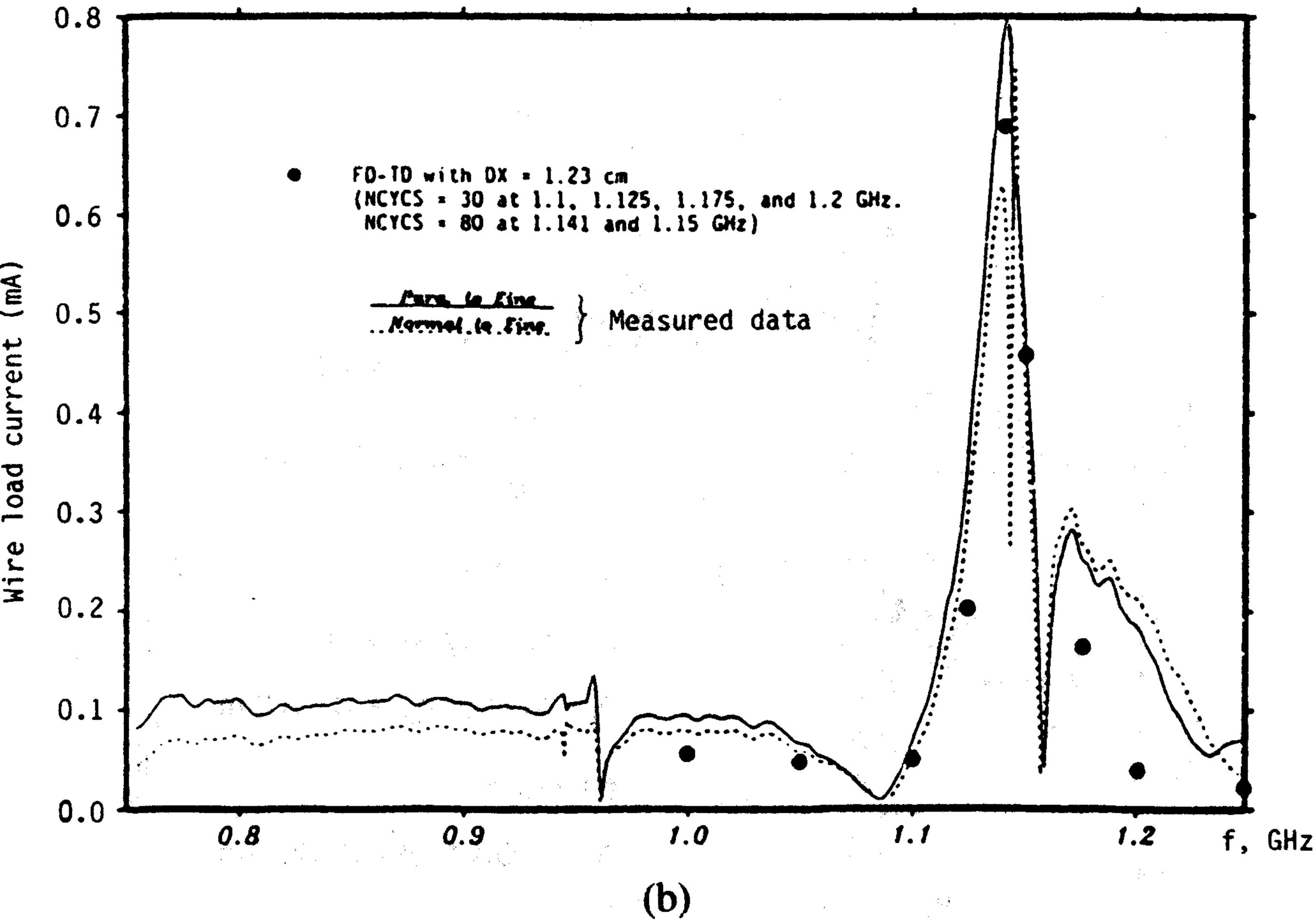
Fig. 9. Experimental validation, PLUTO cavity case. (a) Single wire centered in PLUTO. (b) Wire-pair centered in PLUTO.
