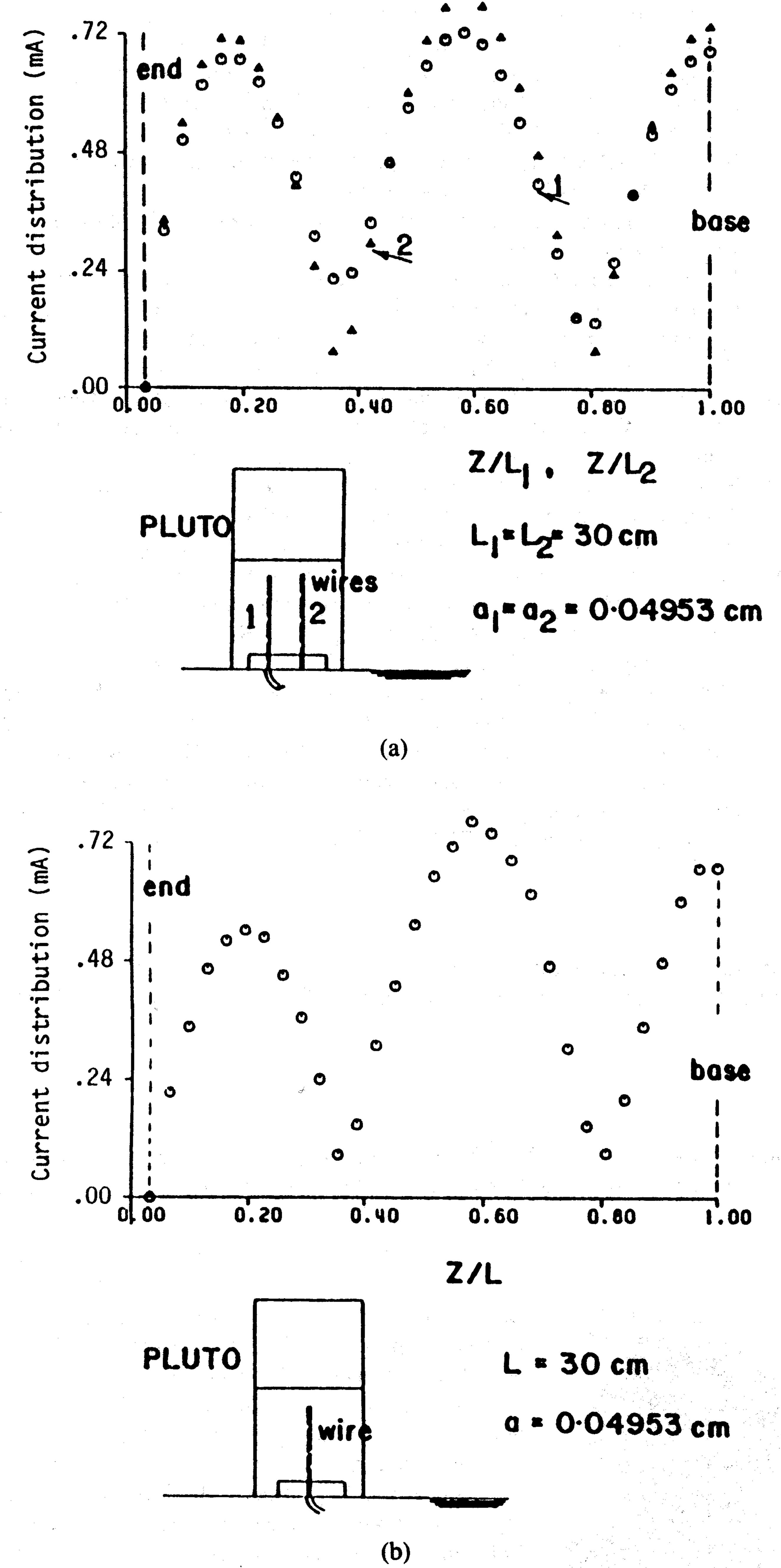
Fig. 10. FD-TD predicted induced current distributions, PLUTO cavity case. (a) Along single wire centered in PLUTO. (b) Along each wire of the wire-pair centered in PLUTO.
