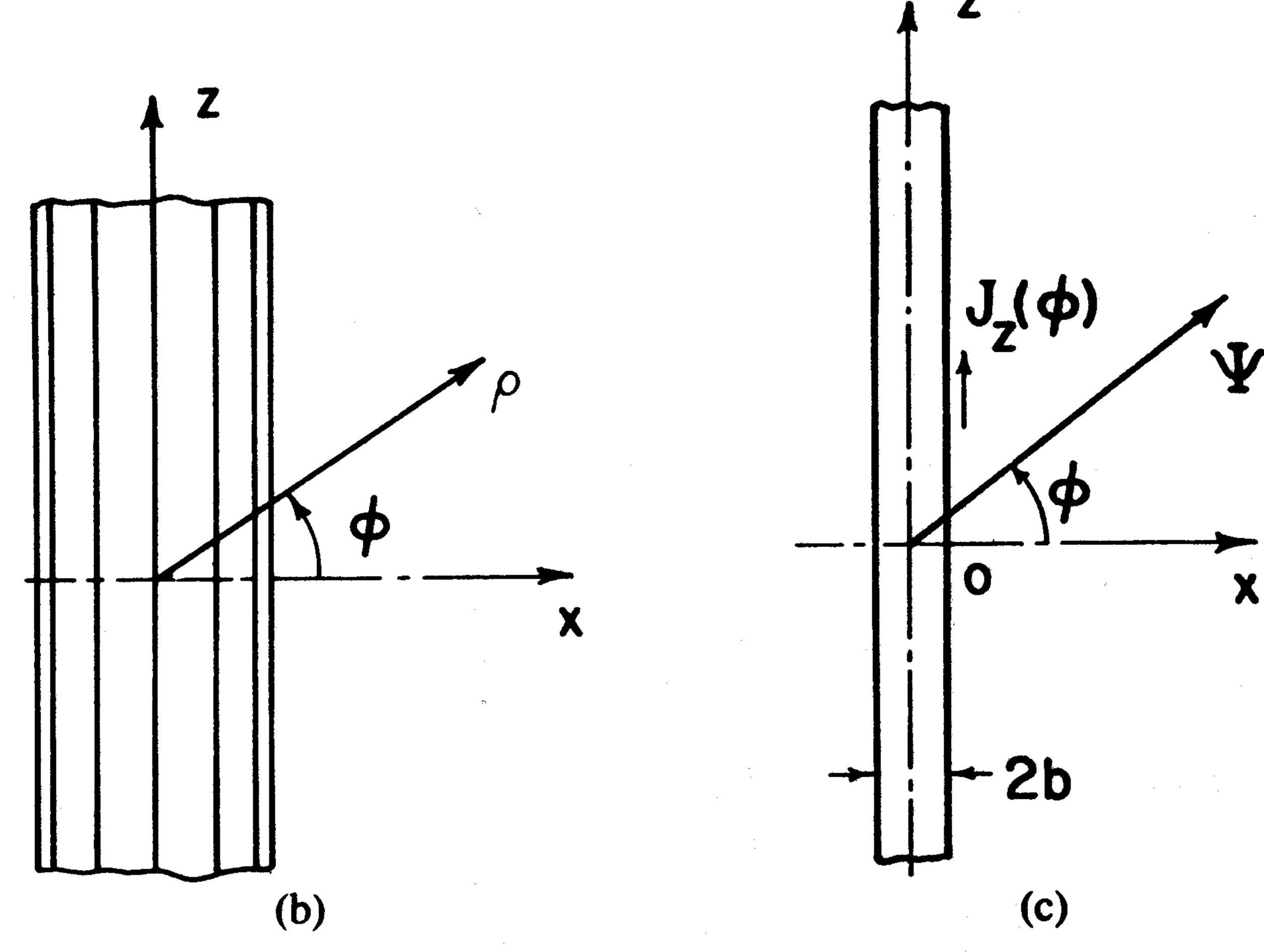
Fig. 1. Equivalence of wire bundle and single wire. (a) Cross-section geometry. (b) Original wire bundle, longitudinal view. (c) Equivalent single wire.
