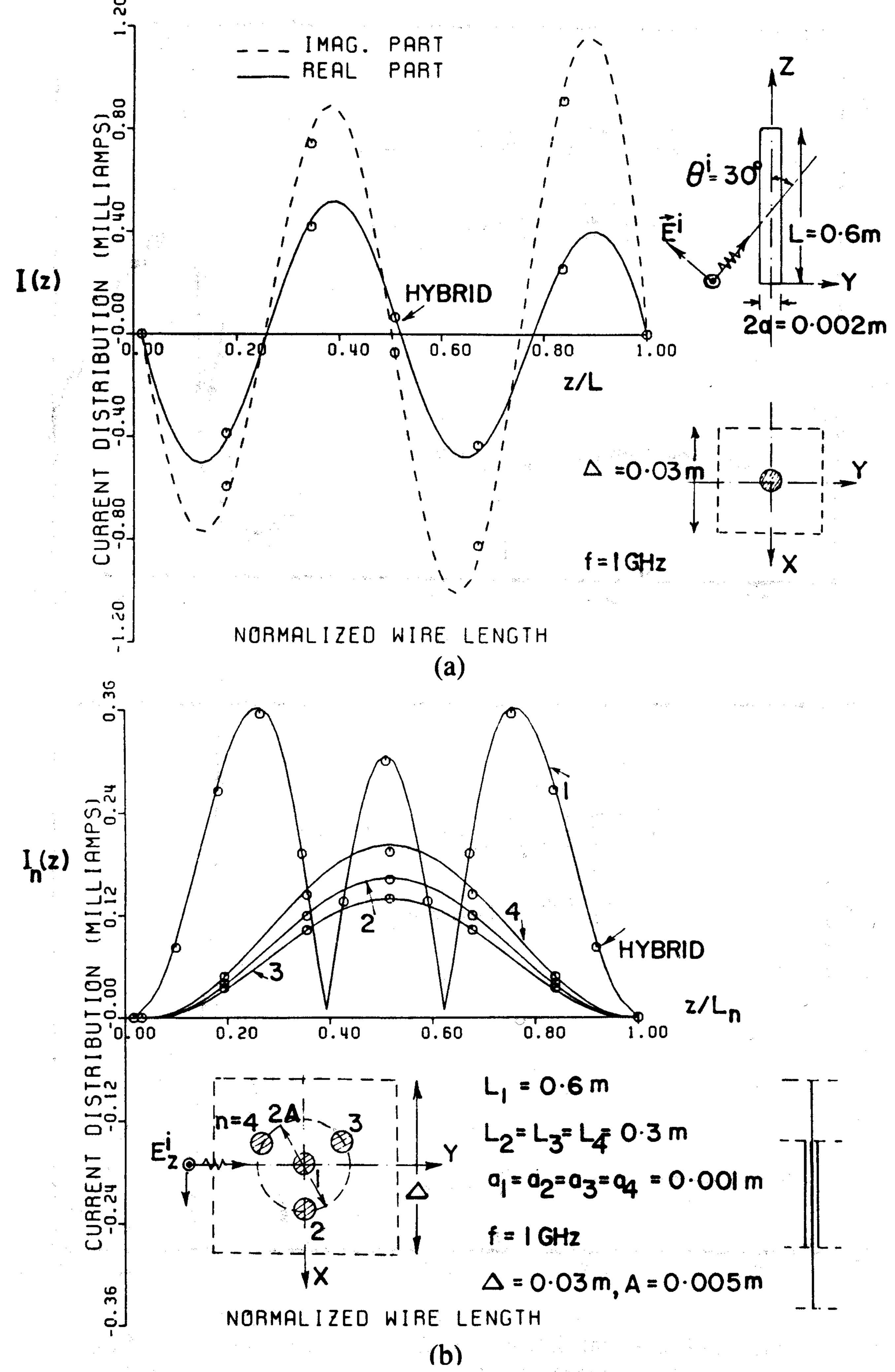
Fig. 7. Sample free-space validations. (a) Single wire. (b) Four-wire bundle, unequal wire lengths.
