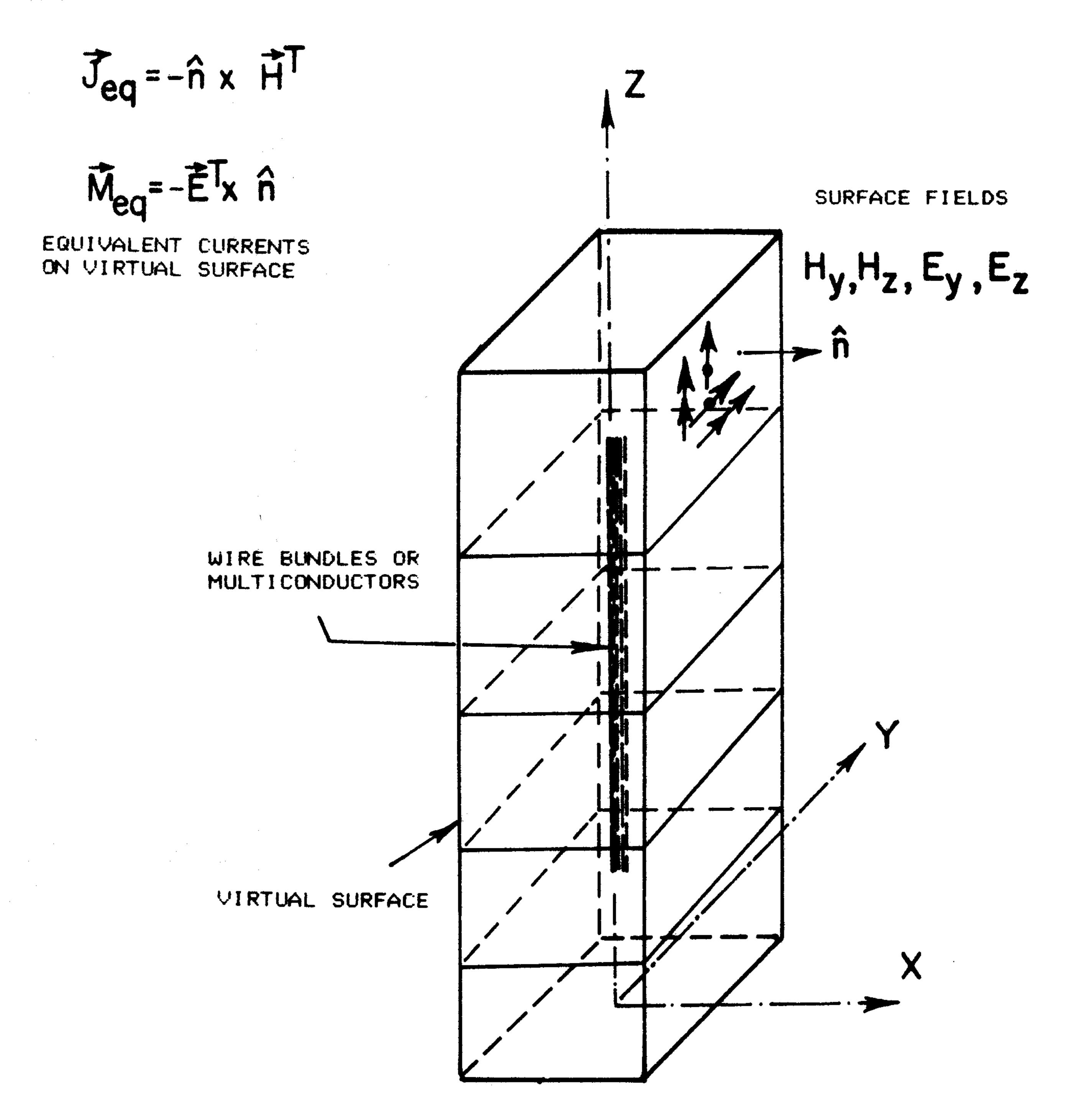
Fig. 6. Wire/wire-bundle within a closed virtual surface.
