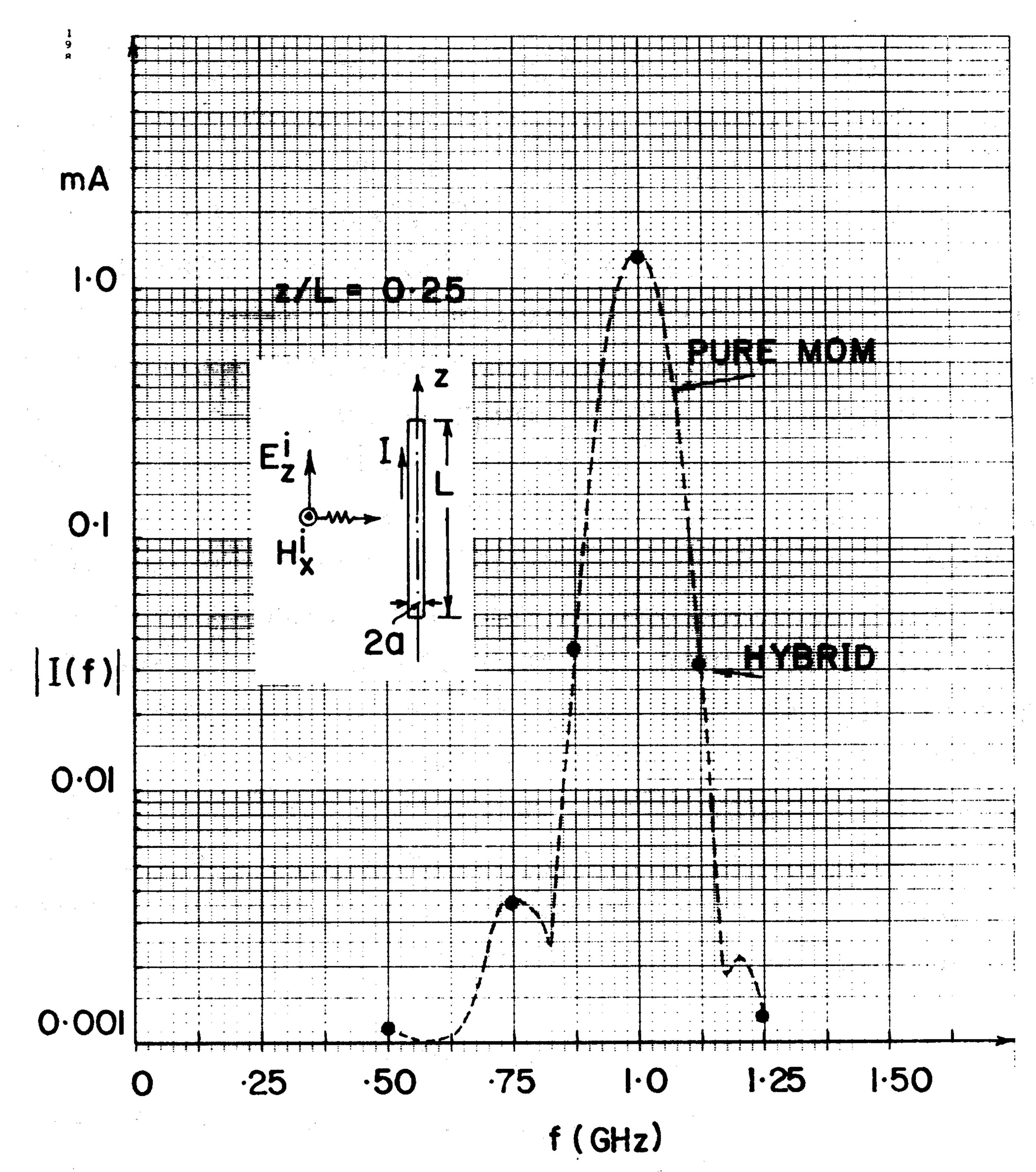
Fig. 11. Validation of predictions of single broad-band FD-TD run for induced wire current versus frequency.
