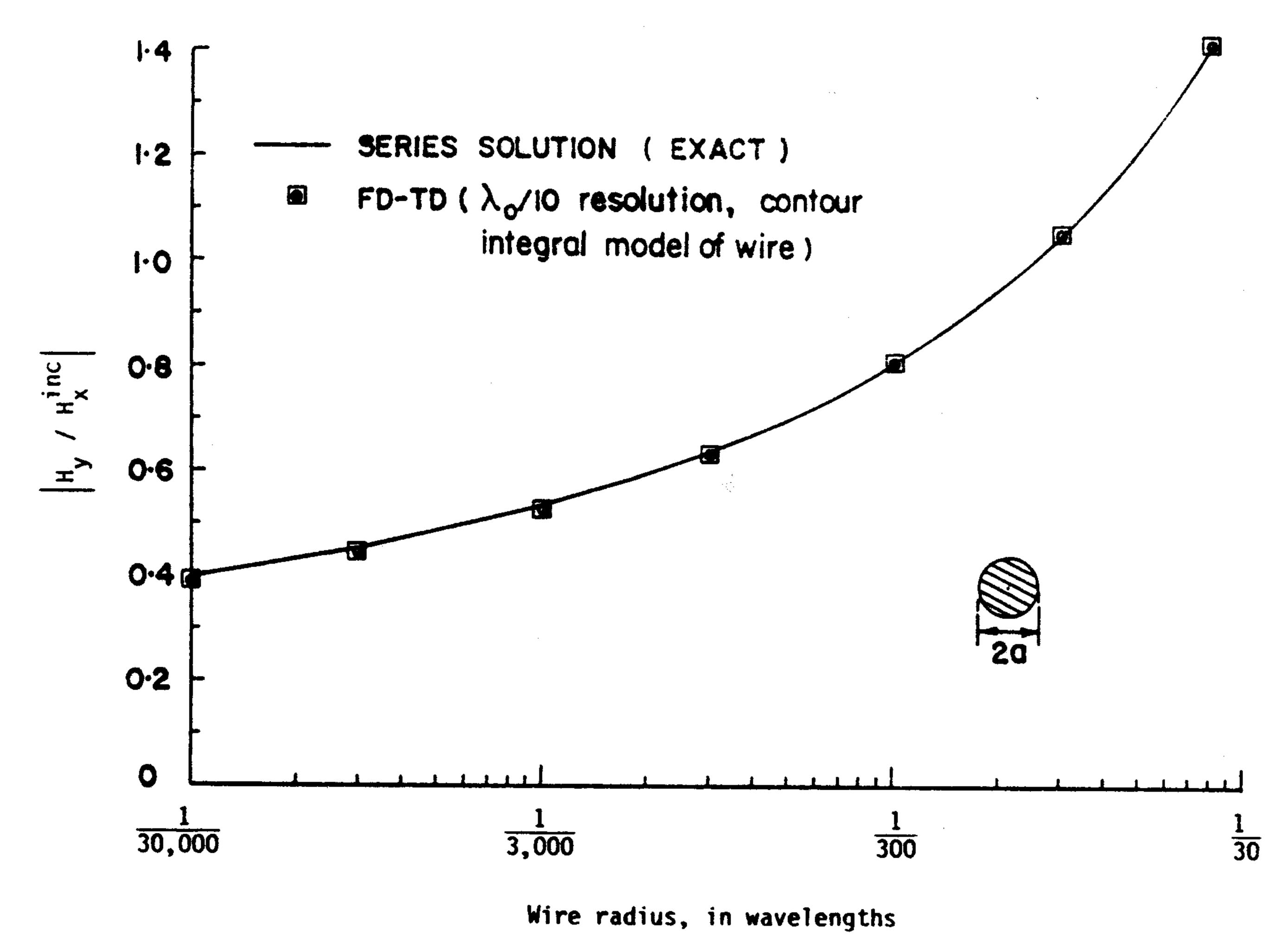
Fig. 4. Comparison of FD-TD and eigenfunction series solution for the scattered circumferential magnetic field at a point 1/20 wavelength from the center of an infinite wire.
