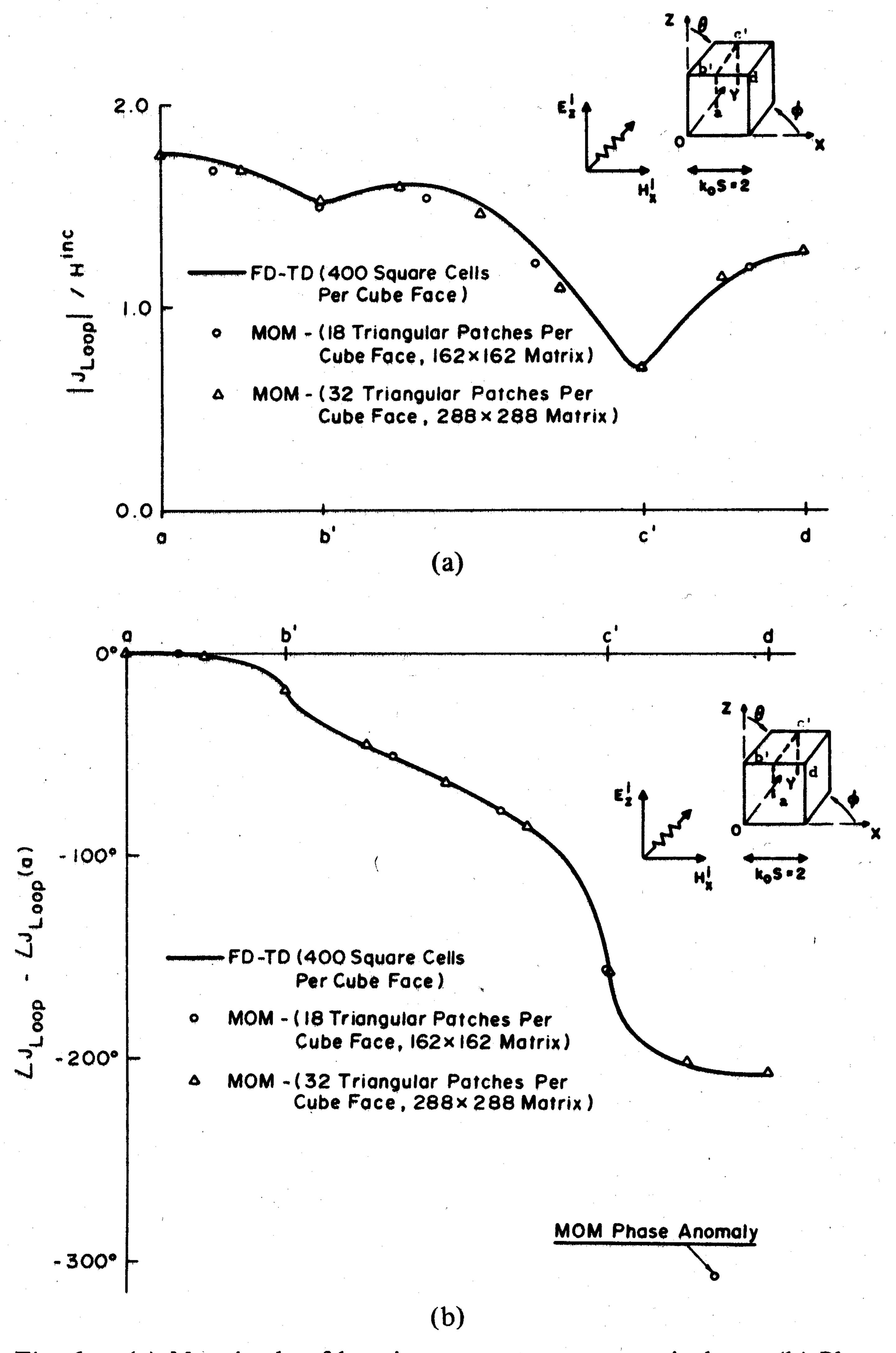
Fig. 6. (a) Magnitude of looping current, center vertical cut. (b) Phase of looping current, center vertical cut.
