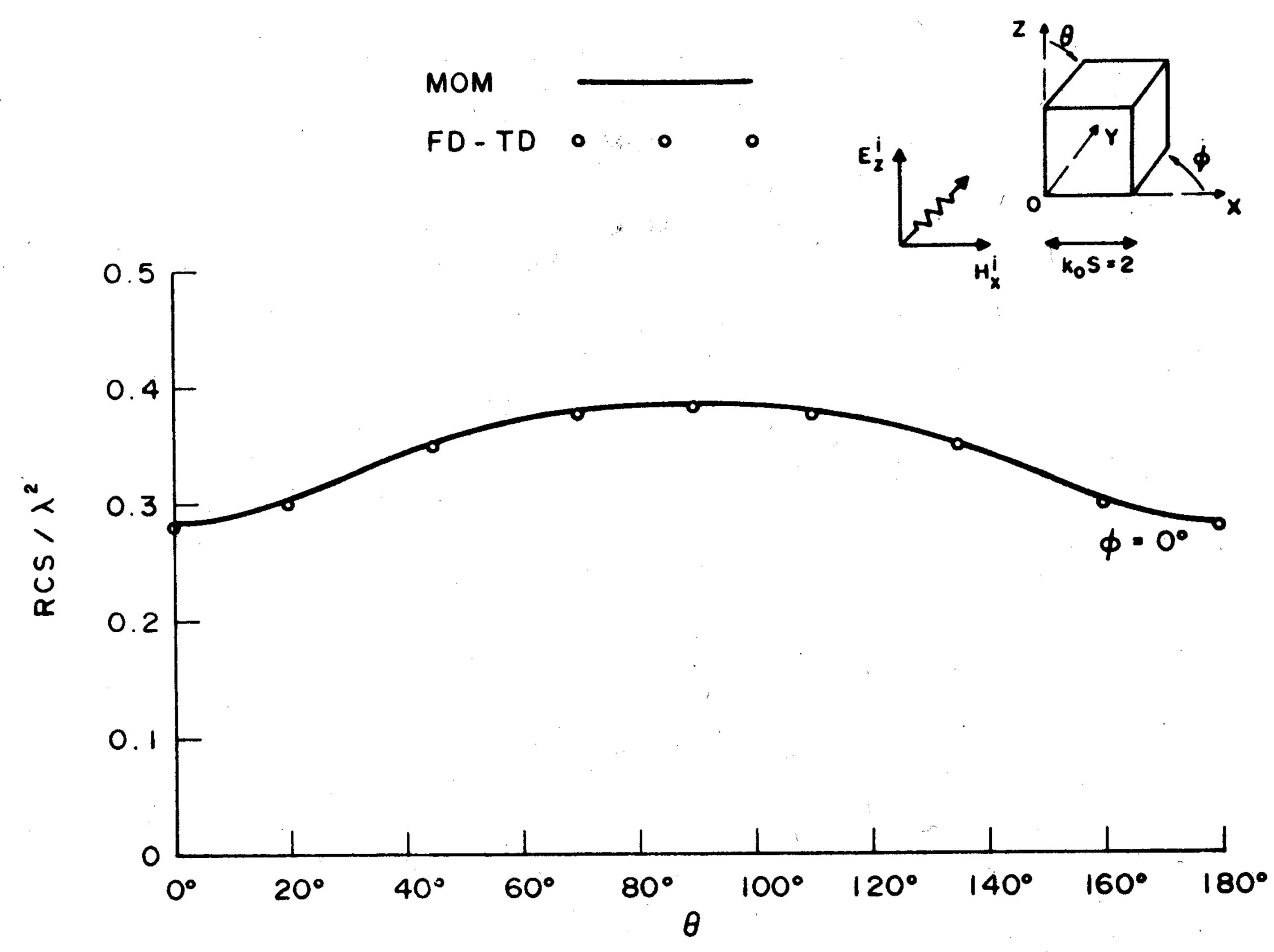
Scattering cross section of the conducting cube scatterer.
