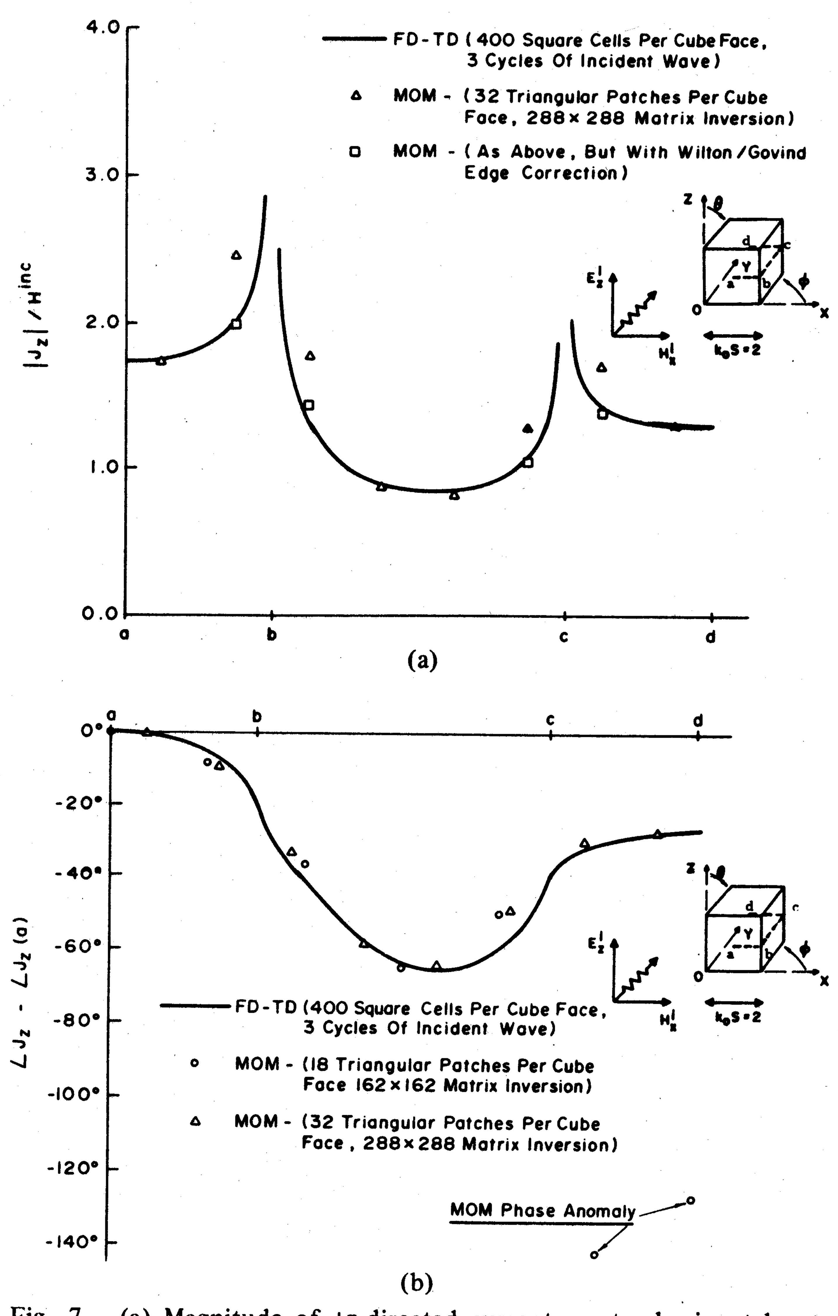
Fig. 7. (a) Magnitude of +z-directed current, center horizontal cut. (b) Phase of +z-directed current, center horizontal cut.
