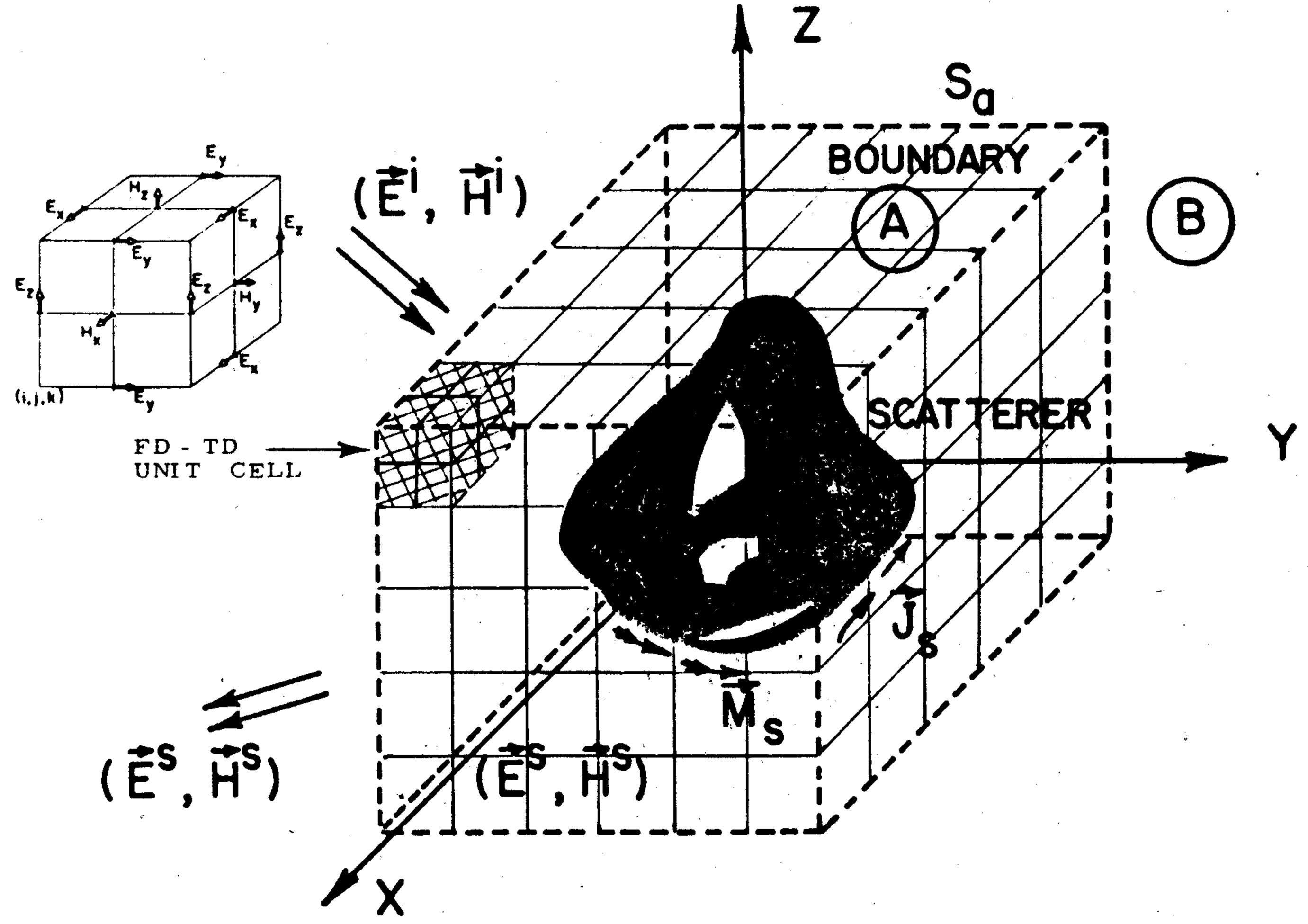
Geometry of a general scatterer in free-space medium and FD-TD lattice arrangement.
