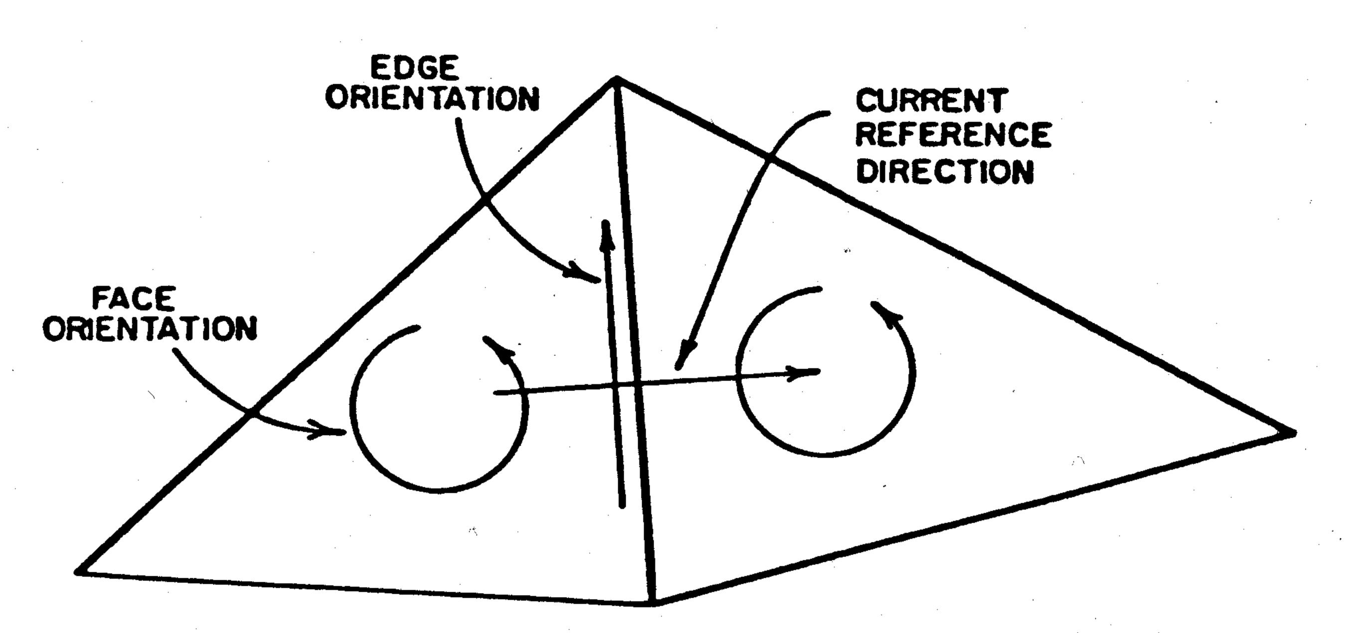
Fig. 4. Scatterer with triangular-patch modeling [18], [19].
