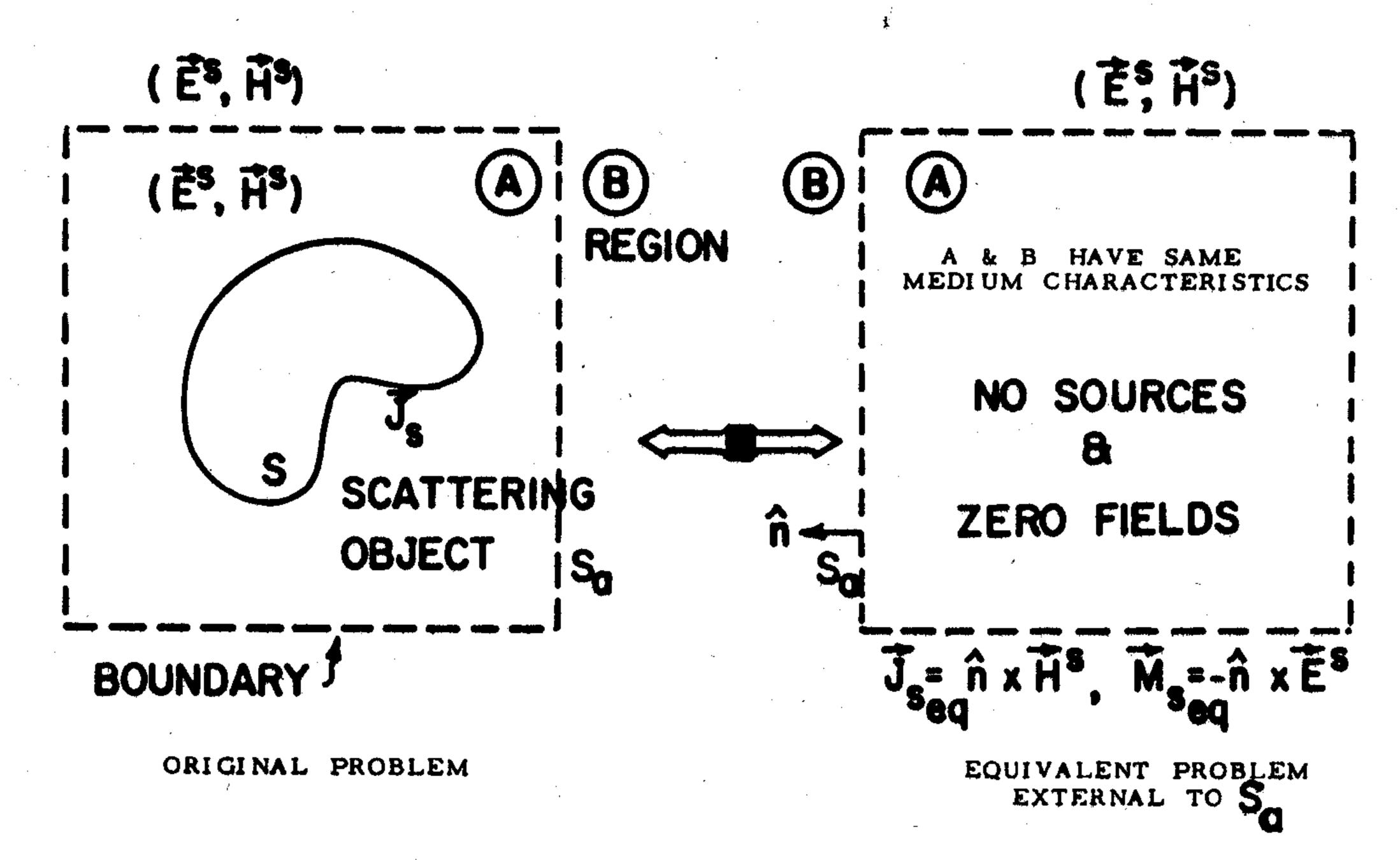
Fig. 3. Electromagnetic equivalence to transform near-fields to farfields.
