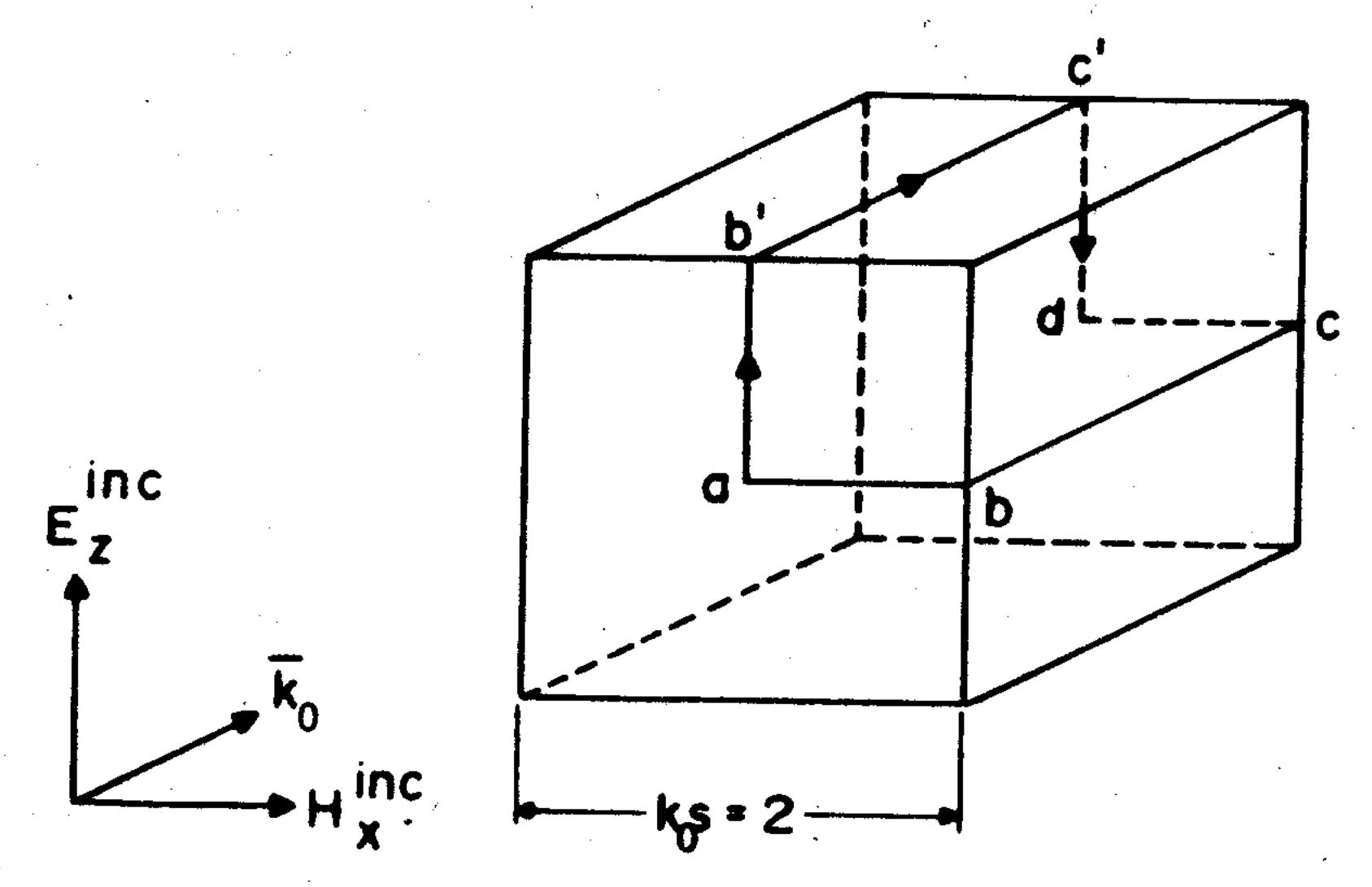
Fig. 5. Geometry of metal-cube scatterer.
