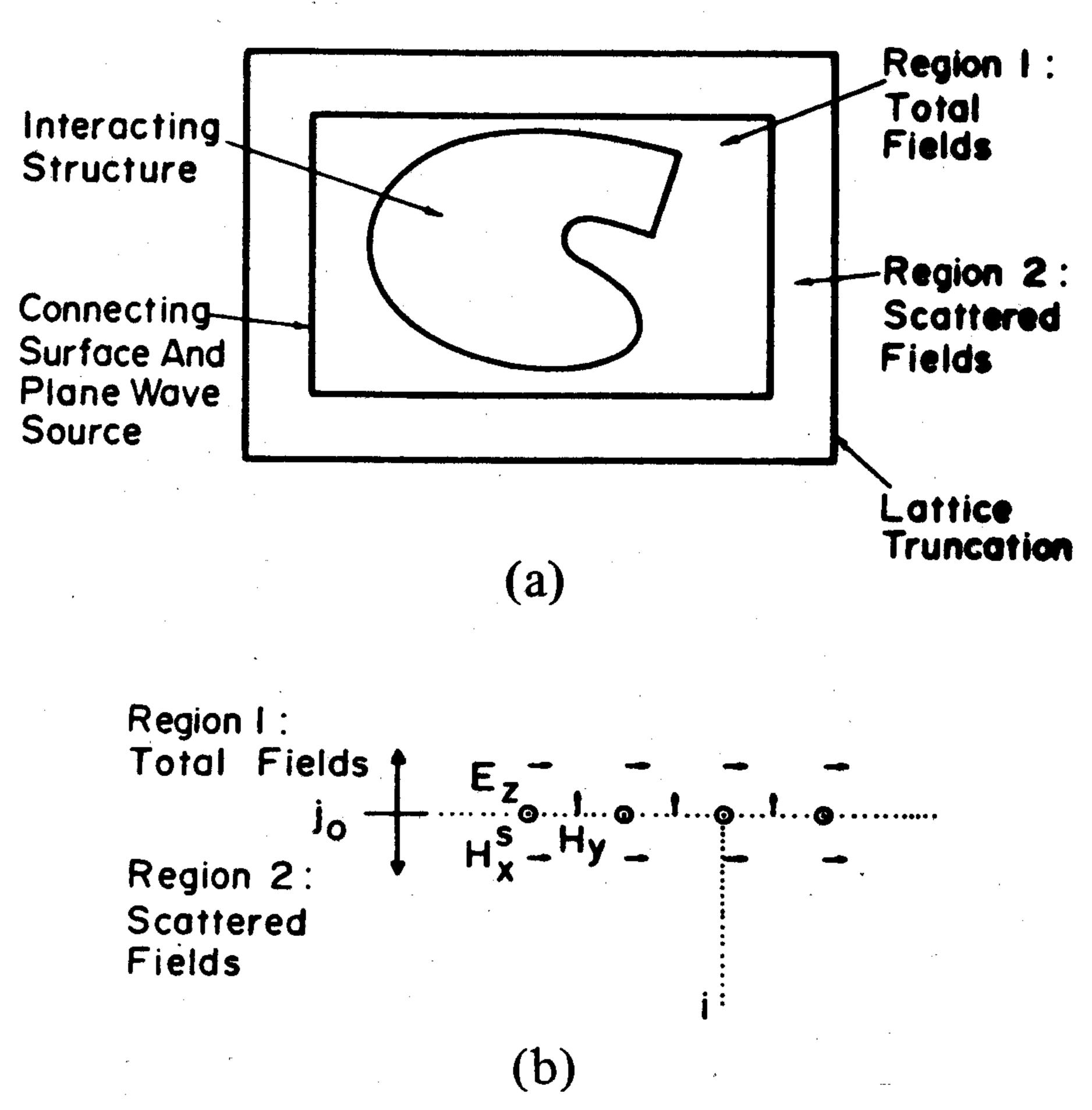
Fig. 2. Division of FD-TD lattice into total-field and scattered-field regions. (a) Lattice division. (b) Typical connecting conditions between regions.
