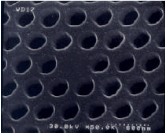
Fabricated device: membrane microresonator in InGaAsP
