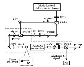
Fig. 3. Experimental setup to demonstrate the pulsedelayed DOPA, using AlGaAs waveguides.
