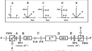
Fig. 2. Novel pulse-delayed DOPA scheme.
