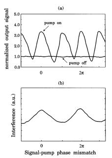
Fig. 4. (a) Normalized output signal for the cases when the pump is on and off:  $I_p = 1.16 \text{ GW/cm}^2$  and  $I_s = 0.35 \text{ GW/cm}^2$ ; (b) interference between pump and signal as a function of the pump-signal phase mismatch.
