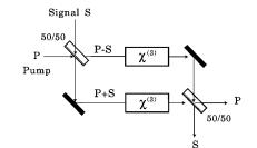
Fig. 1. NMZI scheme for a  $\chi^{(3)}$ -based degenerate OPA.
