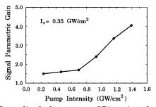
Fig. 5. Normalized degenerate OPA gain of the input signal as a function of pump intensity inside the AlGaAs waveguide.
