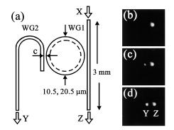
Fig. 1. (a) Illustration of the fabricated ring or disk resonator geometry and (b)-(d) infrared camera images showing switching of light from port Z to port Y at the 1555.6-nm resonance of the 10.5- $\mu$ m-diameter disk.
