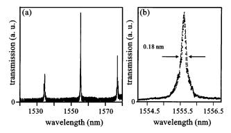
Fig. 4. (a) Measured transmission of the  $10.5-\mu$  mdiameter disk. (b) Fine-resolution spectral scan of the  $10.5-\mu$ m-disk transmitted peak centered at 1555.6 nm and the calculated transmission (dotted curve).
