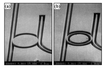
Fig. 2. SEM images of a 10.5- $\mu$ m-diameter (a) disk and (b) ring.
