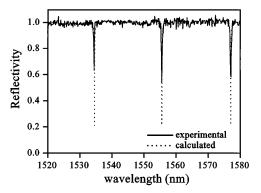
Fig. 3. Measured (experimental) and calculated reflectivity, showing resonances from a 10.5- $\mu$ m disk with 2% coupling and  $\alpha = 1.6$ /cm.
