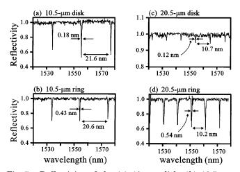
Fig. 5. Reflectivity of the (a) 10- $\mu$ m disk, (b) 10.5- $\mu$ m ring, (c) 20.5- $\mu$ m disk, and (d) 20.5- $\mu$ m ring.  $\Delta \lambda_{\rm FWHM}(\rightarrow \leftarrow)$  and  $\Delta \lambda_{\rm fsr}(\leftrightarrow)$  are indicated in the graphs.
