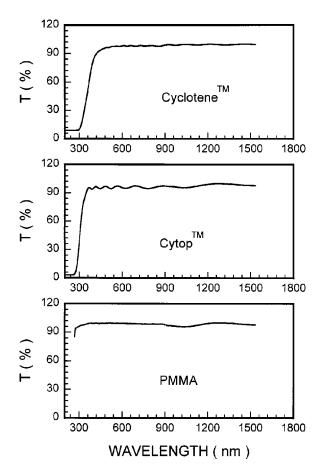
FIG. 2. Room-temperature transmission spectra of the waveguide polymer components, Cyclotene<sup>TM</sup>, Cytop<sup>TM</sup>, and PMMA.
