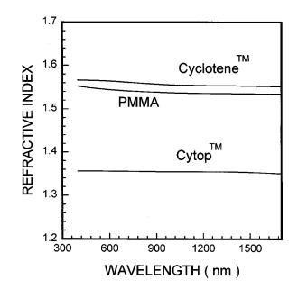
FIG. 3. Wavelength dependence of the refractive indices of Cyclotene<sup>TM</sup>, PMMA, and Cytop<sup>TM</sup>.
