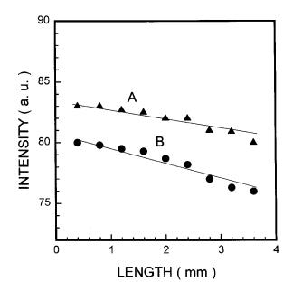
FIG. 4. Measured image intensity as a function of waveguide length for different waveguide structures A: Cytop<sup>TM</sup>/Cyclotene<sup>TM</sup>/Cytop<sup>TM</sup>, and B: Cytop<sup>TM</sup>/PMMA/Cytop<sup>TM</sup>.
