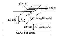
FIG. 1. AlGaAs Bragg filter waveguide structure.
