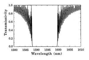
FIG. 5. Theoretically calculated transmissivity spectrum for a Bragg filter. The refractive indices used in the EIM calculations at  $\lambda = 1.6 \ \mu$ m for the top, guiding, and cladding layers were  $n_i = 1.0$ ,  $n_g = 3.26214$ , and  $n_c = 3.08689$ , respectively.
