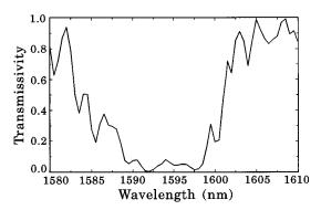
FIG. 4. Experimentally measured transmissivity spectrum of the AlGaAs Bragg filter with a FWHM bandwidth of about 15 nm.
