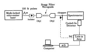
FIG. 3. Experimental setup to measure the bandwidth of the Bragg filter.
